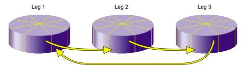
Figure 2-3 Reading Data from a Mirror with a Round-Robin Read Policy
