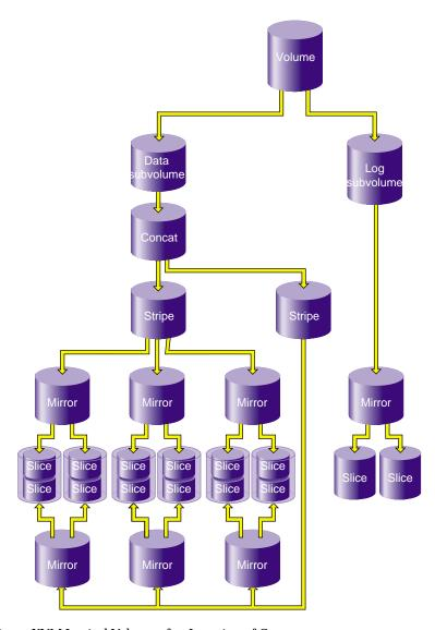
Figure 1-9 XVM Logical Volume after Insertion of Concat
