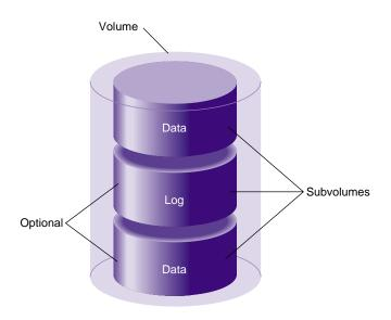
Figure 1-10 shows an XVM volume with system-defined subvolume types.
