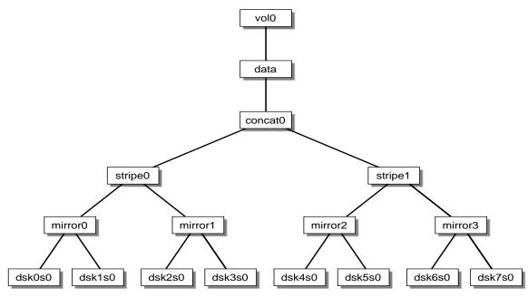
Figure 3-1 XVM Logical Volume with System-Generated Names
