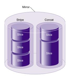
Figure 1-19 shows a mirror composed of a stripe and a concat.
