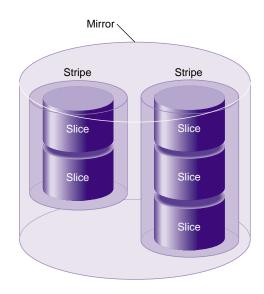
**Figure 1-18** Mirror Composed of Two Stripes
