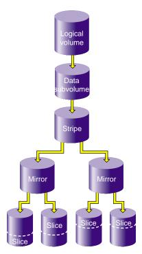
Figure 6-16 XVM Logical Volume after Mirroring Slices
