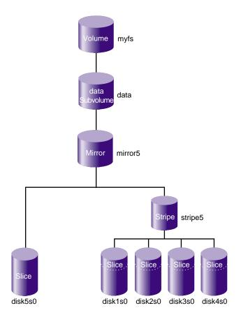
Figure 7-8 Filesystem after Attaching Stripe to Mirror
