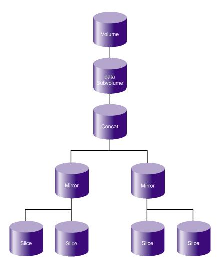
Figure 2-8 Concat Composed of Two Mirrors
