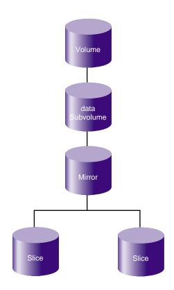
Figure 2-5 Mirror Composed of Two Slices
