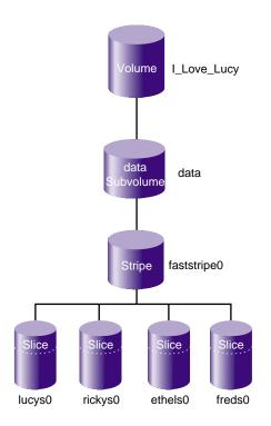
Figure 7-2 Striping a Portion of a Disk
