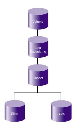
Figure 2-3 Concat Composed of Two Slices
