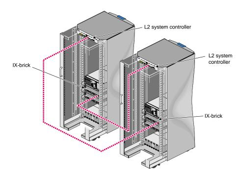
Figure F-5 Serial Connection Between Two SGI Origin 3400 or SGI Origin 3800 Servers
