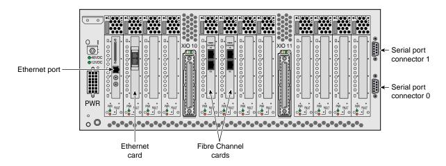
Figure F-2 IX-brick Rear Panel
