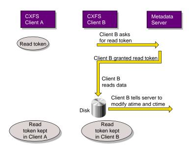
Figure A-10 Metadata Flow on a Read on Client B Following a Read on Client A
