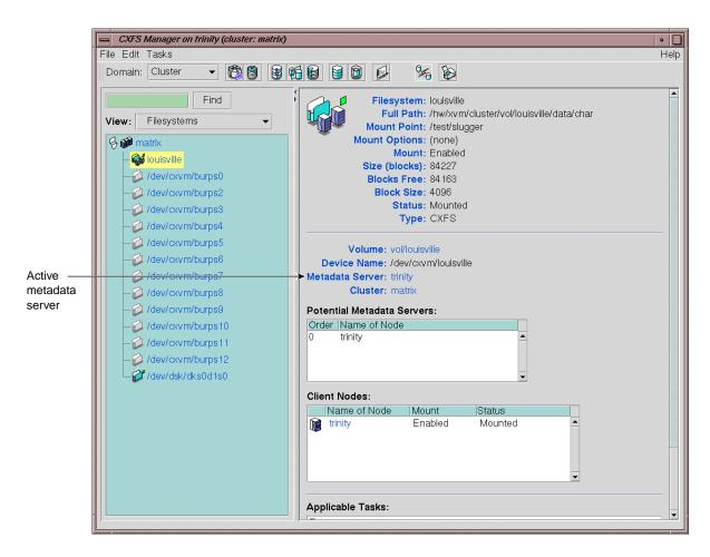
Figure 10-1 Window Showing the Metadata Server
