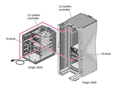
Figure F-4 Serial Connection Between SGI Origin 3200 and Origin 3400/3800 Servers
