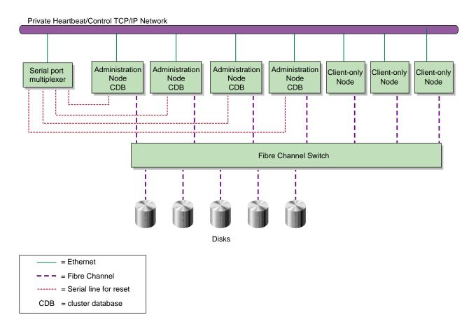
Figure 1-9 Example of a Cluster using Reset
