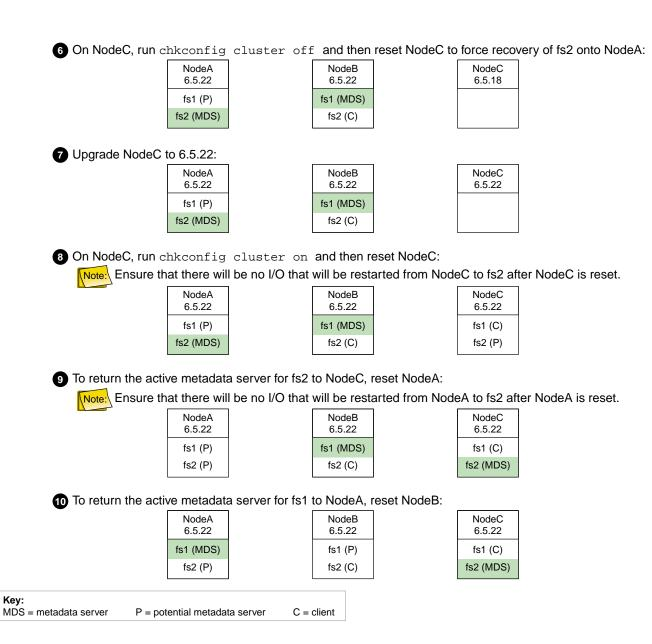
Figure 6-2 Example Rolling Upgrade Procedure (steps 6-10)
