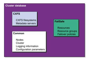
Figure 1-10 Contents of a Coexecution Cluster Database
