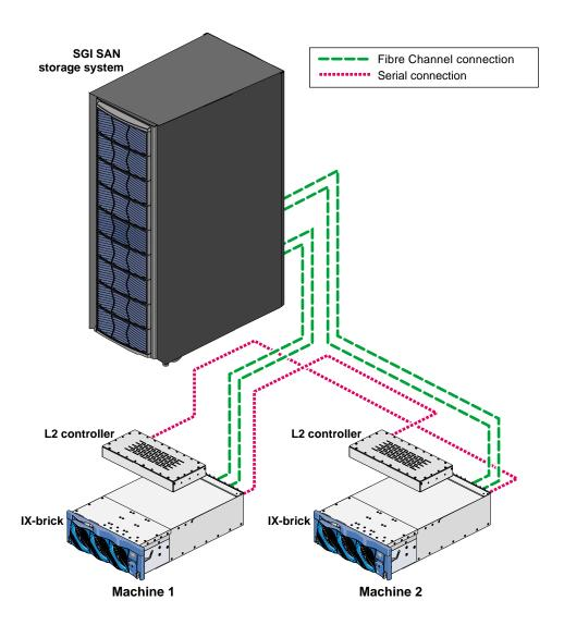
Figure F-3 Altix 3000 and Origin 3000 Serial Connections
