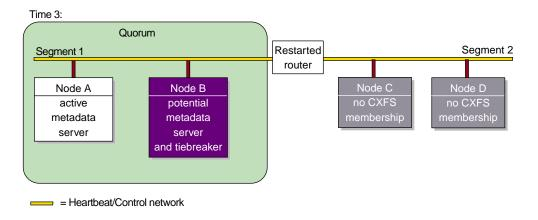
Figure B-6 CXFS Tiebreaker Node
