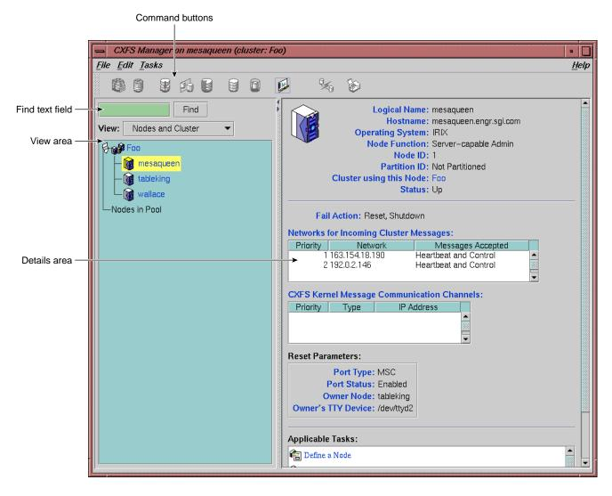
Figure 8-1 CXFS Manager GUI Showing Details for a Node
