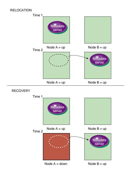
Figure 1-7 Relocation versus Recovery
