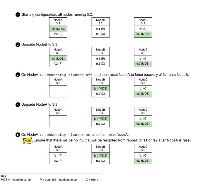
Figure 6-1 Example Rolling Upgrade Procedure (steps 1-5)
