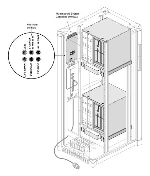
Figure F-10 MMSC Serial Port
