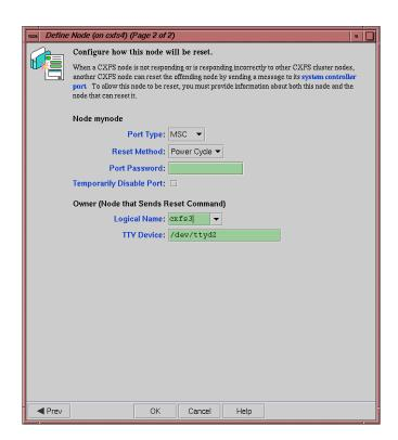
Figure 9-4 Example System Reset Settings
