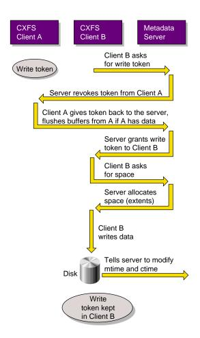
Figure A-8 Metadata Flow on a Write
