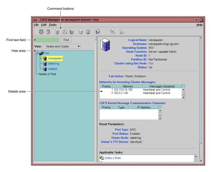
Figure 9-1 CXFS Manager GUI Showing Details for a Node
