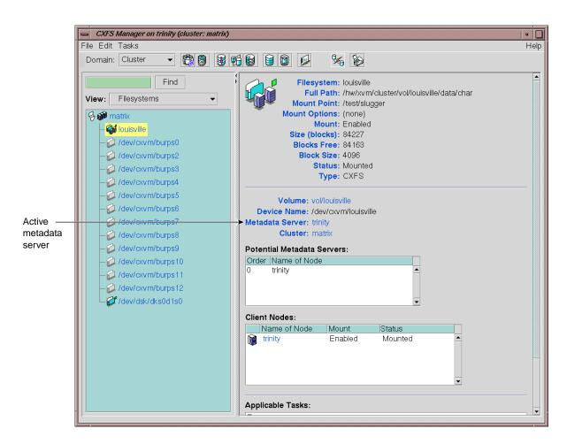
Figure 11-1 Window Showing the Metadata Server
