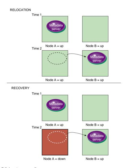
Figure 1-7 Relocation versus Recovery
