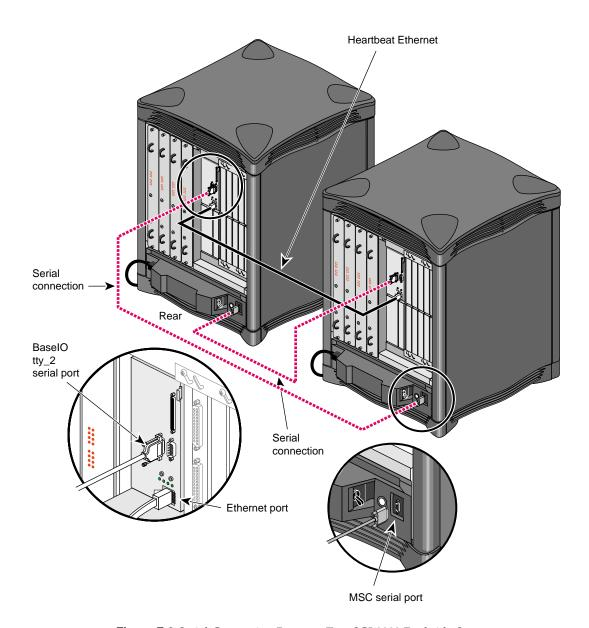
Figure F-9 Serial Connection Between Two SGI 2200 Deskside Servers
