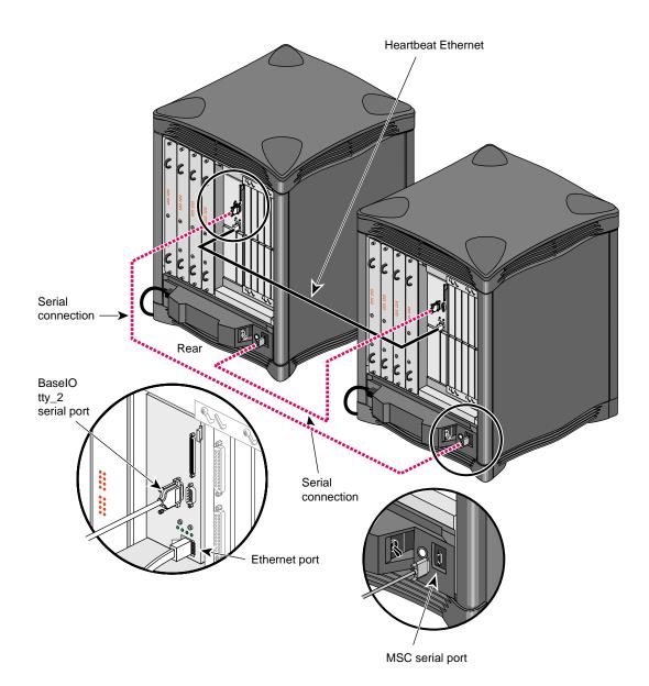
Figure F-10 Serial Connection Between Two SGI 2200 Deskside Servers
