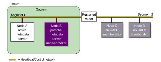
Figure B-6 CXFS Tiebreaker Node
