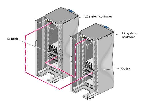
Figure F-7 Serial Connection Between Two SGI Origin 3400 or SGI Origin 3800 Servers
