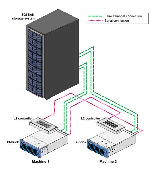
Figure F-5 Altix 3000 and Origin 3000 Serial Connections
