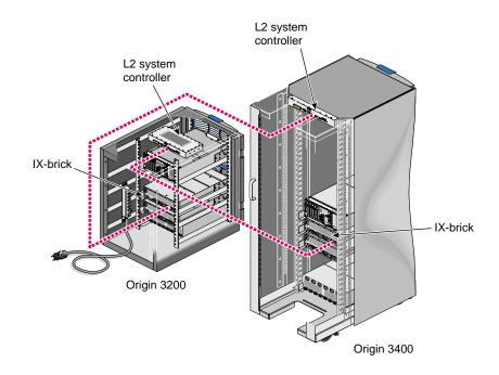
Figure F-6 Serial Connection Between SGI Origin 3200 and Origin 3400/3800 Servers
