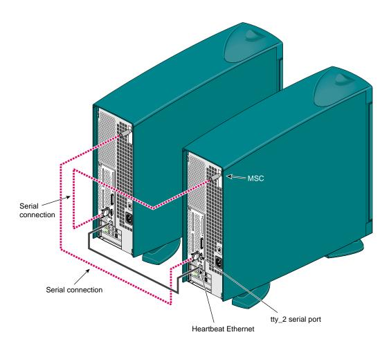
Figure F-9 Serial Connection Between Two Origin 200 Deskside Servers
