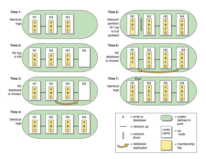
Figure B-1 One Node is Out of Date: Most Recent Log is Replicated
