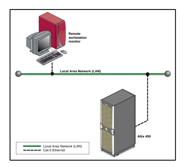
Figure F-1 SGI Altix 450 System Control Network
