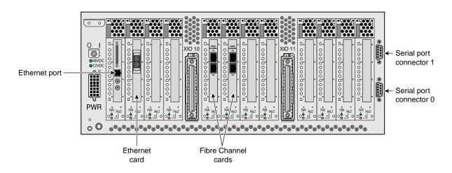
Figure F-4 IX-brick Rear Panel
