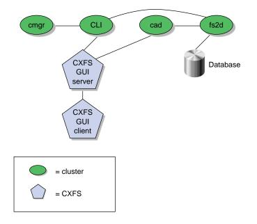
Figure A-4 Communication for an Administration Node Not in a Cluster
