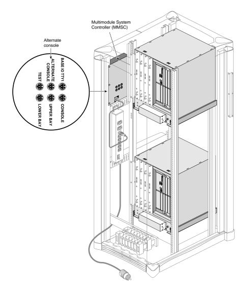
Figure F-11 MMSC Serial Port
