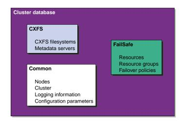
Figure 1-9 Contents of a Coexecution Cluster Database
