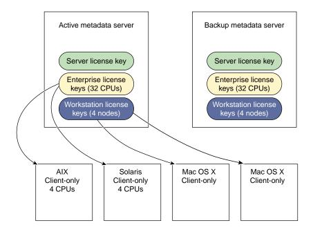
Figure 4-2 Server-Side License Keys: Adding a New Client-Only Node
