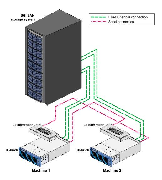
Figure E-5 Altix 3000 and Origin 3000 Serial Connections
