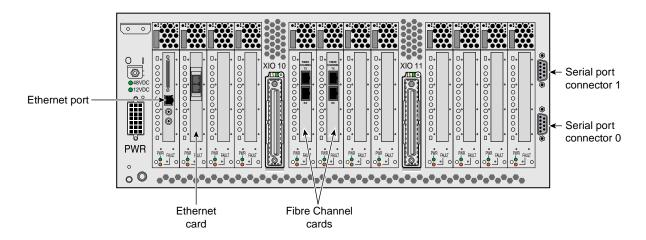
Figure E-4 IX-brick Rear Panel
