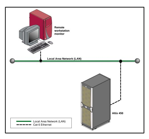
Figure E-1 SGI Altix 450 System Control Network
