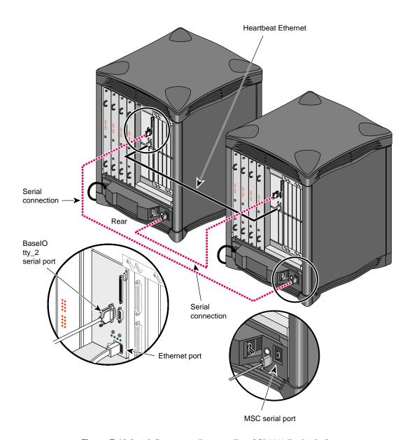
Figure E-10 Serial Connection Between Two SGI 2200 Deskside Servers
