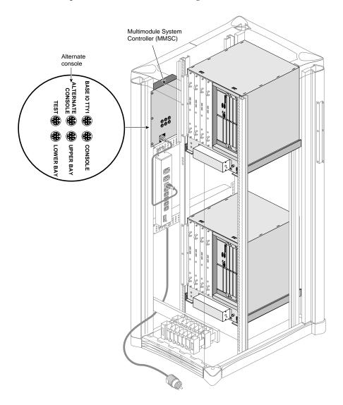
Figure E-11 MMSC Serial Port
