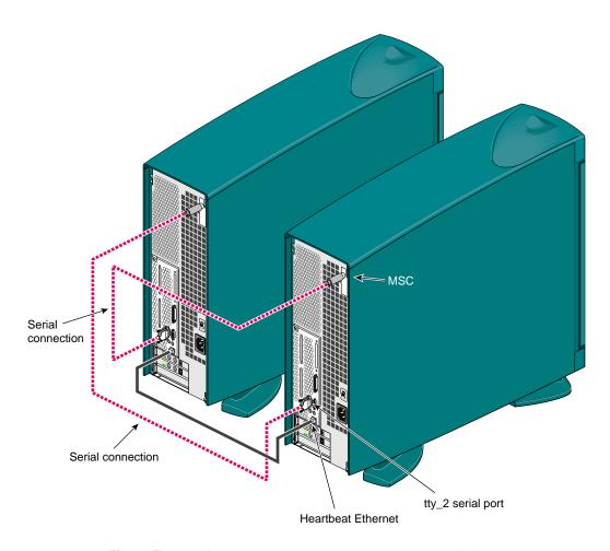
Figure E-9 Serial Connection Between Two Origin 200 Deskside Servers
