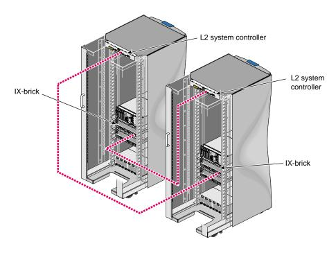
**Figure E-7** Serial Connection Between Two SGI Origin 3400 or SGI Origin 3800 Servers
