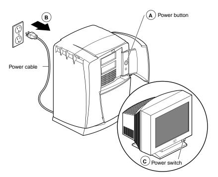
Figure 2-1 Powering Off the Octane2 Workstation
