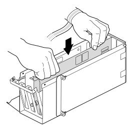
**Figure 4-23** Inserting a PCI Board with an Extra-long Connector
