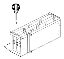
Figure 4-17 Inserting the Board Screw
