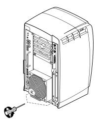
**Figure 3-3** Loosening the Power Supply Screws
