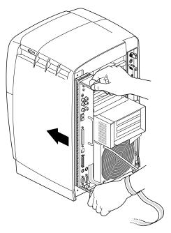
**Figure 2-24** Locking the System Module to the Frontplane
