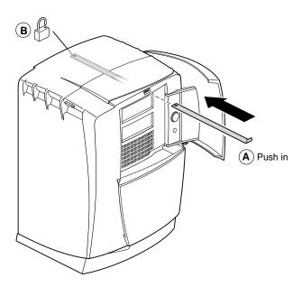
Figure 2-28 Installing the Lockbar
