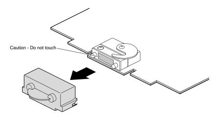
**Figure 2-22** Removing the Compression Connector Cap
