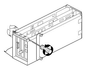
**Figure 4-37** Removing the I/O Door Screws
