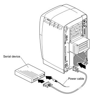
**Figure 6-13** Plugging In the Serial Cable
