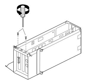
Figure 4-20 Removing the I/O Panel Screws
