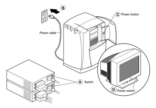
Figure 6-10 Turning On External Devices and the Octane2 Workstation
