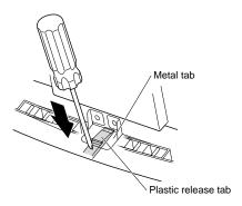
**Figure 7-33** Releasing the Plastic Base
