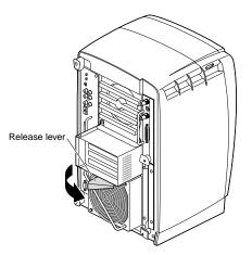
Figure 4-7 Opening the Release Lever
