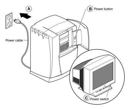
**Figure 6-9** Powering On the Octane2 Workstation
