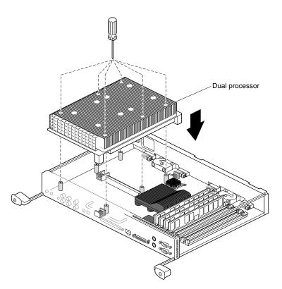
Figure 2-16 shows a dual processor installation.
