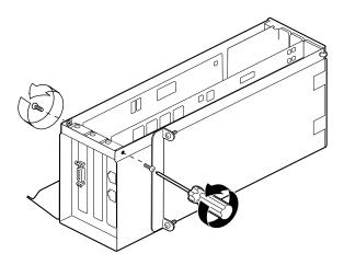
**Figure 4-21** Removing the I/O Door Screws
