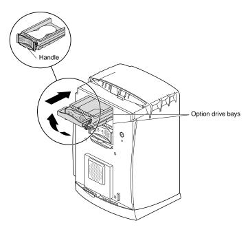
Figure 7-7 Inserting a Secondary (Option) Internal Drive
