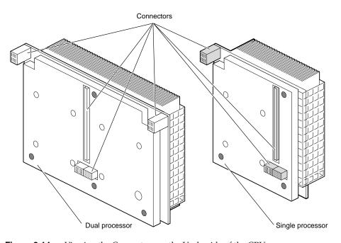
Figure 2-14 Viewing the Connectors on the Underside of the CPU
