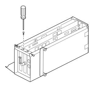
Figure 4-29 Removing the PCI Board Screw
