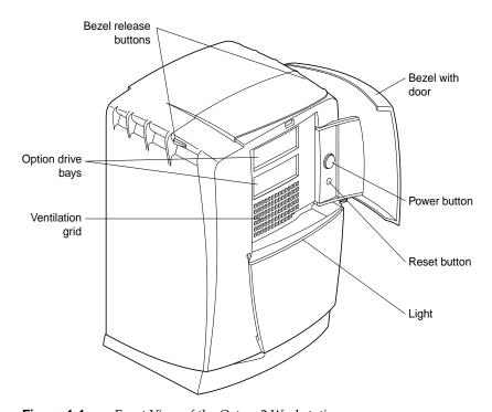
Figure 1-1 Front View of the Octane2 Workstation
