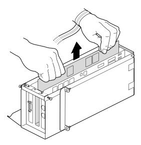
Figure 4-30 Extracting the PCI Board
