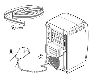
**Figure 4-5** Attaching the Wrist Strap to the Chassis
