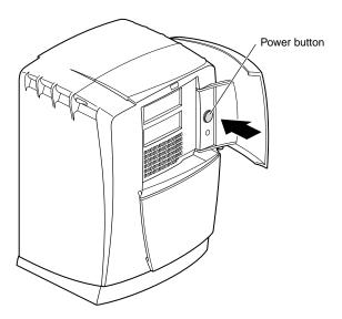
Figure 1-18 Powering On the Octane2 Workstation
