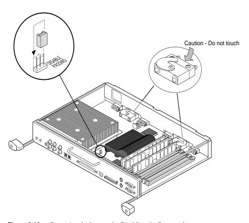
**Figure 8-10** Removing the Jumper for Disabling the Password
