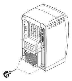
Figure 5-19 Tightening the XIO Tri-Module Screws
