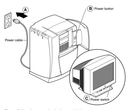
**Figure 5-21** Powering On the Octane2 Workstation
