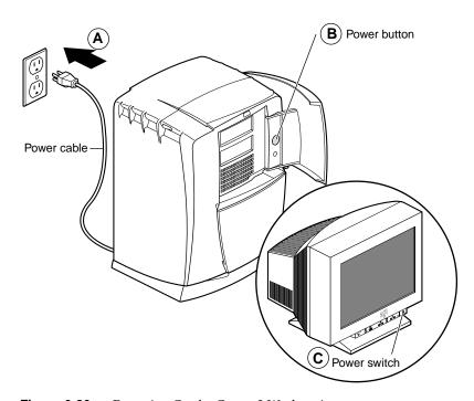
Figure 6-20 Powering On the Octane2 Workstation
