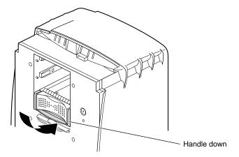
Figure 7-18 Locking the System Drive
