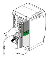
**Figure 5-9** Removing the XIO Tri-Module
