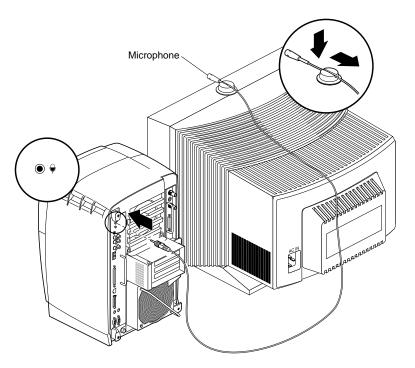
Figure 6-15 Installing the Microphone
