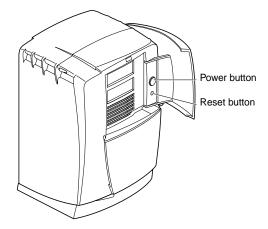
Figure 1-25 Power Button and Reset Button
