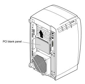
Figure 4-47 Removing the Blank Panel
