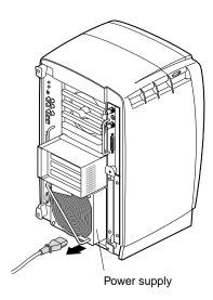
Figure 3-2 Unplugging the Power Cable
