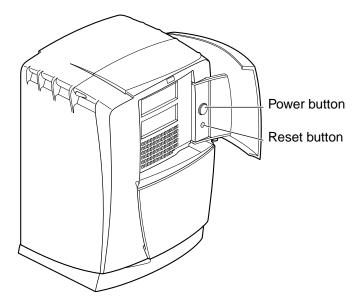
Figure 8-7 Pressing the Reset Button
