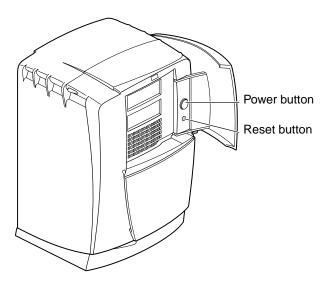
Figure 8-12 Power Button and Reset Button
