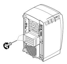
**Figure 4-51** Tightening the PCI Screws
