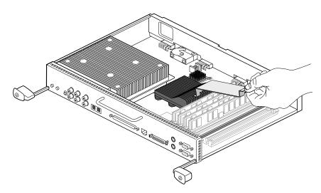
Figure 2-19 Removing the DIMM bracket
