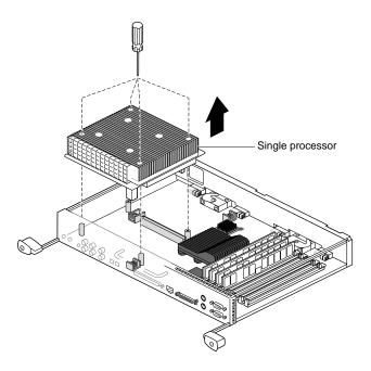
**Figure 2-11** Removing a Single Processor
