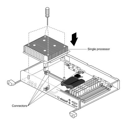
Figure 2-15 Installing a Single Processor
