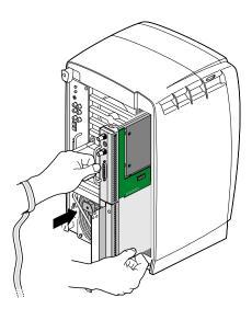
Figure 5-18 Inserting the XIO Tri-Module
