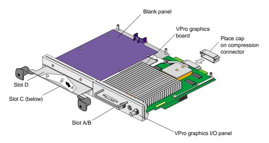
**Figure 5-10** Placing the XIO Tri-Module on Its Side
