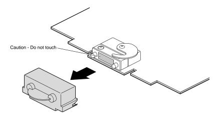
Figure 4-48 Removing the Cap from the Compression Connector
