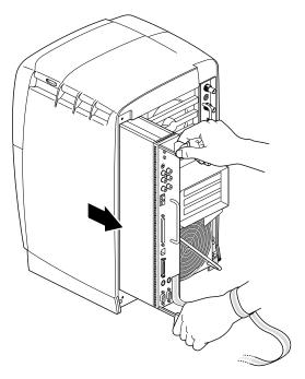
**Figure 2-6** Releasing the System Module from the Frontplane
