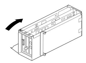
Figure 4-24 Closing the I/O Door
