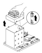
Figure 7-28 Removing the Fan From the Back of the Drive Bay
