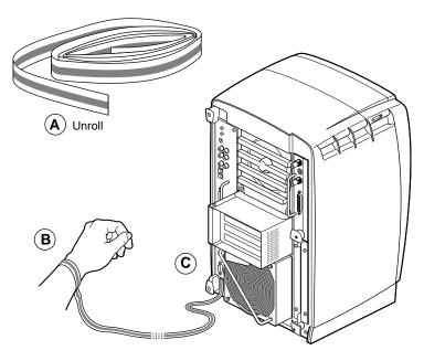
Figure 7-22 Attaching the Wrist Strap
