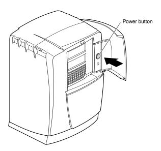
Figure 1-15 Powering On the Octane2 Workstation
