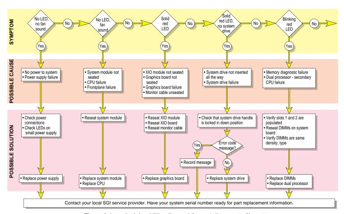
Figure 8-1 Lightbar LEDs - Front of Octane2, Diagnostic Chart #1
