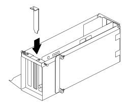
Figure 4-42 Inserting the I/O Blank Panel
