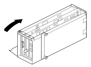
Figure 4-40 Closing the I/O Door
