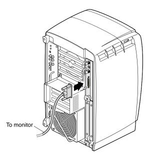
**Figure 5-20** Reconnecting the Monitor Cable
