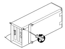
Figure 4-11 Loosening the Screws on the PCI Module
