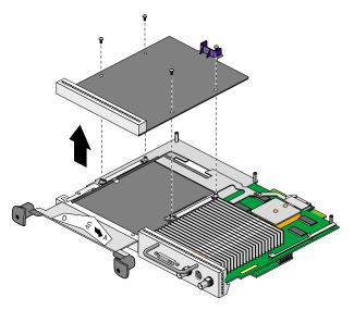
Figure 5-15 Removing the Blank Panel
