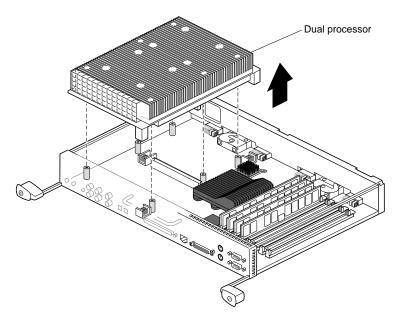
Figure 2-13 Lifting a Dual Processor from the System Module
