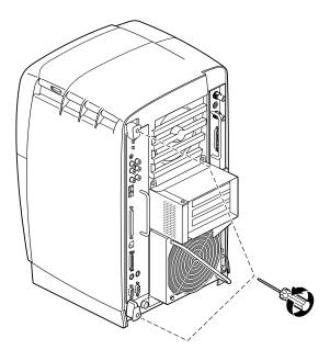
Figure 2-5 Loosening the System Module Screws
