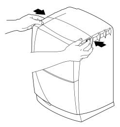
Figure 7-4 Pressing the Bezel Release Buttons
