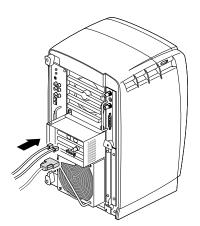
Figure 4-52 Installing the PCI Cables
