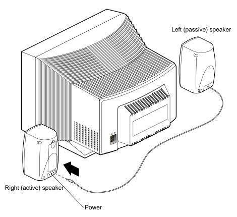
**Figure 1-7** Attaching the Speaker-to-Speaker Cable
