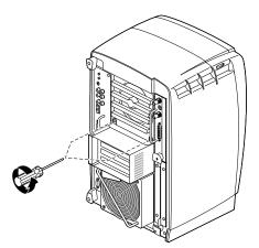
Figure 4-6 Removing the Screws From the PCI Module
