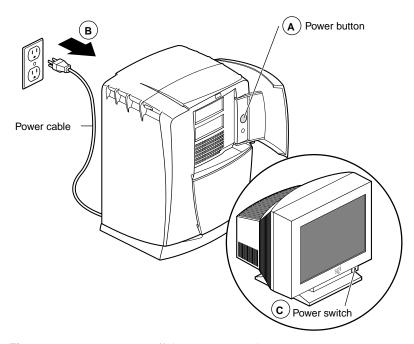
**Figure 4-3** Powering Off the Octane2 Workstation
