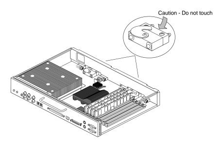
**Figure 2-8** Locating the Compression Connectors
