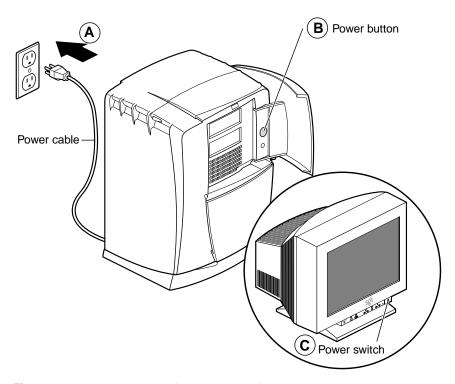
**Figure 3-8** Powering On the Octane2 Workstation
