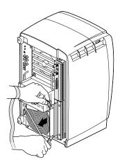
**Figure 5-8** Releasing the XIO Tri-Module
