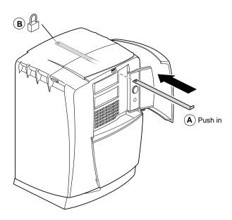
Figure 1-17 Inserting the Lockbar
