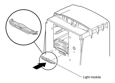
Figure 7-21 Inserting the Light Module
