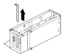
Figure 4-15 Removing the Blank I/O Panel
