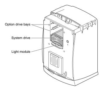
Figure 7-6 Identifying the Secondary (Option) Drive Bays
