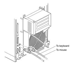
Figure 6-19 Disconnecting the Mouse and Keyboard
