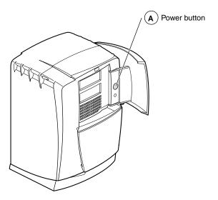
Figure 1-23 Powering Off the Octane2 Workstation
