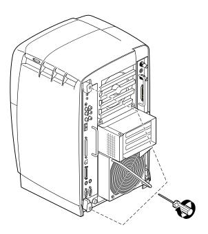
**Figure 2-25** Tightening the System Module Screws
