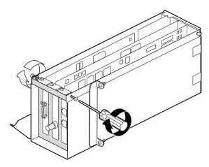
**Figure 4-25** Reinstalling the I/O Door Screws
