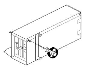
Figure 4-28 Tightening the PCI Module Door Screws
