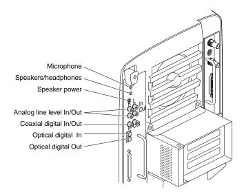
Figure 6-14 Audio Ports on the System Module
