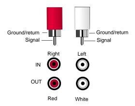
The following diagram shows the port (jack) pinout for the coaxial digital ports and plugs.
