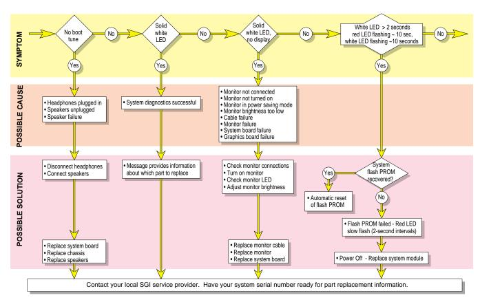
Figure 8-2 Lightbar LEDs - Front of Octane2, Diagnostic Chart #2
