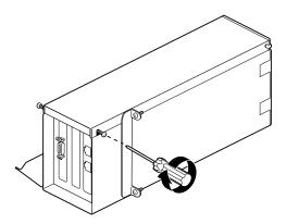
**Figure 4-45** Tightening the PCI Module Door Screws
