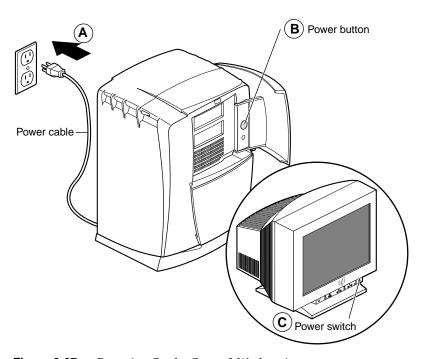
**Figure 2-27** Powering On the Octane2 Workstation
