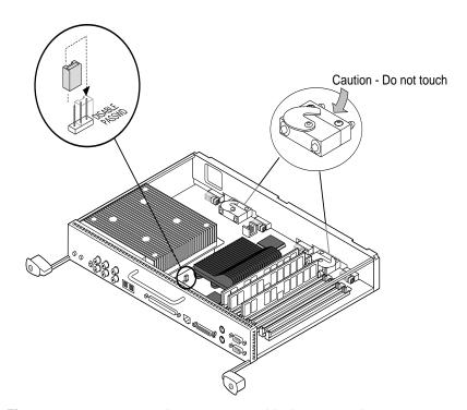
**Figure 8-11** Removing the Jumper to Enable the Password
