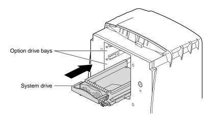
**Figure 7-17** Inserting the New Drive
