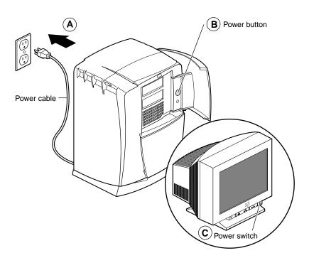
Figure 7-38 Powering on the Octane2 Workstation
