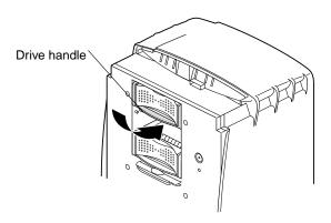
Figure 7-8 Locking the Secondary (Option) Drive
