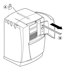
Figure 2-2 Removing the Lockbar
