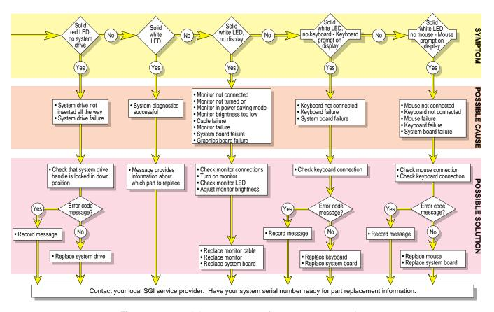
Figure 8-3 Lightbar LEDs - Front of Octane2, Diagnostic Chart #3
