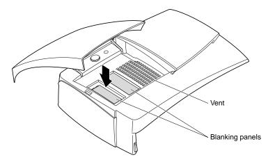
Figure 7-10 Releasing the Blank Panel
