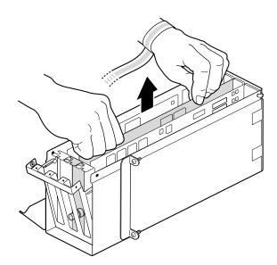
Figure 4-39 Removing a PCI Board
