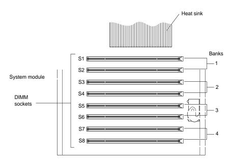
Figure 2-17 Identifying DIMM Sockets and DIMM Banks
