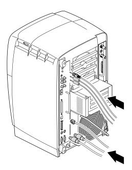
**Figure 2-26** Reconnecting Cables to the System Module
