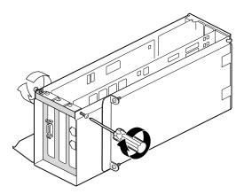
**Figure 4-31** Inserting the I/O Door Screws
