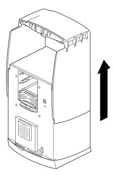
Figure 7-31 Sliding the Front Cover Forward
