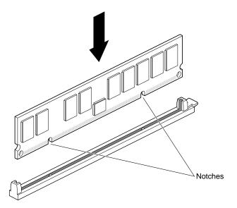
Figure 2-21 Locating the Notches on a DIMM
