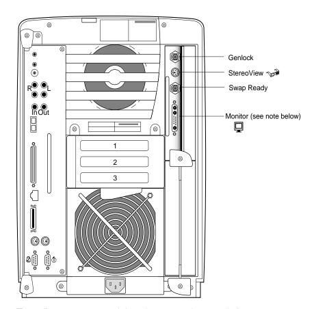
Figure 5-2 shows the XIO Tri-Module and each of the VPro graphics board I/O ports.
