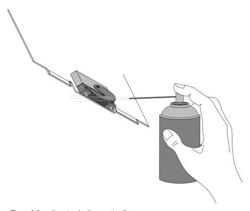
**Figure A-2** Spraying the Compression Connector
