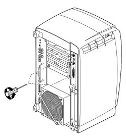
**Figure 4-46** Removing the Screws from the Blank Panel
