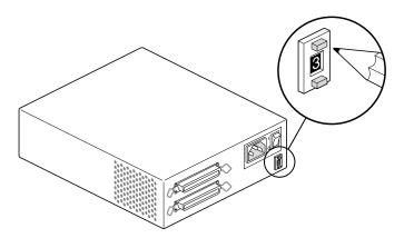
Figure 6-1 Manually Setting the SCSI Address
