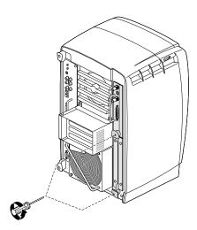
Figure 5-7 Removing the XIO Tri-Module Screws
