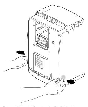
**Figure 7-30** Releasing the Plastic Top Cover
