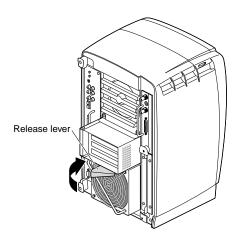
Figure 4-50 Closing the Release Lever
