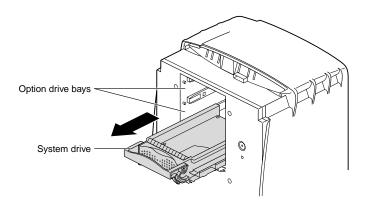
**Figure 7-16** Removing the System Drive
