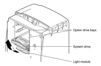
**Figure 7-15** Unlocking the System Drive
