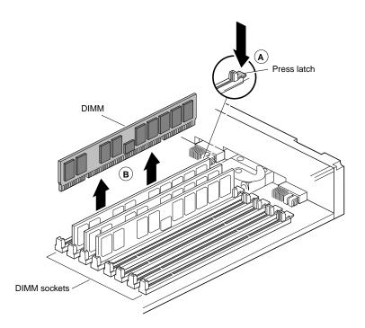
Figure 2-20 Removing a DIMM
