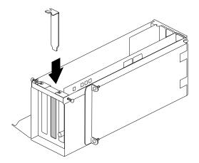
Figure 4-32 Inserting the I/O Blank Panel
