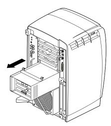
Figure 4-8 Removing the PCI Module
