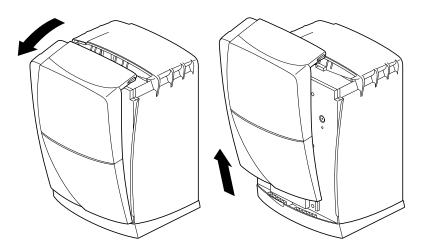
Figure 7-5 Removing the Bezel
