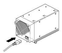
**Figure 3-5** Plugging In the Power Cable
