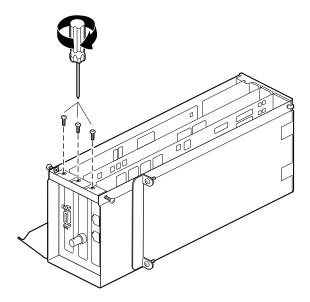
**Figure 4-26** Reinstalling the I/O Panel Screws
