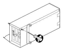
**Figure 4-19** Tightening the I/O Door Screws
