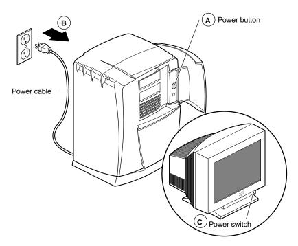
**Figure 5-3** Powering Off the Octane2 Workstation
