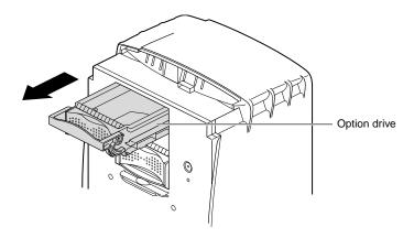
Figure 7-12 Sliding Out the Secondary (Option) Drive
