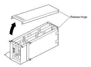
Figure 4-12 Opening and Removing the PCI Module Door
