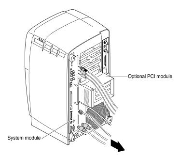
**Figure 2-3** Removing the Cables from the System Module
