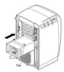
Figure 4-49 Installing the PCI Module
