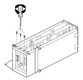
Figure 4-36 Removing the I/O Panel Screws
