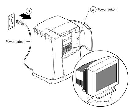
**Figure 3-1** Powering Off the Octane2 Workstation
