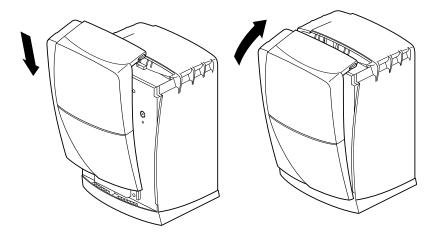
Figure 7-36 Reinstalling the Bezel
