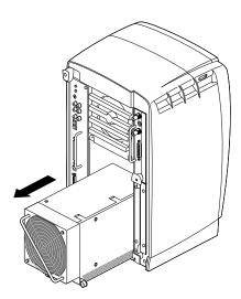
**Figure 3-4** Removing the Power Supply
