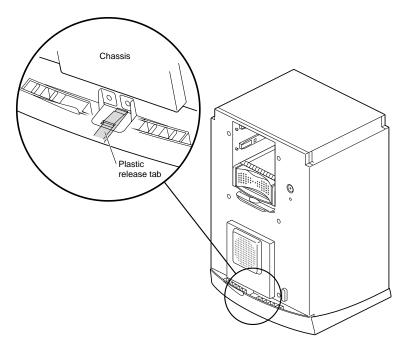
**Figure 7-32** Locating the Release Slots
