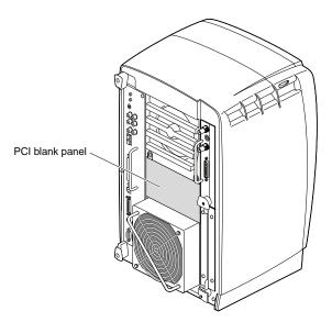
Figure 4-1 Workstation without the Optional PCI Module
