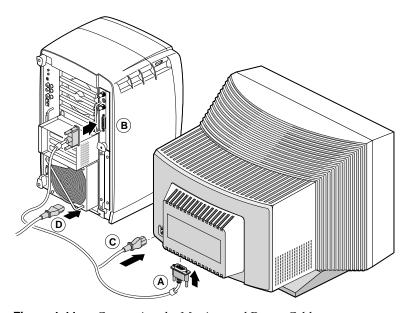
**Figure 1-11** Connecting the Monitor and Power Cables
