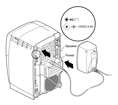
**Figure 1-9** Connecting the Speaker and Power Cables
