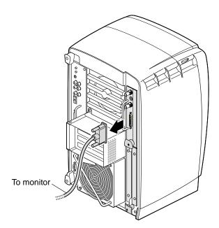
Figure 5-4 Removing the Monitor Cable
