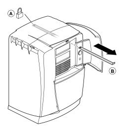
**Figure 7-3** Unlocking and Removing the Lockbar
