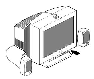
**Figure 1-13** Powering On the Monitor
