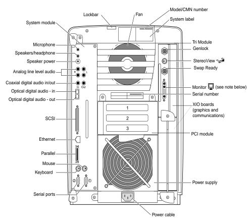
Figure 1-2 Back View of the Octane2 Workstation
