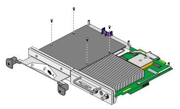
**Figure 5-14** Removing the Screws from the Blank Panel
