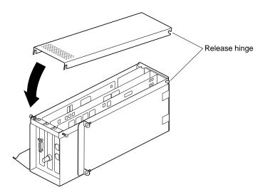
**Figure 4-18** Placing the Door on the PCI Module
