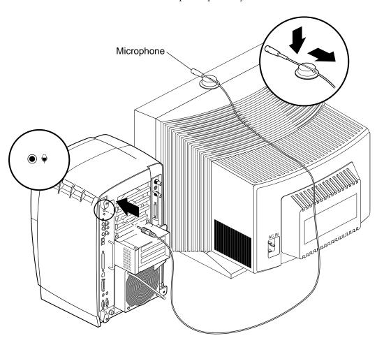
**Figure 1-10** Attaching the Microphone
