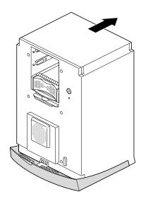
Figure 7-34 Sliding the Chassis Backward
