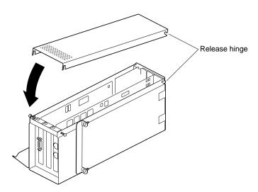
Figure 4-44 Reinstalling the PCI Module Door
