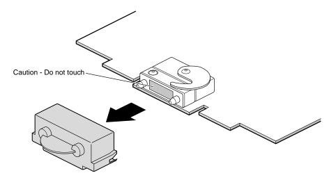
Figure 5-17 Removing the Cap from the XIO Board Compression Connector
