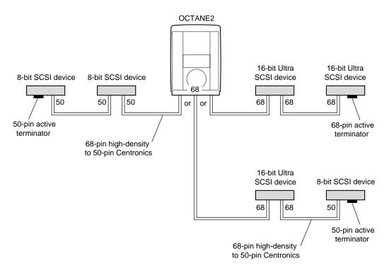
Figure 6-4 Using the Correct Cables between Devices and/or the Octane2 Workstation
