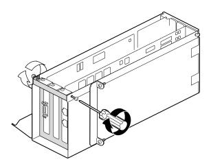
**Figure 4-41** Inserting the I/O Door Screws
