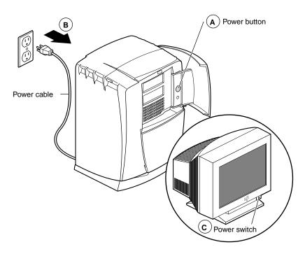
**Figure 7-1** Powering Off the Octane2 Workstation and Monitor
