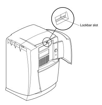
Figure 1-16 Locating the Lockbar Slot
