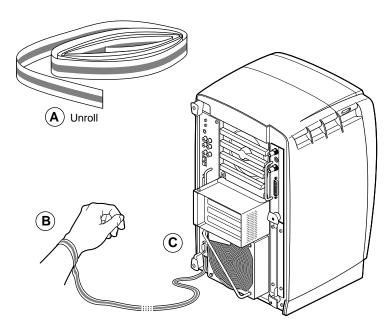
Figure 5-5 Attaching the Wrist Strap
