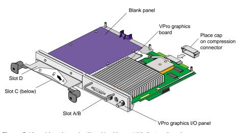
Figure 5-12 Identifying the Slots Used by an XIO Option Board
