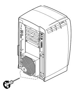
**Figure 3-7** Inserting and Tightening the Screws
