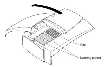
**Figure 7-9** Opening the Bezel Door
