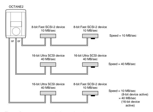
**Figure 6-5** Comparing Speed of Daisy-Chained Devices
