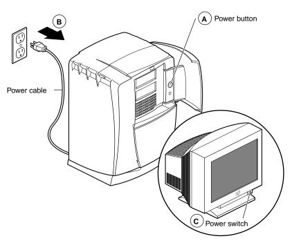
**Figure 6-2** Powering Off the Octane2 Workstation
