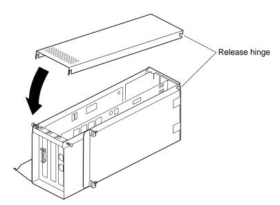
Figure 4-34 Reinstalling the PCI Module Door
