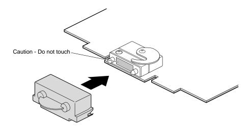
Figure 2-10 Placing the Compression Cap on the Compression Connector
