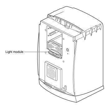
Figure 7-19 Locating the Light Module
