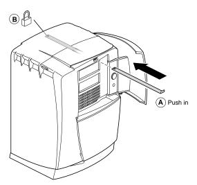
Figure 7-37 Replacing the Lockbar
