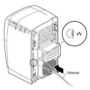
**Figure 1-6** Attaching the Ethernet Cable
