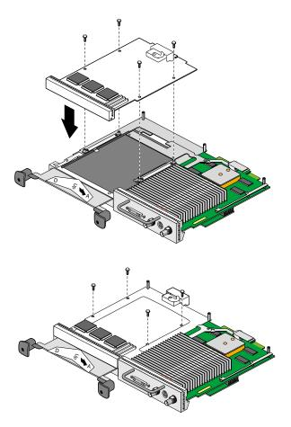
Figure 5-16 Installing the Screws
