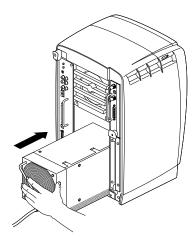
**Figure 3-6** Sliding In the New Power Supply
