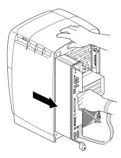
Figure 2-7 Removing the System Module from the Chassis
