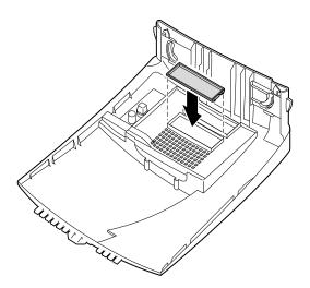
**Figure 7-13** Replacing the Blank Panel
