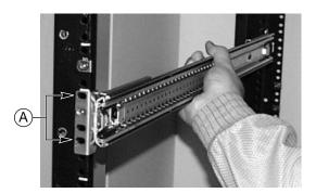
Figure 8 Slide Rail Assembly Aligned with Holes in Rack
