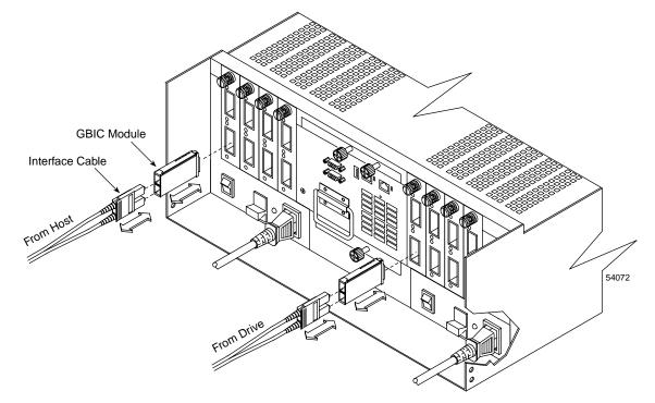
3. Remove the interface cables from the failed GBIC module (Figure 4-12).
