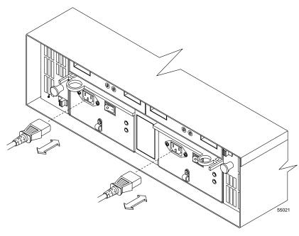
Figure 8-14 Connecting the Drive Enclosure Power Cords
