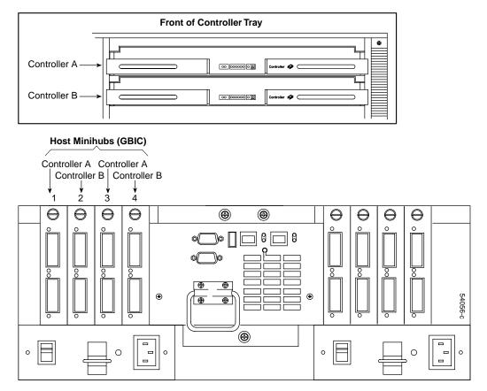
Figure 2-12Controller Enclosure Host Interface Connectors
