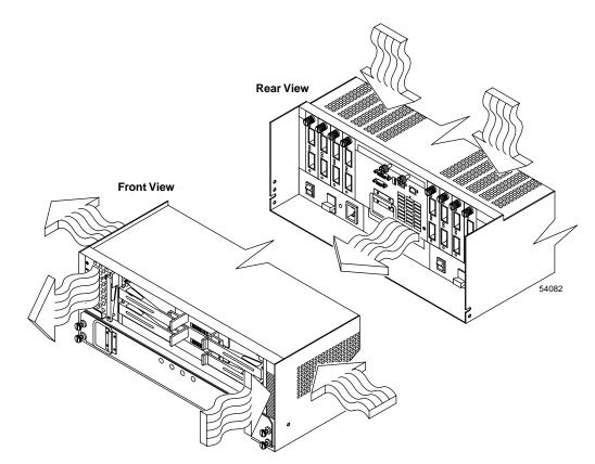
Figure 2-7 Controller Enclosure Air Flow
