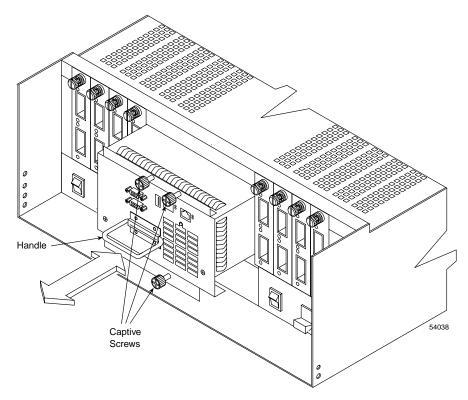
Figure 4-9 Removing and Installing a Fan/Communications Canister
