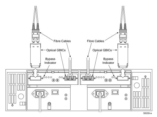
Figure 5-10 Fibre Channel Cables and GBICs
