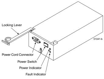
Figure 5-7Power Supply Canister
