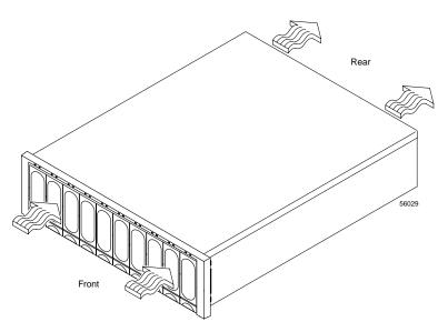
Figure A-9 Drive Enclosure Air Flow
