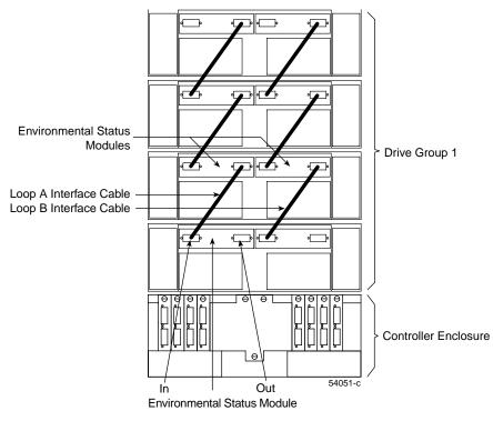
Figure 8-2 Connecting Additional Drive Enclosures to Drive Loops A and B
