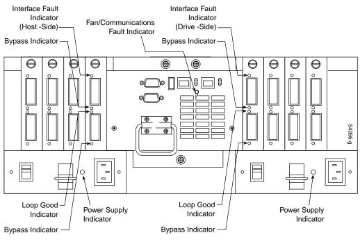
Figure 3-6 and Table 3-2 describe the indicator lights on the rear of the controller enclosure.
