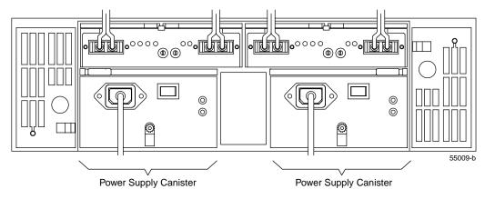
Figure 5-6 Power Supply Canisters in a Drive Enclosure
