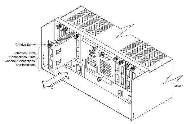
6. Unfasten the captive screw on the minihub and remove it from the chassis (Figure 4-13).
