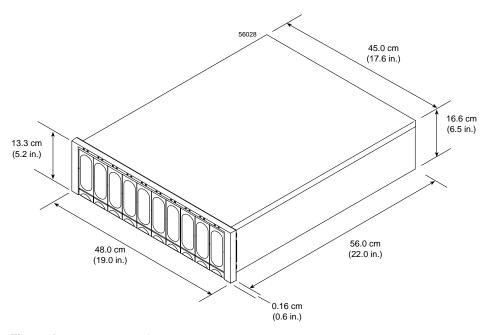
Figure A-8 Drive Enclosure Dimensions
