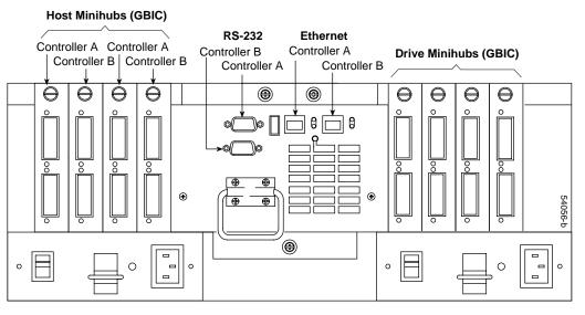
Figure 2-3 Interface Components (Rear)
