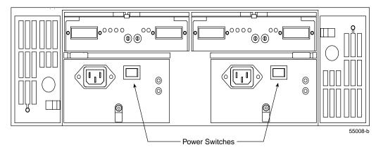
Figure 6-1Turning the Power On and Off
