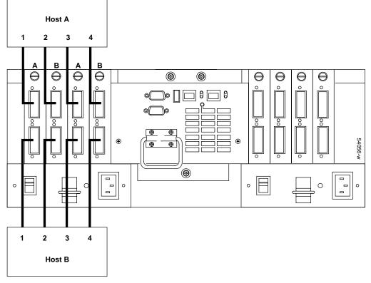
Figure 8-8 shows two hosts directly connected. These hosts share controller bandwidth.
