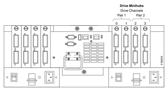
Figure 2-13 Controller Enclosure Drive Minihub Connectors (Rear)
