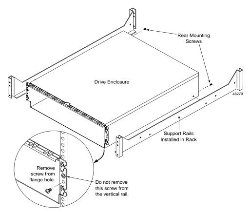
Figure 6-7 Removing the Empty Drive Enclosure
