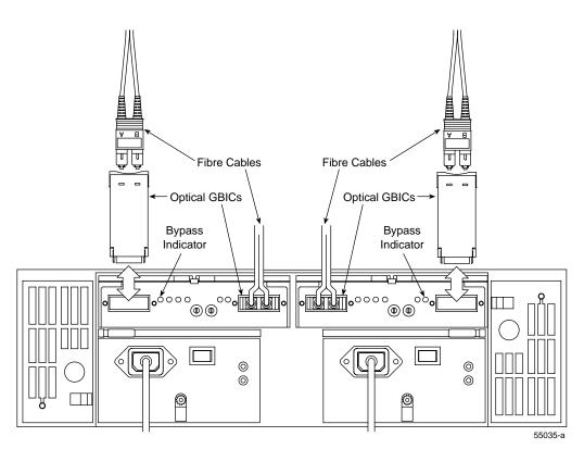
Figure 7-6 Removing and Installing a GBIC
