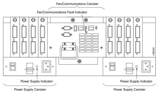
Figure 3-3 Fan/Communications and Power Supply Indicators (Rear)
