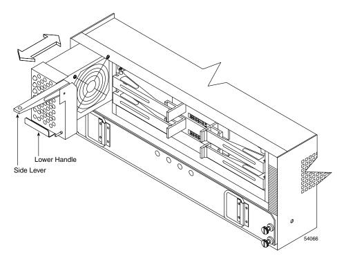
Figure 4-6 Removing and Installing a Controller Fan Canister
