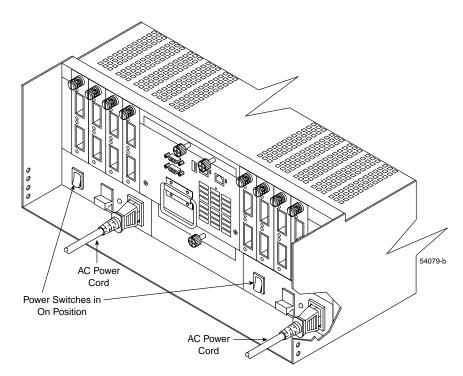
Figure 3-2 Turning the Power On
