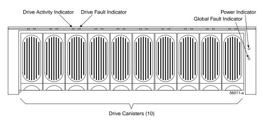
Figure 5-1Front View of the Drive Enclosure
