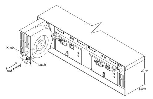
Figure 7-2 Removing and Installing a Fan Canister
