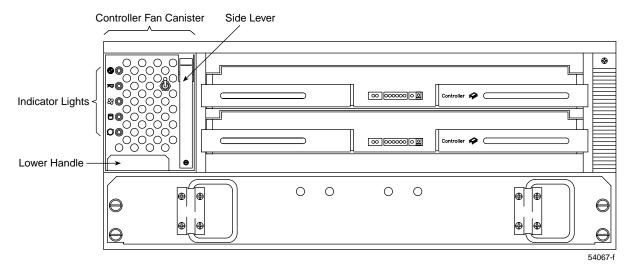
Figure 2-6 Controller Fan Canister
