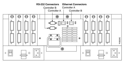
Figure 8-12 Connecting Ethernet and Serial Interface Cables
