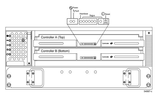
Figure 2-4Redundant Controllers and Indicator Lights
