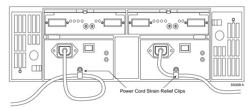
Figure 8-15 Securing the Power Cords in the Cord Clips
