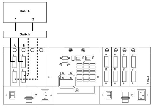
Figure 8-9 Switch Connect — 1 Host - 2 HBA
