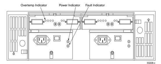
Figure 6-2 Overtemp, Power, and Fault Indicators
