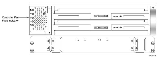
Figure 3-4 Controller Fan Fault Indicator (Front)
