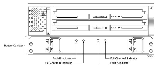
Figure 2-5 Battery Canister
