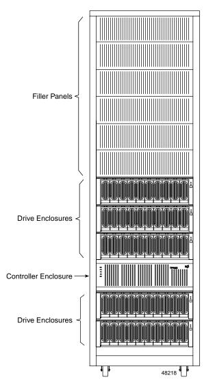
Figure A-1 TP9400 with Controller Enclosures and Drive Enclosures
