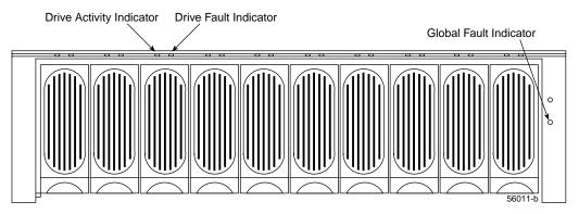
Figure 6-3 Activity and Fault Indicators on Front of Drive Enclosure
