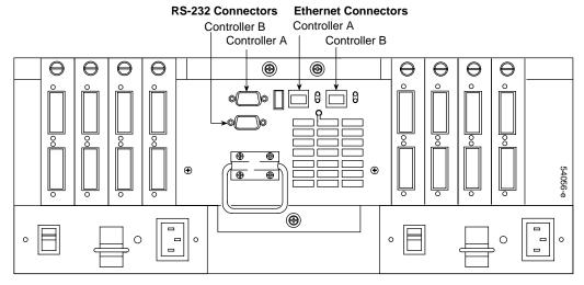
Figure 2-9 Controller Enclosure Diagnostic Interface Connectors (Rear)
