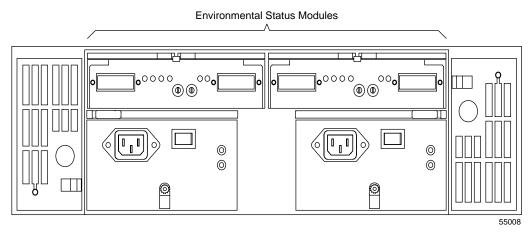
**Figure 5-8** Environmental Status Modules in the Drive Enclosure
