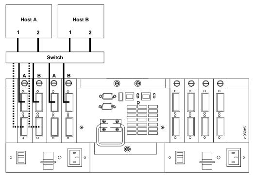
Figure 8-10Switch Connect — 2 Host - 2 HBA/Host
