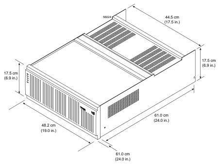
Figure A-6 Controller Enclosure Dimensions
