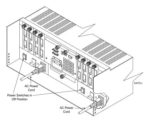
Figure 8-13Connecting the Controller Enclosure Power Cords
