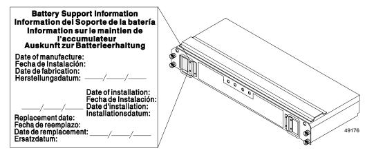
Figure 3-7 Checking the Battery Service Date
