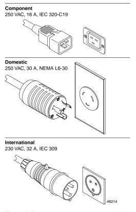
Figure A-5 AC Power Connectors and Receptacles
