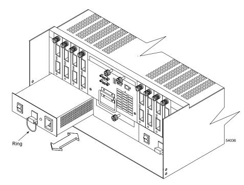
4. Remove the failed power supply (Figure 4-11). Pull the ring to release the canister and slide it out.
