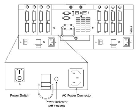
Figure 4-10 Power Supply Switch, Connector, and Indicator
