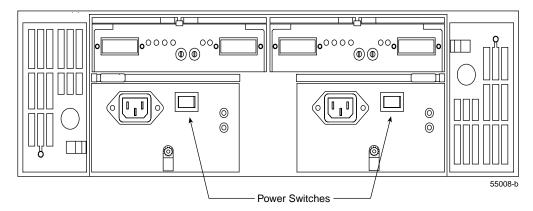
Figure 8-16 The Drive Enclosure Power Switches
