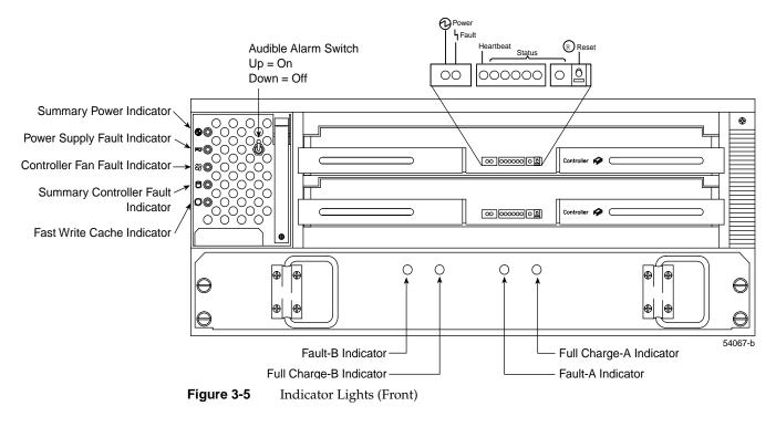
**Note:** You have the option of using the audible alarm to warn you of faults (Figure 3-5). The alarm is turned on (in upward position) when shipped. To disable the alarm, flip the switch to the downward position.
