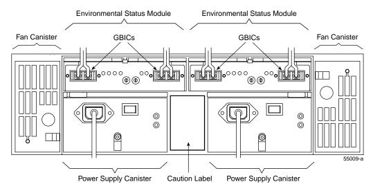
Figure 5-2 Rear View of the Drive Enclosure
