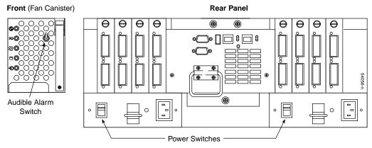
Figure 8-17 The Controller Enclosure Power Switches and Alarm Switch
