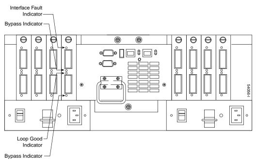
Figure 2-11 Minihub Canister and indicator lights
