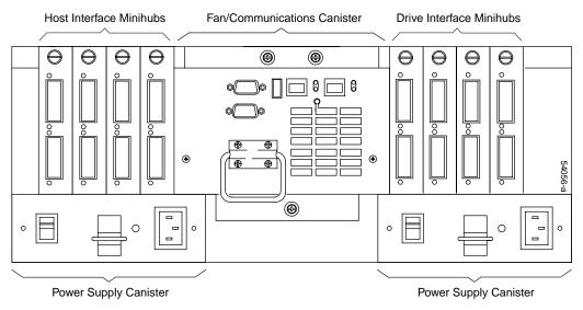
Figure 2-2 Rear View of the Controller Enclosure
