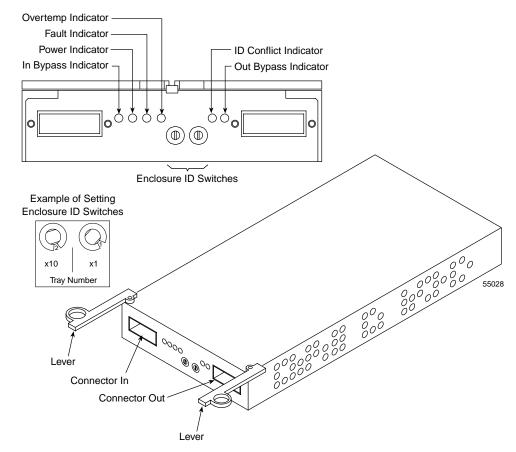
Figure 5-9 Environmental Status Module Indicators and Connectors
