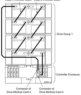
Loop A Interface Cable Loop B Interface Cable
