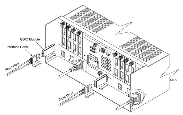
Figure 2-14Removing and Installing a GBIC Module
