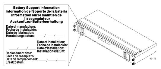
**Figure 3-8** Checking the Battery Service Date
