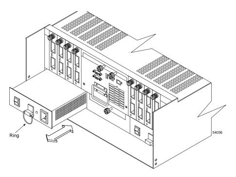
Figure 4-12 Removing and Installing a Power Supply Canister
