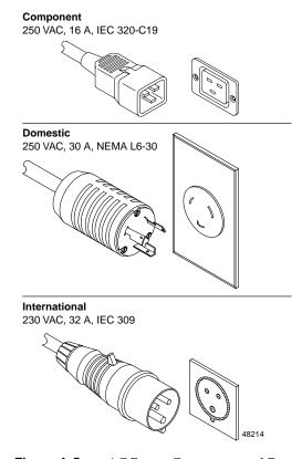
**Figure A-5** AC Power Connectors and Receptacles
