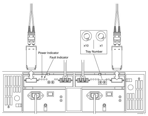
**Figure 7-7** Removing GBICs from the Environmental Status Module
