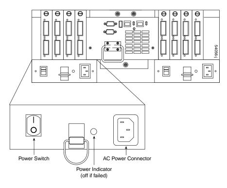
Figure 4-11 Power Supply Switch, Connector, and Indicator
