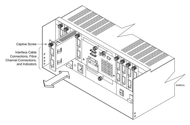
Figure 4-15 Removing and Installing a Minihub
