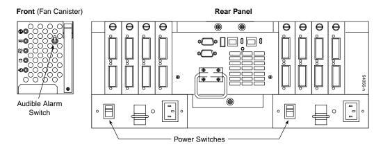
Figure 8-18 The Controller Enclosure Power Switches and Alarm Switch
