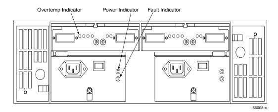
**Figure 6-2** Overtemp, Power, and Fault Indicators
