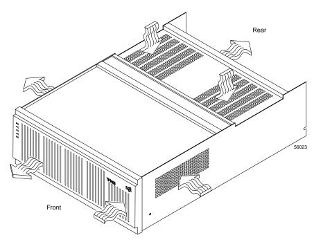
Figure A-7 Controller Enclosure Air Flow
