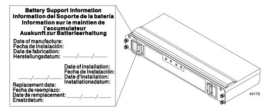
**Figure 4-4** Recording the Battery Support Information
