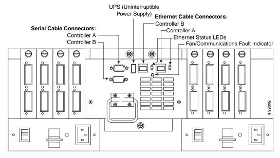
Figure 4-9 Fan/Communications Interface Cables and Fault Indicator
