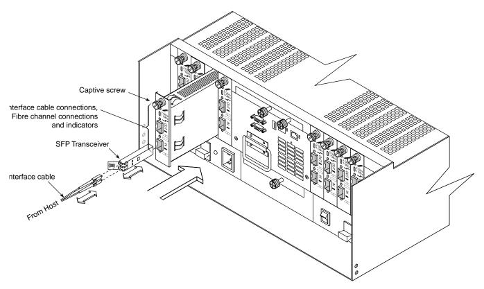
Figure 4-14 Removing and Installing an SFP transceiver
