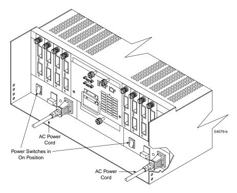
**Figure 3-2** Turning the Power On
