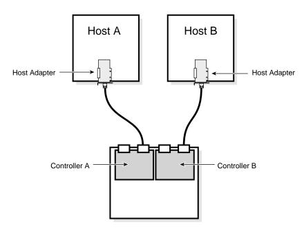
Figure 8-8 Direct Host Connect for Non fail-over Configuration
