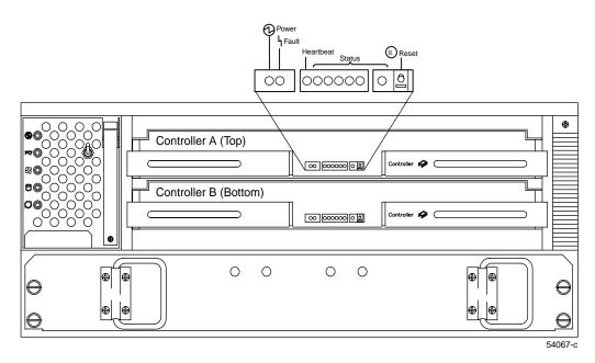
Figure 2-6 Redundant Controllers and Indicator Lights
