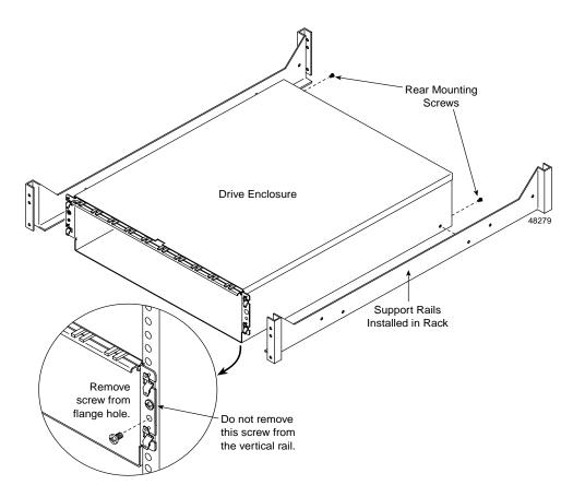
**Figure 6-7** Removing the Empty Drive Enclosure
