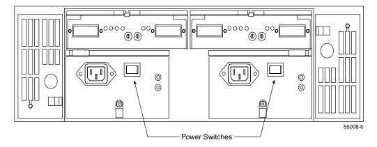
**Figure 8-17** The Drive Enclosure Power Switches
