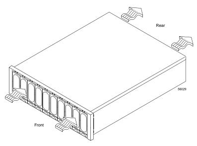
Figure A-9 Drive Enclosure Air Flow
