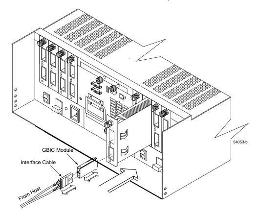
Figure 2-4 GBIC Minihub with GBIC Module
