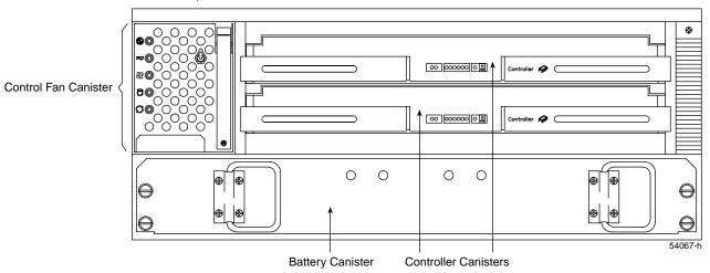
**Figure 2-1** Front View of the Controller Enclosure
