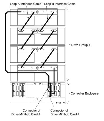
**Figure 8-4** Cabling Redundant Drive Loops to the Controller
