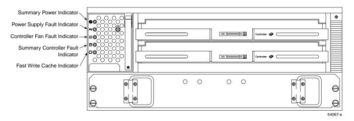
Figure 4-8 Controller Fan Indicators
