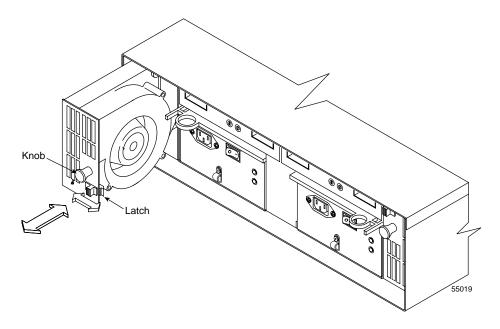
**Figure 7-2** Removing and Installing a Fan Canister
