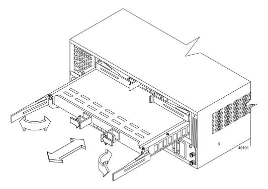
**Figure 4-2** Removing and Installing a Controller Canister
