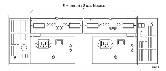
**Figure 5-8** Environmental Status Modules in the Drive Enclosure
