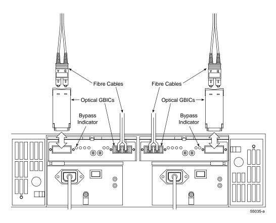
**Figure 7-6** Removing and Installing a GBIC
