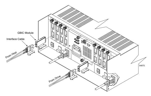
**Figure 4-13** Removing and Installing a GBIC Module
