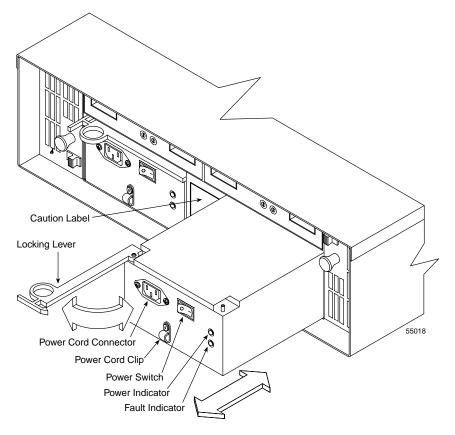
**Figure 7-4** Removing and Installing a Power Supply Canister
