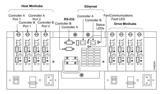
Figure 2-3 TP9400 Interface Components
