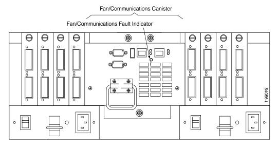
Figure 2-10 Fan/Communications Canister and Fault Indicator
