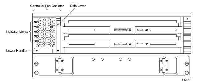
Figure 2-8 Controller Fan Canister
