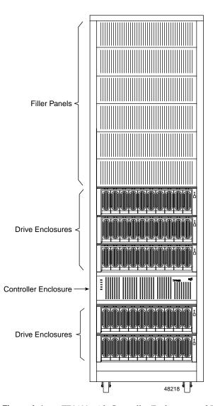
Figure A-1 TP9400 with Controller Enclosures and Drive Enclosures
