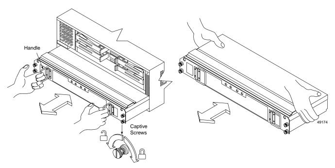
**Figure 4-5** Removing and Installing a Battery Canister
