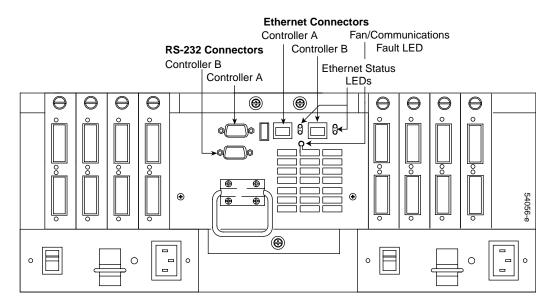
Figure 2-11 Controller Enclosure Diagnostic Interface Connectors (Rear)
