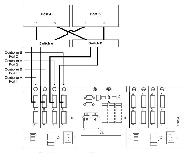
**Figure 8-12** Multi-Switch Connect — 2 Host
