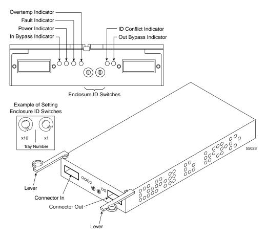
**Figure 5-9** Environmental Status Module Indicators and Connectors
