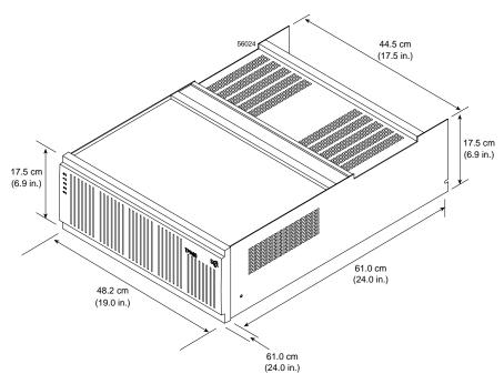
Figure A-6 Controller Enclosure Dimensions
