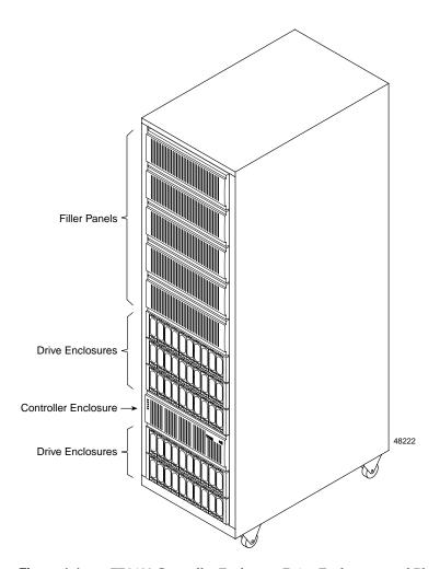
Figure 1-1 TP9400 Controller Enclosure, Drive Enclosures, and Blank Panels
