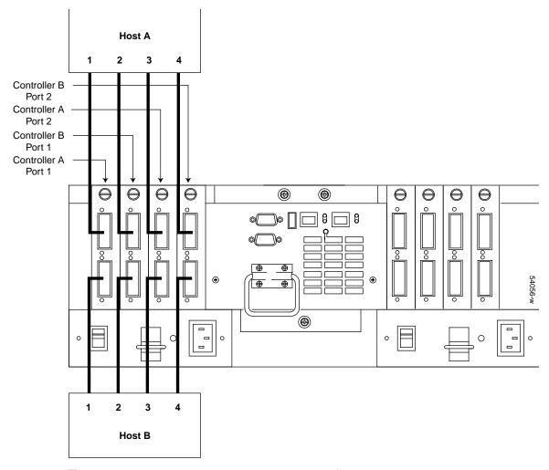
**Figure 8-9** Direct Host Connect — 2 Host - 4 HBA/Host
