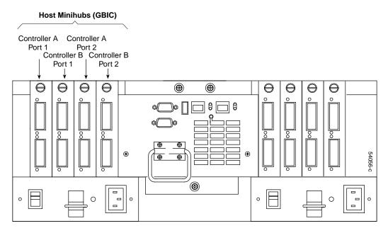
Figure 2-14 Controller Enclosure Host Interface Connectors
