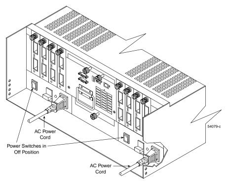
Figure 8-14 Connecting the Controller Enclosure Power Cords
