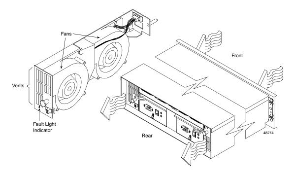
**Figure 5-5** Fan Canister and Drive Enclosure Air Flow
