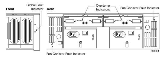
Figure 7-3 Fault Lights for Fan Canister Replacement
