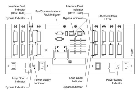
**Figure 3-6** 1 GB Interface Controller Rear Indicator Lights (GBIC)
