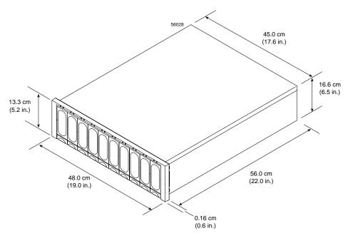
Figure A-8 Drive Enclosure Dimensions
