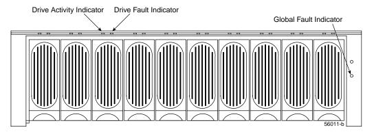
**Figure 6-3** Activity and Fault Indicators on Front of Drive Enclosure
