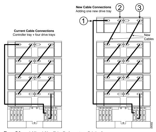
Figure 7-9 Adding A New Drive Enclosure to an Existing Loop
