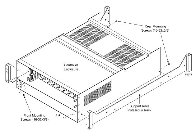
**Figure 3-9** Removing the Controller Enclosure from the Rack
