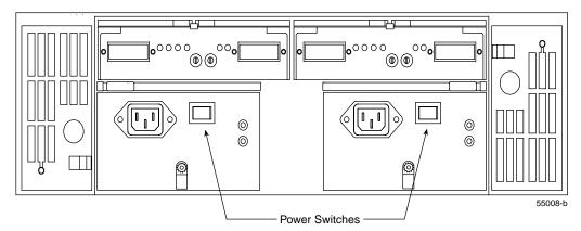
**Figure 6-1** Turning the Power On and Off
