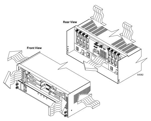
Figure 2-9 Controller Enclosure Air Flow
