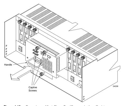
Figure 4-10 Removing and Installing a Fan/Communications Canister
