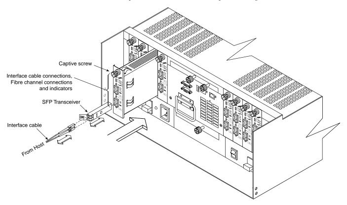
**Figure 2-17** Removing and Installing an SFP Transceiver
