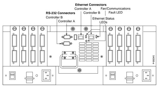
Figure 8-13 Connecting Ethernet and Serial Interface Cables
