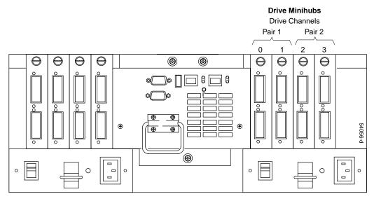
Figure 2-15 Controller Enclosure Drive Minihub Connectors (Rear)
