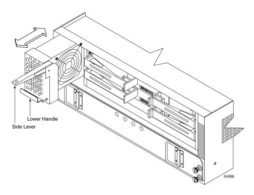
Figure 4-7 Removing and Installing a Controller Fan Canister
