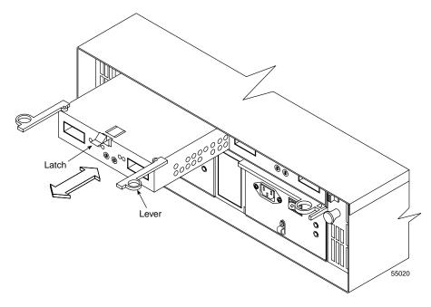
Figure 7-8 Removing and Installing an Environmental Status Module
