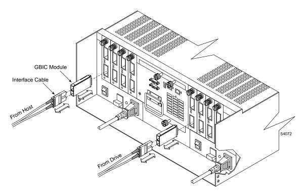
**Figure 2-16** Removing and Installing a GBIC Module
