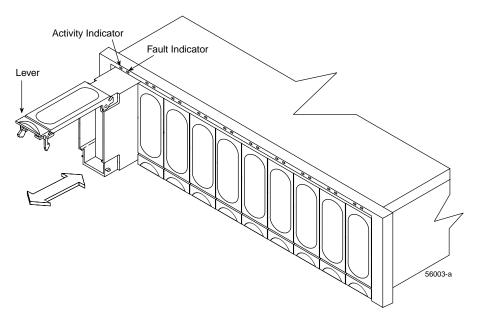
**Figure 7-1** Removing and Installing a Drive Sled
