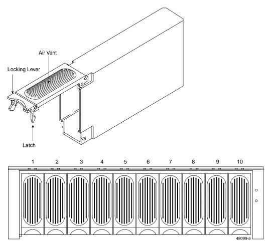
Figure 5-4 Drive Sleds and Drive Numbering
