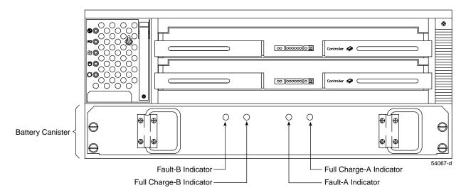
Figure 2-7 Battery Canister
