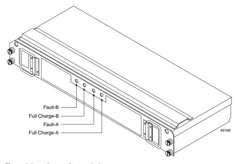
Figure 4-6 Battery Canister Indicators
