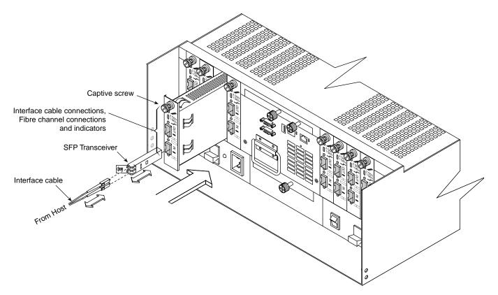
**Figure 2-5** SFP Minihub with SFP Transceiver
