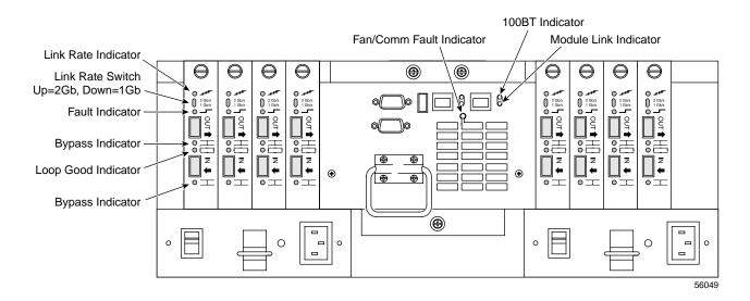
**Figure 3-7** 2 GB Interface Controller Rear Indicator Lights (SFP)
