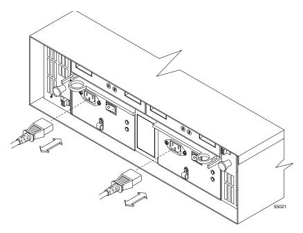
**Figure 8-15** Connecting the Drive Enclosure Power Cords
