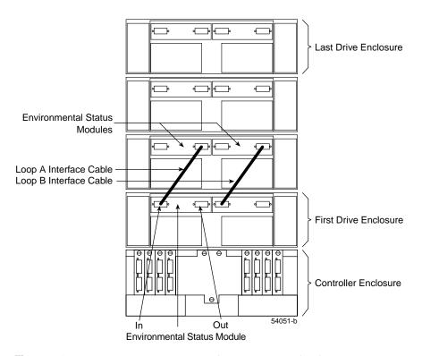
Figure 8-1 Connecting Two Drive Enclosures Into a Redundant Drive Loop
