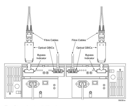
Figure 5-10 Fibre Channel Cables and GBICs
