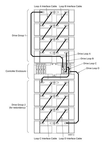
**Figure 8-5** Two Drive Groups, Each With Redundant Drive Loops
