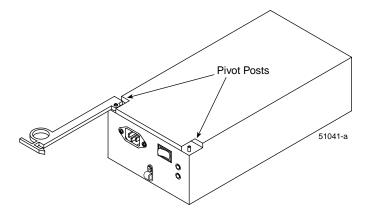
Figure 7-5 Power Supply Canister Lever
