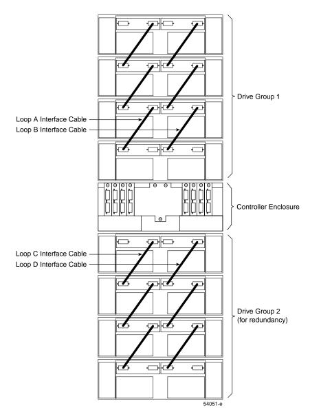
Figure 8-3 Connecting a Second Redundant Drive Loop
