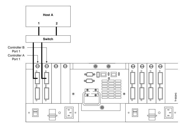
**Figure 8-10** Switch Connect — 1 Host - 2 HBA
