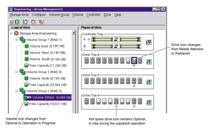
Figure 2-11 Status Changes During Example Recovery Operation
