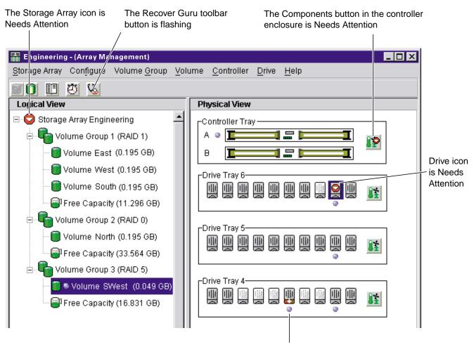
The hot spare drive is In Use (taking over for a failed drive). This means that the data from the fariled drive has been reconstructed to the hot spare drive. Because the hot spare drive has taken over for the failed drive, the associated volume (Volume SWest) in Volume Group 3 remains Optimal.
