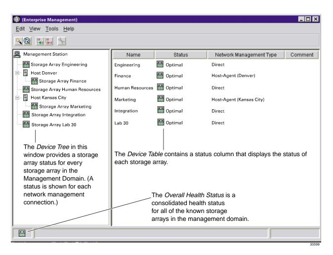
Figure 2-7 Monitoring the Health of Storage Arrays
