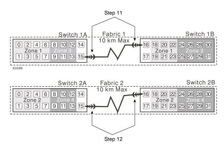
**Figure 3-20** Connecting Switches over a Remote Network to Complete Fabric Environments
