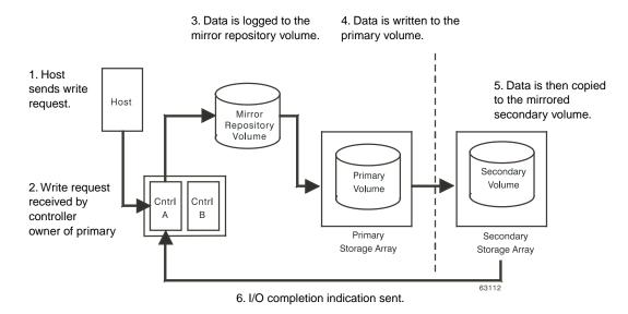
**Figure 3-3** Data Replication between Storage Arrays
