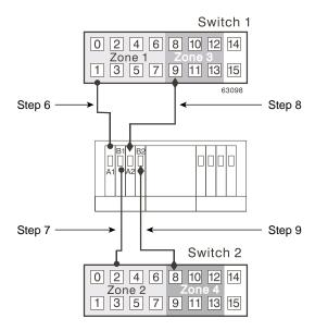
**Figure 3-19** Storage Array Connections to Fibre Channel Switches
