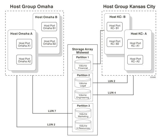
**Figure 2-2** Storage Partitioning Example
