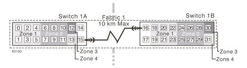
**Figure 3-22** Switch Zoning for the Campus Configuration
