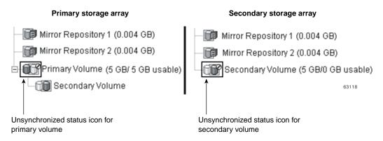
Figure 3-4 Mirrored Volume Pair in Unsynchronized Status
