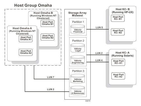
**Figure 2-5** Heterogeneous Hosts Example
