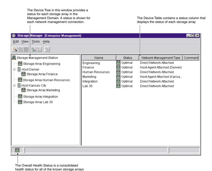
Figure 2-6 Monitoring the Health of Storage Arrays Using the Enterprise Management Window
