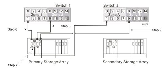
**Figure 3-30** Primary Storage Array Connections to Fibre Channel Switches
