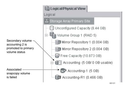
Figure 3-11 Snapcopy Volume Failure Because of Role Reversal
