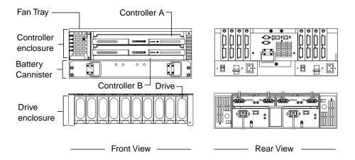
Figure 1-1 Physical Components of a Storage Array
