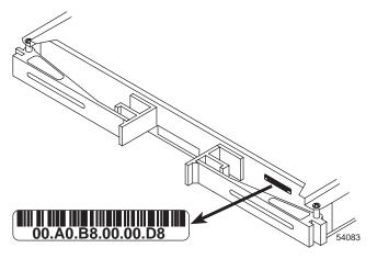
Figure 2-5 Identifying the Controller Ethernet Address
