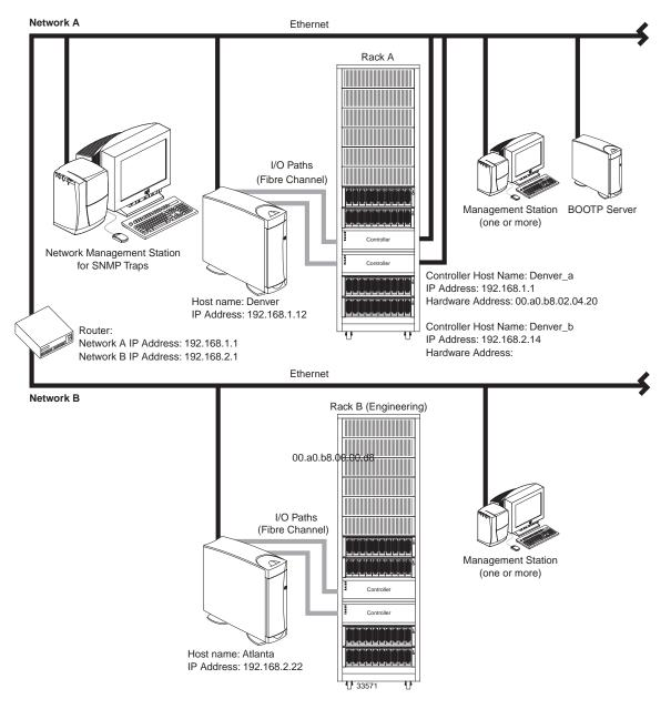
Figure 2-3 Example — Network Using Directly and Host-Agent Managed Storage Arrays
