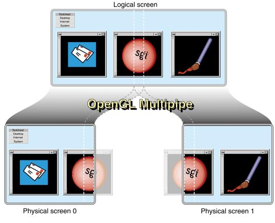
Figure 1-2OpenGL Multipipe with Overlapping Screens
