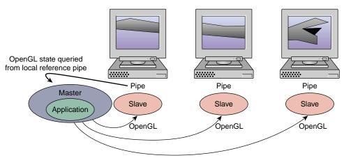
Figure 3-2 Running in -mstrmode track Mode
