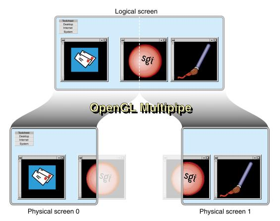
Figure 1-1OpenGL Multipipe with Non-Overlapping Screens
