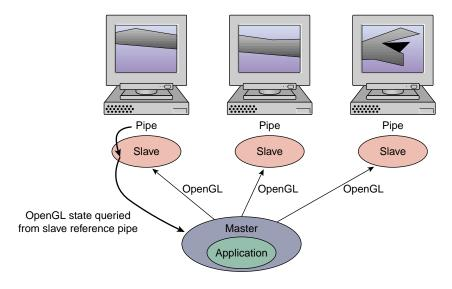
Figure 3-1 Running in -mstrmode off Mode
