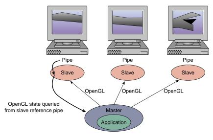
Figure 4-1 Running in Master Mode off
