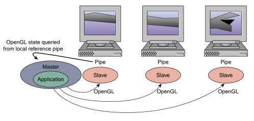
Figure 4-2 Running in Master Mode track
