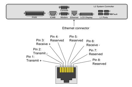
Figure B-11 shows the pin number locations and pin assignments for the Ethernet connector on the L2 controller hardware for the SGI Origin and Onyx 300 and 350 with NUMAlink Module.
