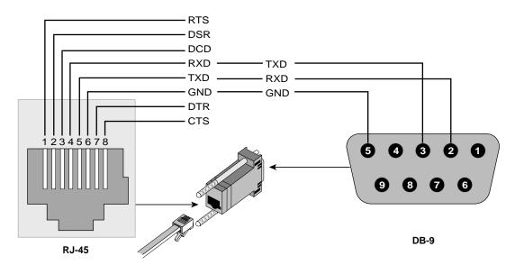
Figure B-2 RJ-45 to DB-9 Serial Adapter Pin Assignments
