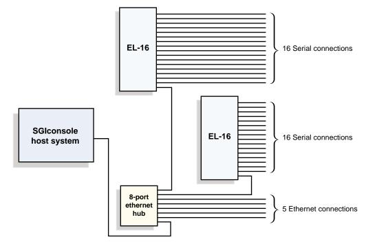
Figure 2-9 Sample Cabling Configuration: One Ethernet Hub, Two Serial Port Servers
