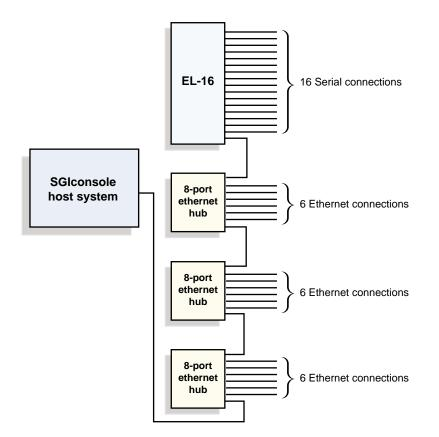
Figure 2-8 Sample Cabling Configuration: Three Ethernet Hubs, One Serial Port Server
