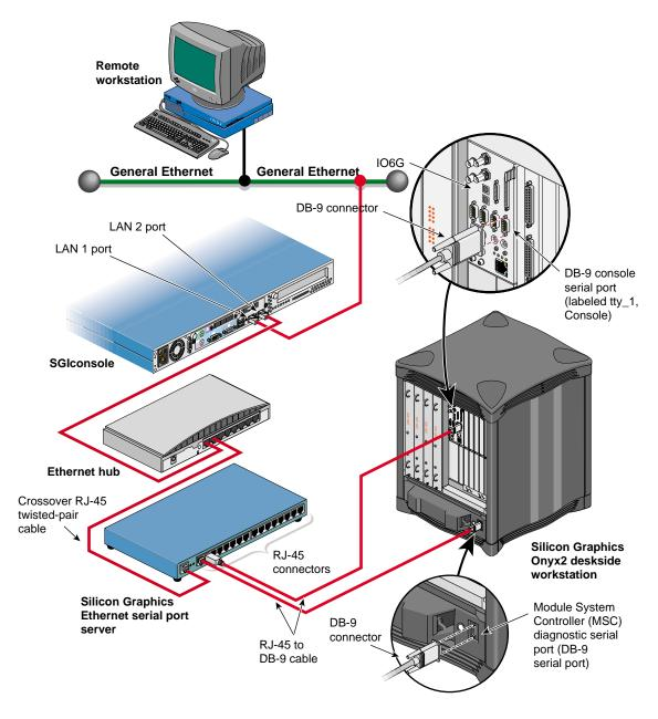
Figure 5-27 Connecting a Silicon Graphics Onyx2 Deskside Workstation to an SGIconsole
