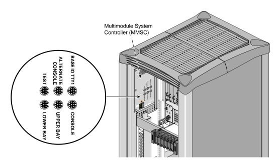
Figure B-22 shows the MMSC 8-pin mini-DIN connectors of the Silicon Graphics Onyx2 rackmount graphics system.
