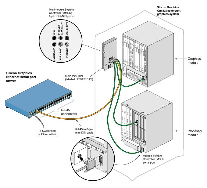
Figure 5-36 Connecting the MMSC Lower Bay Connector to the Processor Module MSC Serial Port
