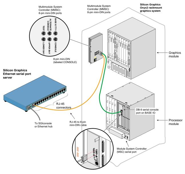
Figure 5-34 Connecting the MMSC Base I/O TTY1 to the Processor Module tty\_1, Console Connector
