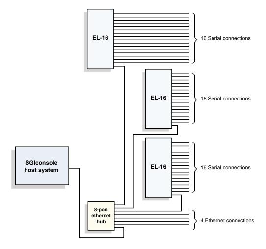
Figure 2-12 Sample Cabling Configuration: One Ethernet Hub, Three Serial Port Servers
