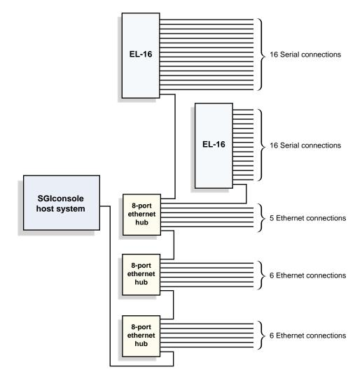
Figure 2-11 Sample Cabling Configuration: Three Ethernet Hubs, Two Serial Port Servers
