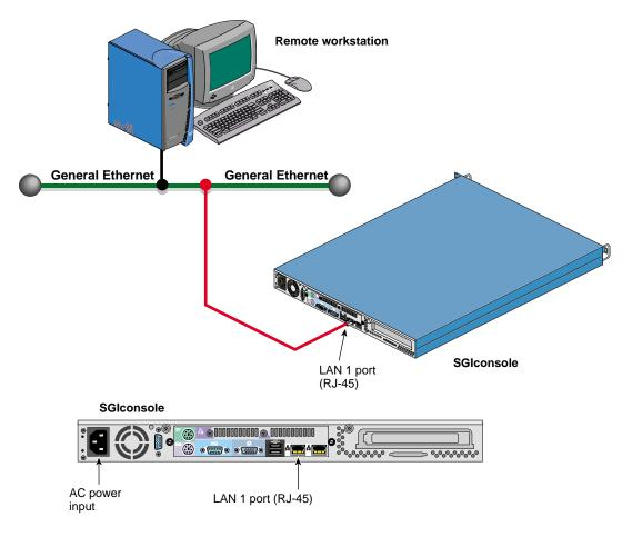
Figure 3-2 Example Connection of Remote Workstation to SGIconsole
