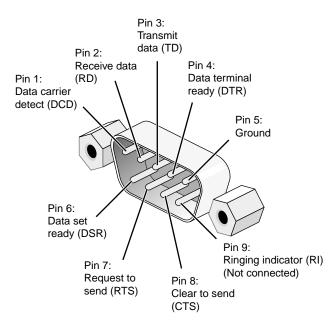
Figure B-10 SGI Altix 350, Origin and Onyx 300 and 350 DB-9 Serial Port Connector Pin Assignments
