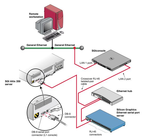
Figure 5-11 Connecting an SGI Altix 350 Server to a (Dell D600 Laptop) SGIconsole
