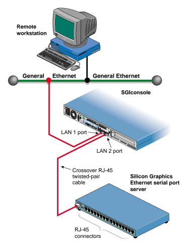
Figure 3-8 Connecting a Serial Port Server to an SGIconsole Host System with no Ethernet Hub
