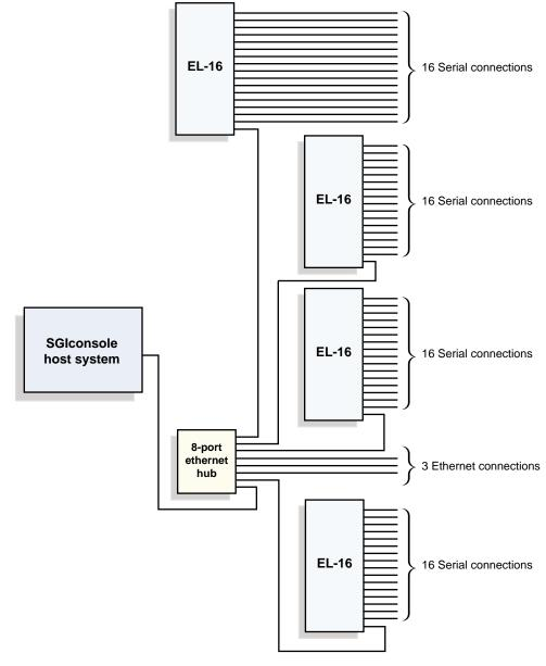
Figure 2-15 Sample Cabling Configuration: One Ethernet Hub, Four Serial Port Servers
