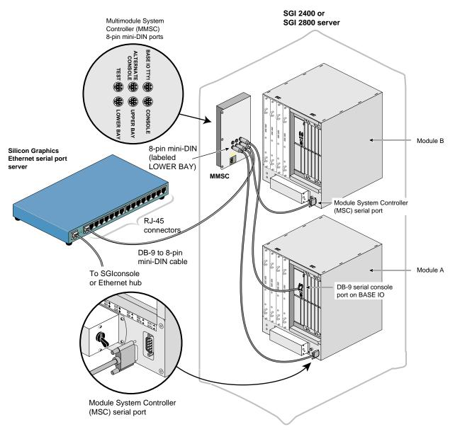
Figure 5-23 Connecting the MMSC Lower Bay Connector to the Module A MSC Serial Port
