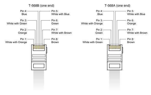
Figure B-8 Typical Color Codes for a Crossover RJ-45 Ethernet Cable
