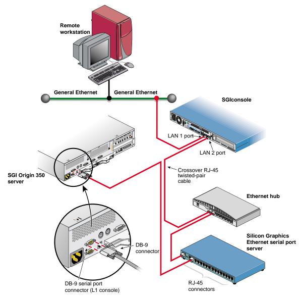
Figure 5-8 Connecting an SGI Origin 350 Server to an (SGI 1100) SGIconsole
