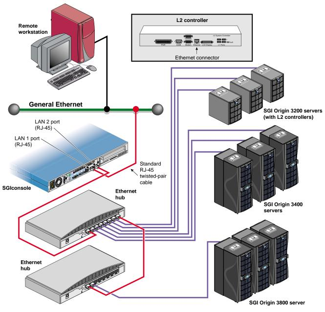
Figure 4-4 Connecting SGI Origin 3000 Series Servers with L2 Controllers to SGIconsole
