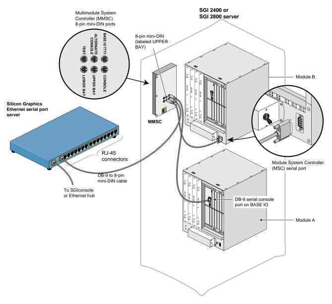
Figure 5-22 Connecting the MMSC Upper Bay Connector to the Module B MSC Serial Port
