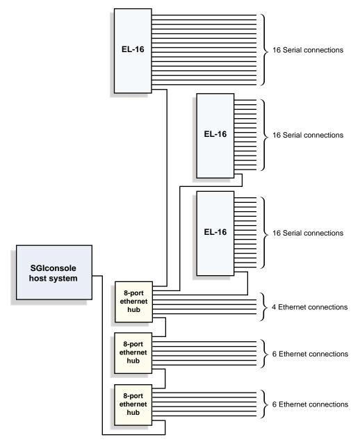
Figure 2-14 Sample Cabling Configuration: Three Ethernet Hubs, Three Serial Port Servers
