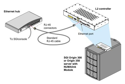
Figure 4-3 Connecting an Origin 300 or Origin 350 Server with NUMAlink Module L2 Controller to an Ethernet Hub
