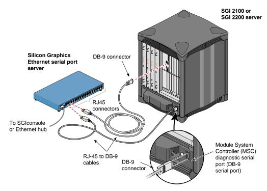
Figure 5-17 Connecting the SGI 2100 or SGI 2200 Server MSC Serial Port to the Serial Port Server
