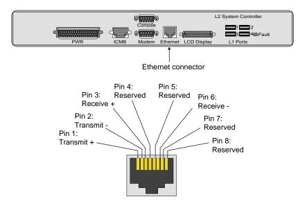
Figure B-18 shows the pin number locations and pin assignments for the Ethernet connector on the L2 controller hardware available for the SGI Origin and Altix 3000 series servers.
