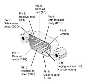
Figure B-17 SGI Origin and Altix 3000 Series C-brick DB-9 Serial Port Connector Pin Assignments
