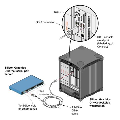
Figure 5-29 Connecting the tty\_1, Console Connector to the Serial Port Server
