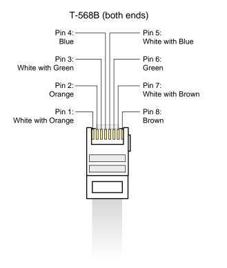
Figure B-7 Typical Color Codes for a Standard RJ-45 Ethernet Cable
