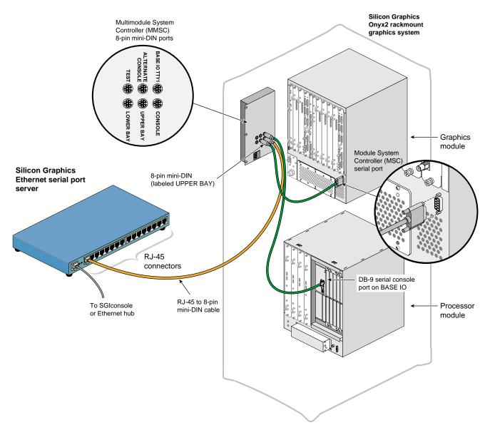
Figure 5-35 Connecting the MMSC Upper Bay Connector to the Graphics Module MSC Serial Port
