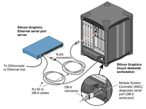
Figure 5-30 Connecting the MSC Serial Port Connector to the Serial Port Server
