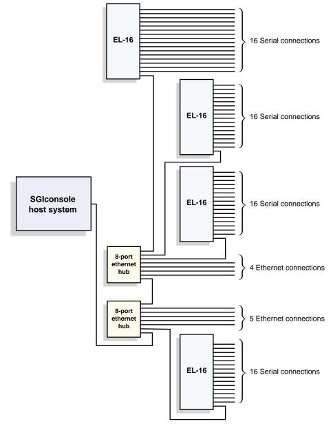
Figure 2-16 Sample Cabling Configuration: Two Ethernet Hubs, Four Serial Port Servers
