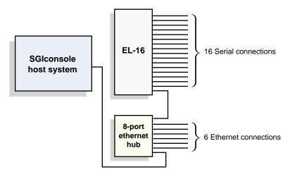
Figure 2-6 Sample Cabling Configuration: One Ethernet Hub, One Serial Port Server
