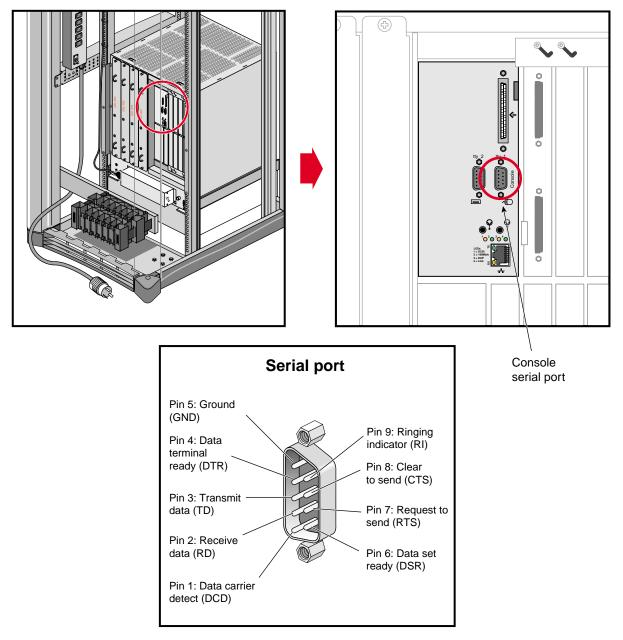
Figure B-13 SGI 2400 and SGI 2800 Server Serial Port Pin Location and Assignments
