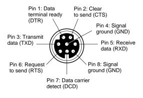
Figure B-16 MMSC 8-pin Mini-DIN Connector Pin Assignments
