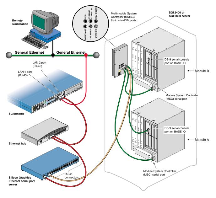
Figure 5-18 Connecting an SGI 2400 or SGI 2800 Server to an SGIconsole (SGI 1100 Shown)
