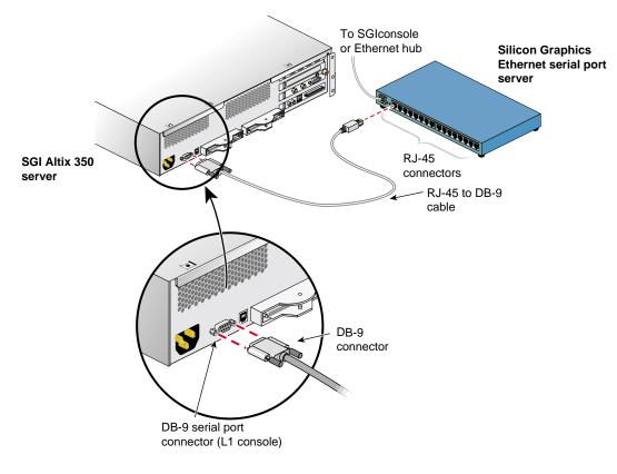
Figure 5-13 Connecting the Altix 350 Server Serial Port Connector to the Serial Port Server
