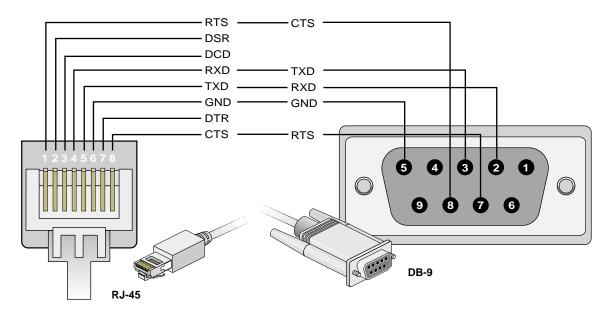
Figure B-3 RJ-45 to DB-9 Serial Cable With Flow Control Pin Assignments
