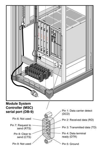
Figure B-21 shows the pin locations and assignments for the module system controller (MSC) of the Silicon Graphics Onyx2 rackmount graphics system.
