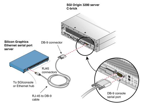
Figure 5-26 Connecting the SGI Origin 3200 Server Console Port to the Serial Port Server
