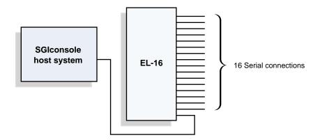
Figure 2-5 Sample Cabling Configuration: No Ethernet Hub, One Serial Port Server
