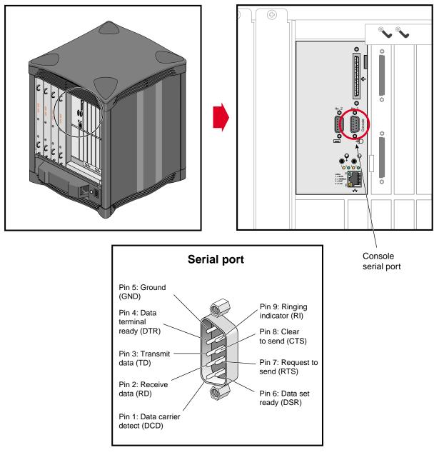
Figure B-12 SGI 2100 and SGI 2200 Server Serial Port Pin Location and Assignments
