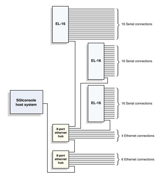
Figure 2-13 Sample Cabling Configuration: Two Ethernet Hubs, Three Serial Port Servers
