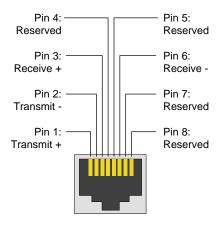
Figure B-6 RJ-45 Ethernet Jack Pin Assignments
