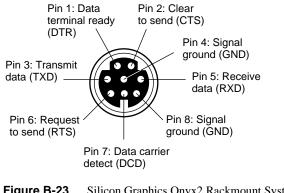
Figure B-23 shows the pin number locations and pin assignments for the MMSC 8-pin mini-DIN connectors of the Silicon Graphics Onyx2 rackmount graphics system.
