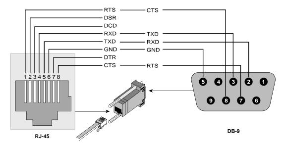
Figure B-4 RJ-45 to DB-9 Serial Adapter With Flow Control Pin Assignments
