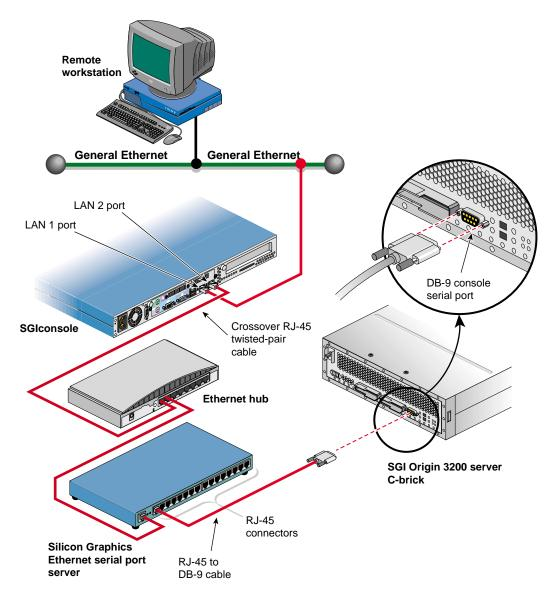
Figure 5-24 Connecting an SGI Origin 3200 Server Without an L2 Controller to an SGI console
