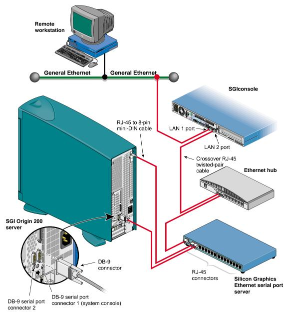
Figure 5-1 Connecting an SGI Origin 200 Server to an SGIconsole (SGI 1100 Shown)
