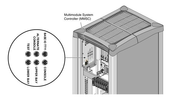
Figure B-15 shows the MMSC 8-pin mini-DIN connectors.
