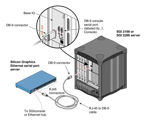
Figure 5-16 Connecting the SGI 2100 or SGI 2200 tty\_1, Console Connector to the Serial Port Server
