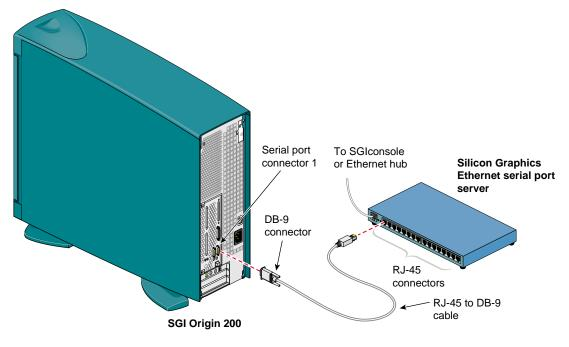
Figure 5-3 Connecting the SGI Origin 200 Server Serial Port Connector to the Serial Port Server
