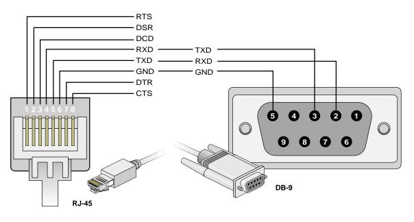
Figure B-1 RJ-45 to DB-9 Serial Cable Pin Assignments
