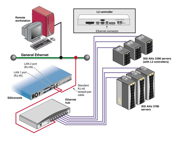
Figure 4-7 Connecting SGI Altix 3000 Series Servers (With L2) to an SGIconsole
