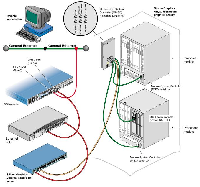
Figure 5-31 Connecting a Silicon Graphics Onyx2 Rackmount System to an SGIconsole
