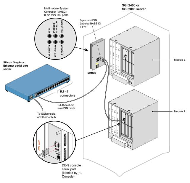
Figure 5-21 Connecting the MMSC Base I/O TTY1 to the Module A tty\_1, Console Connector
