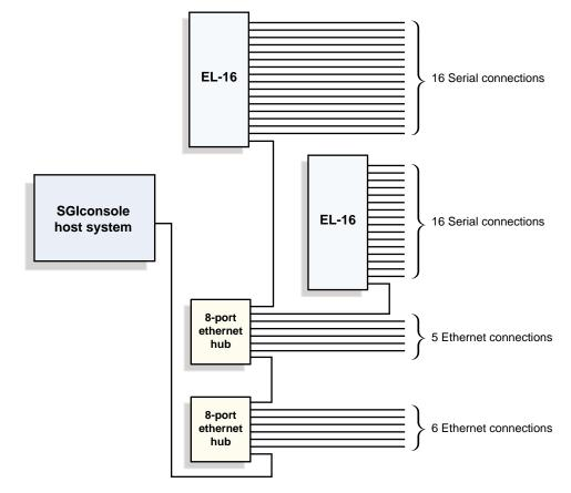
Figure 2-10 Sample Cabling Configuration: Two Ethernet Hubs, Two Serial Port Servers
