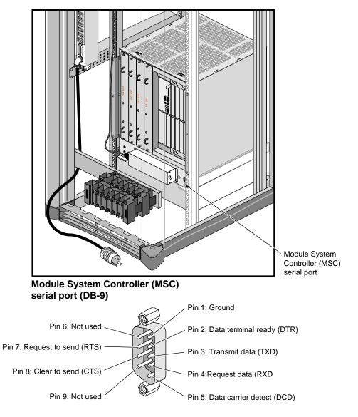
Figure B-14 shows the pin locations and assignments for the Module System Controller (MSC) serial port (DB-9 connector).
