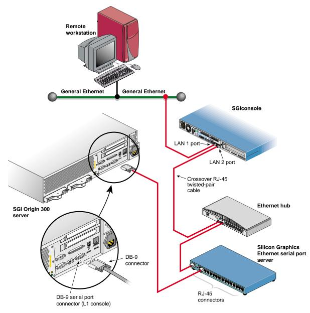
Figure 5-5 Connecting an SGI Origin 300 Server to an SGIconsole (SGI 1100 shown)
