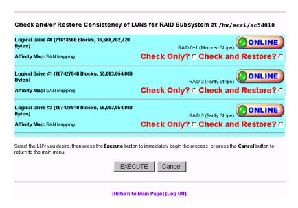
Figure 3-37 Data Consistency Check/Restore
