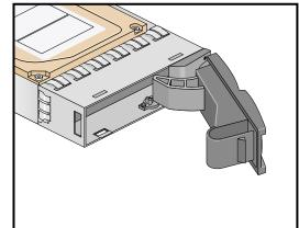
5. Release the handle of the replacement carrier by pressing the latch in the handle towards the right, as shown in Figure 3-5. Insert the carrier into the enclosure.
