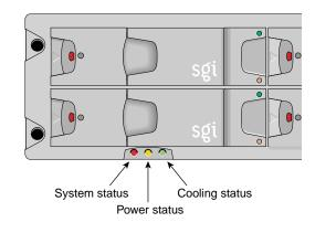
Figure 4-1ESI/Ops Panel LEDs
