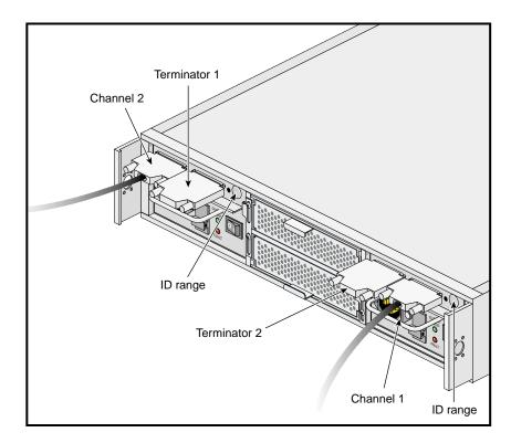
**Figure 2-2** Attaching Interface Cable on 2 x 4 Configuration
