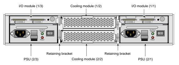
Figure 1-17 Rear Module Locations and Bay Numbering
