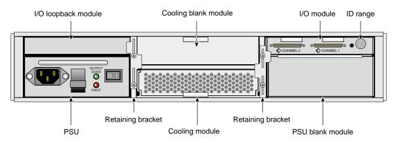
Figure 1-2Rear Module Location in Standard Configuration
