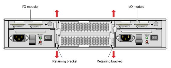
Figure 3-4 I/O Module Retaining Bracket
