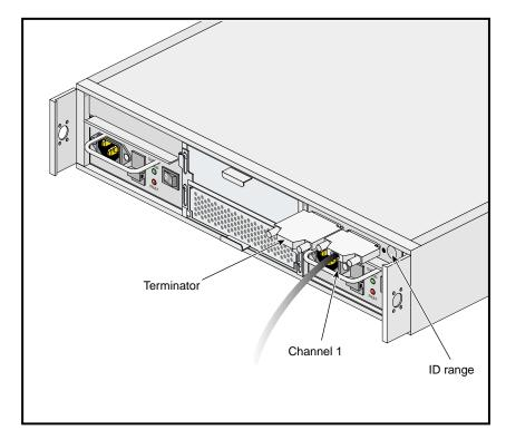
Figure 2-1Attaching Interface Cable on 1 x 8 Configuration
