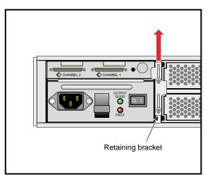
Figure 3-1 Power Supply Module Retaining Bracket
