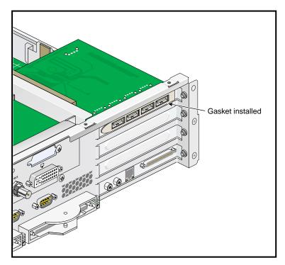
Figure 2 Attaching Gasket to USB Card Bulkhead
