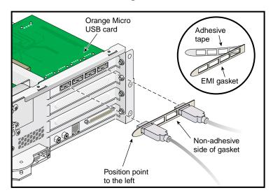
Figure 1 Inserting Two Type A USB Connectors
