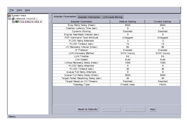
Figure 8-5 Example: After Clicking the HBA Icon to Show the Adapter Parameters
