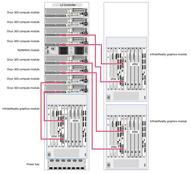
Figure 3-11 illustrates a six-pipe Onyx 300 graphics system with NUMAlink module.
