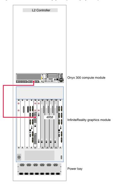
Figure 3-1 illustrates a one-pipe Onyx 300 graphics system without NUMAlink module.
