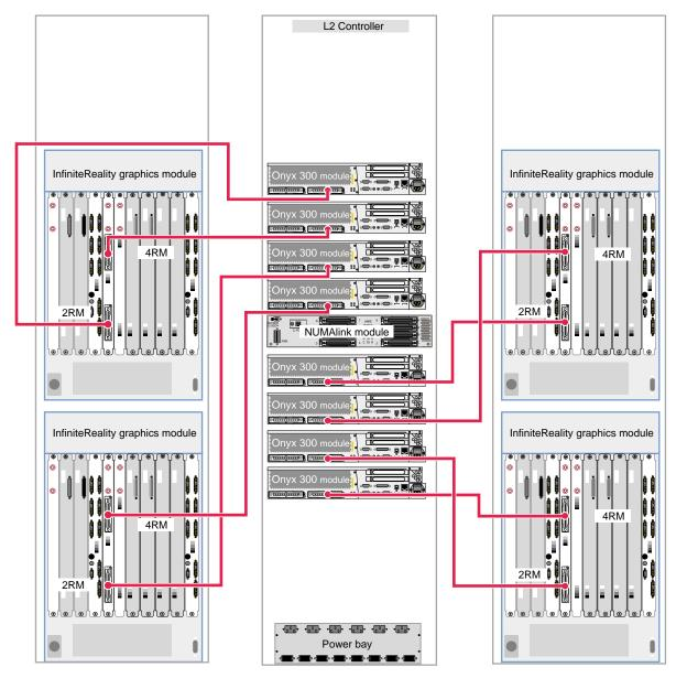
Figure 3-13 Eight-pipe Graphics System (Four 4-RM and Four 2-RM Pipes)
