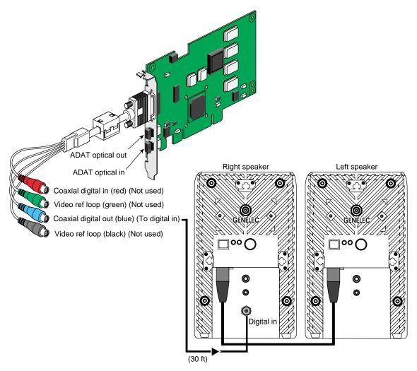
Figure 2-5 Connecting the Audio PCI Card to Speakers
