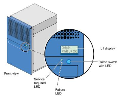
Figure 1-13 L1 Controller Display, Switch, and LEDs
