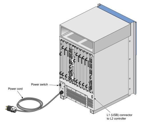
3. Set the power switch of the InfiniteReality graphics module to the On position. Figure 2-17 shows the location of the power switch.
