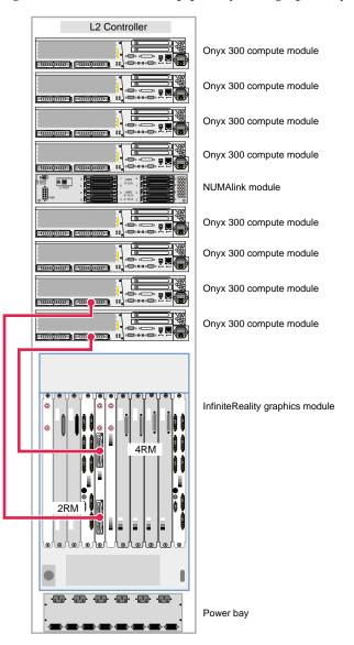
Figure 3-8 illustrates a two-pipe Onyx 300 graphics system with NUMAlink module.
