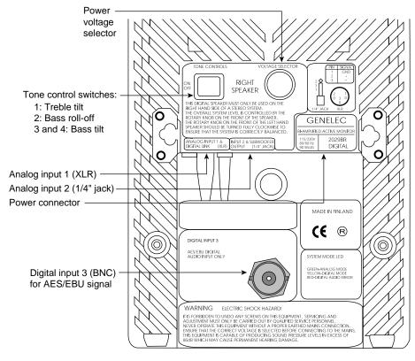
Figure 2-6 shows the location of the controls and connectors on the back of the right speaker.
