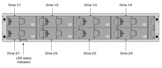
Figure 1-33 Front View of TP900 Storage Module
