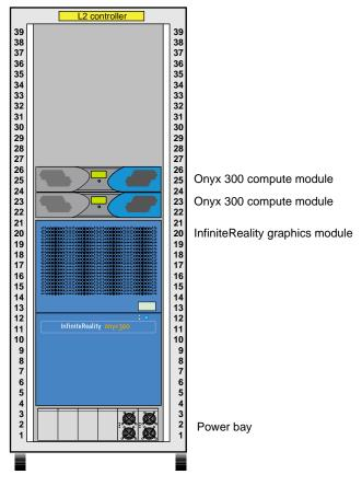
Figure 1-18 Unit Numbering within Rack
