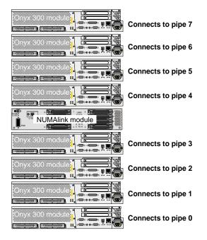
Figure 3-6 Pipe Connections
