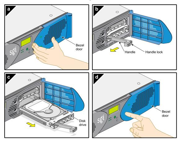
Figure 2-24 Removing a Disk Drive
