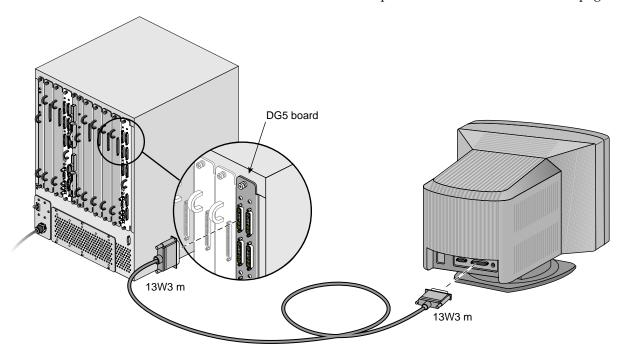
Figure 2-1 Monitor-to-DG5 Connection
