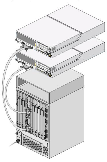
In both configurations, the InfiniteReality graphics module connects to the XIO port of an Onyx 300 compute module as shown in Figure 1-2.
