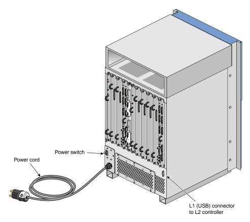
Figure 2-20 InfiniteReality Graphics Module Power Switch
