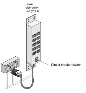
Figure 2-16 PDU Circuit Breaker Switch
