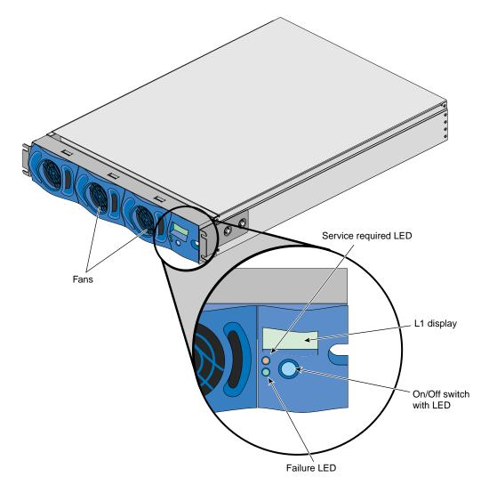
Figure 1-26 Front View of NUMAlink Module
