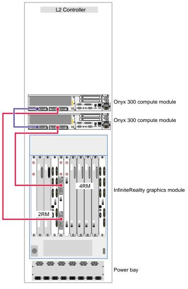
Figure 3-2 illustrates a two-pipe Onyx 300 graphics system without NUMAlink module.
