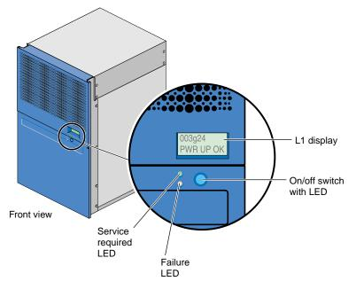
Figure 1-6 Front Components
