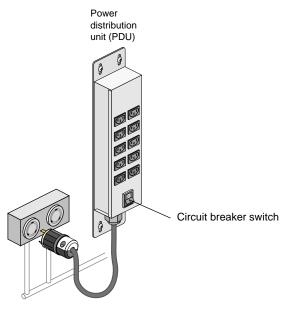
Figure 2-19 PDU Circuit Breaker Switch
