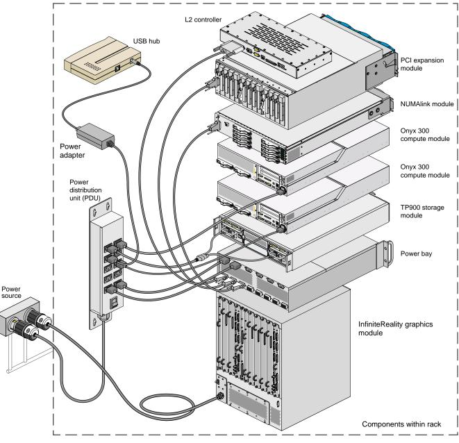
Figure 2-10 PDU and Power Connections
