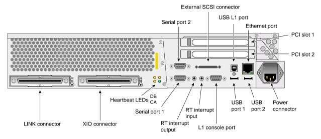
Figure 1-17Rear I/O Ports and Features
