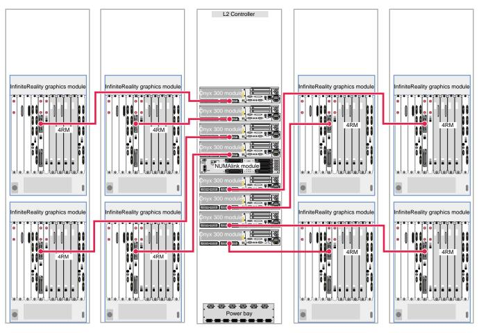
Figure 3-14 Eight-pipe Graphics System (Eight 4-RM Pipes)
