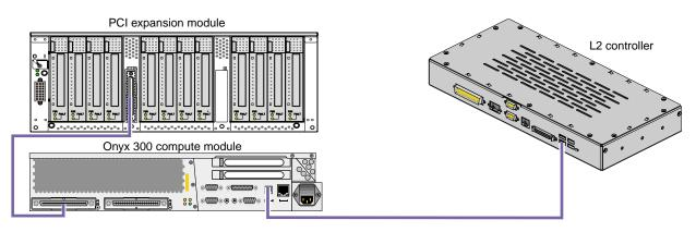
Figure 2-14 PCI Expansion Module Connection to L2 Controller
