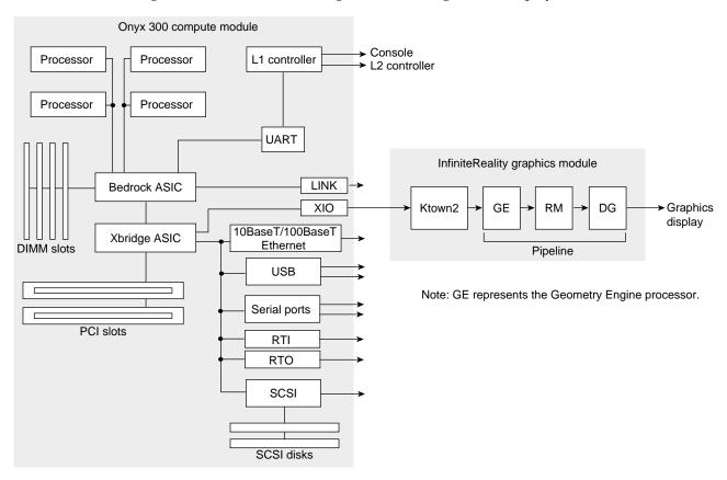
Figure 1-3 Onyx 300 Graphics System Block Diagram
