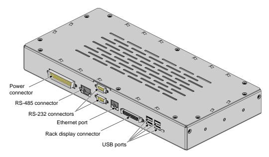
Figure 1-22 Front View of the L2 Controller
