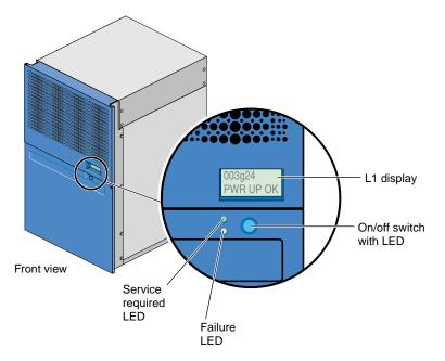
Figure 2-18 Front View of InfiniteReality Graphics Module
