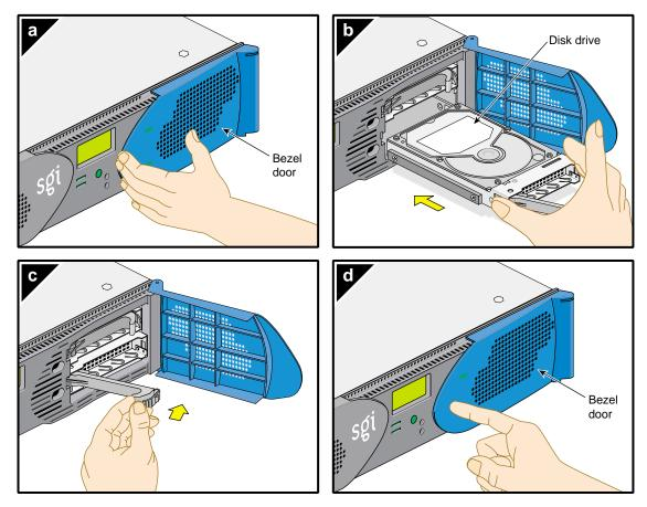
Figure 2-23Installing a Disk Drive
