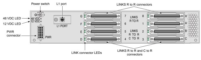
Figure 1-27 Rear View of NUMAlink Module
