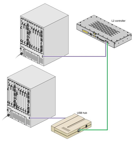
Figure 2-11 InfiniteReality Connections to L2 Controller
