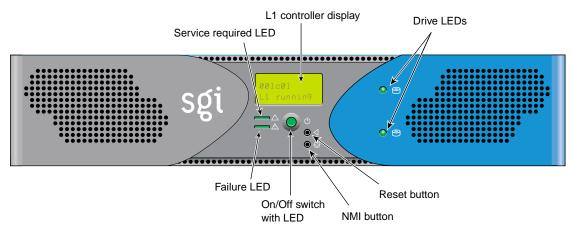
Figure 1-16 Front Controls and Indicators
