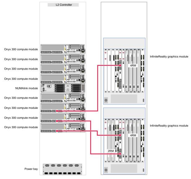
Figure 3-9 illustrates a three-pipe Onyx 300 graphics system with NUMAlink module.
