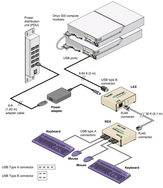
Figure 2-3 Keyboard and Mouse Connections via USB Extender
