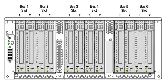
Figure 1-29 shows the PCI card slot numbering on the PCI expansion module.
