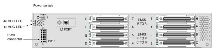
Figure 2-15 NUMAlink Module Power Switch
