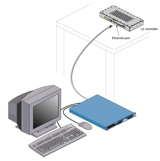
To attach a system console that runs the SGIconsole software to your system, connect the system console to the L2 controller Ethernet port connector as shown in Figure 2-8.
