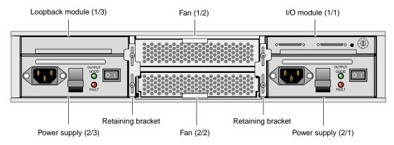
Figure 1-34 Rear View of TP900 Storage Module
