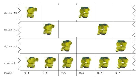
Figure 9 illustrates frame multiplexing on a four-pipe system.
