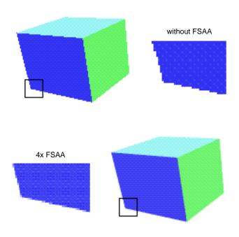
Figure 11 illustrates the advantage of using a 4x FSAA solution.
