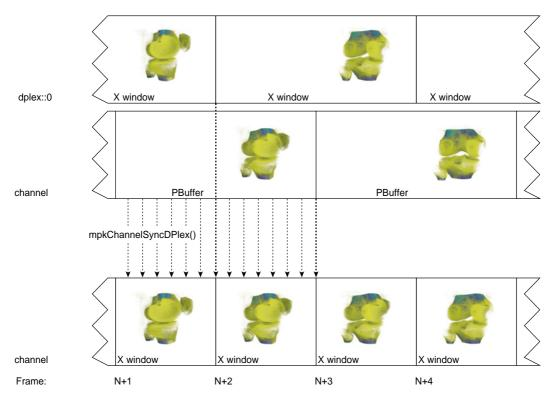
**Figure 3-14** Two-Pipe Full-Scale DPLEX Compound
