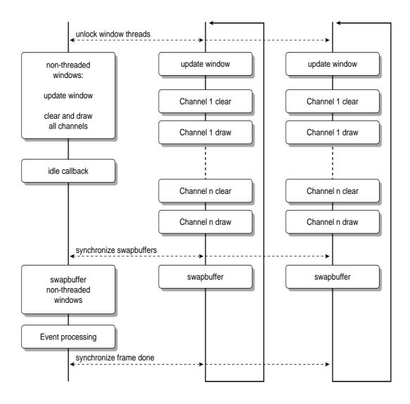
Figure 2-4 A Simplified mpkConfigFrame() Call
