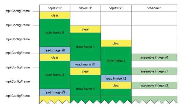
**Figure 3-13** The Execution of a DPLEX ASYNC Compound
