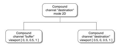
**Figure 4-1** Compound Tree for a 2D Decomposition
