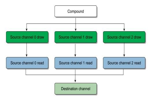
Figure 3-1 Source and Destination Channels
