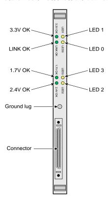
Figure 2 Front-panel Items of the VME Interface Board
