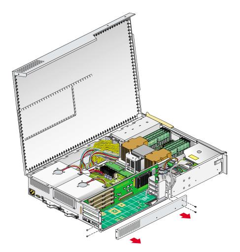
**Figure 6-12** Removing the Lower PCI/PCI-X Support Bracket
