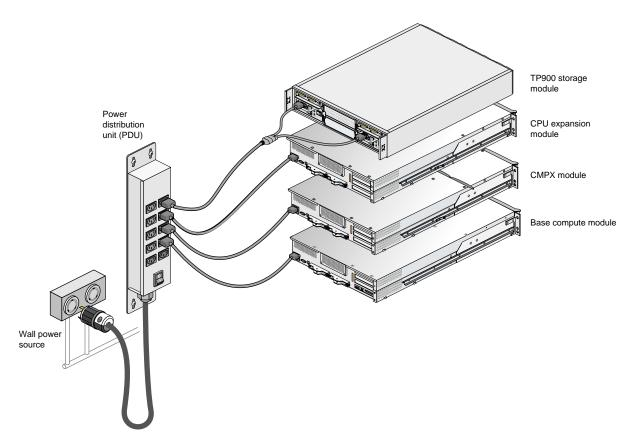
Figure 2-18 Power Connection Example for Altix 350 System
