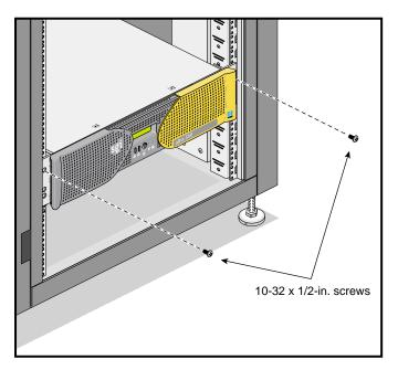
**Figure 1-20** Securing the Module to the Rack
