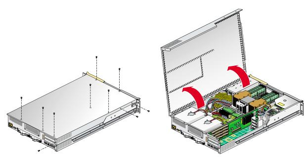
Figure 6-27 Opening Module to Remove DIMM
