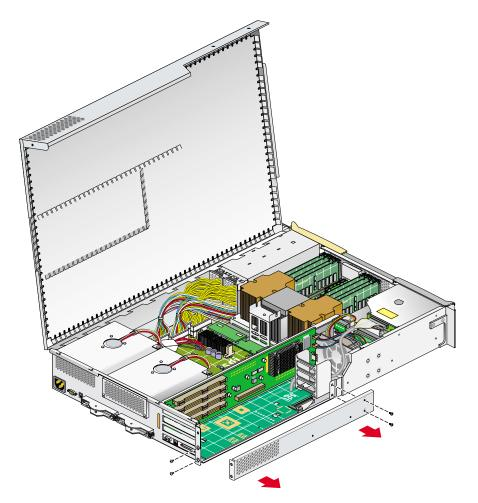
Figure 6-5 Removing the Lower PCI/PCI-X Support Bracket
