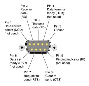
**Figure A-5** DB-9 Connector Pin Assignments
