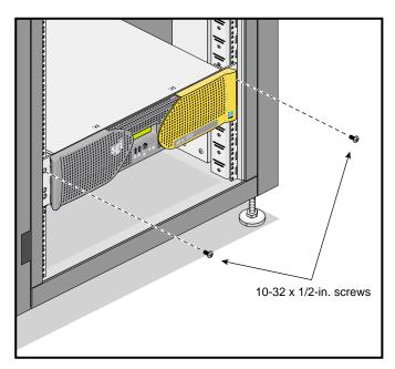
**Figure 1-24** Securing the Module to the Rack
