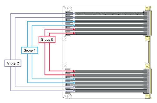
Figure 6-24 Layout of Slots and DIMM Memory Groups
