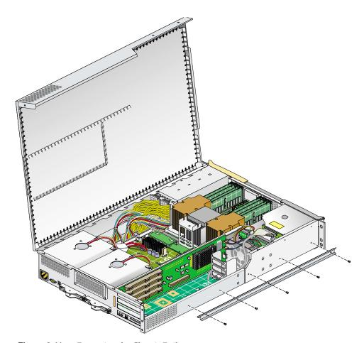
Figure 6-11 Removing the Chassis Rail
