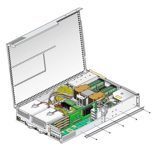
Figure 6-16 Replacing the Optional Chassis Rail
