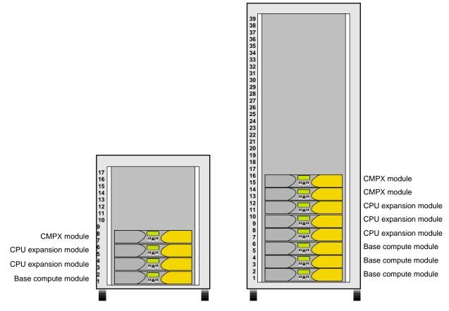
Figure 2-19 Unit Numbering Within Racks
