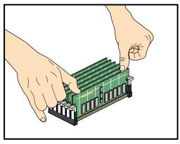
Figure 6-26 Inserting a DIMM
