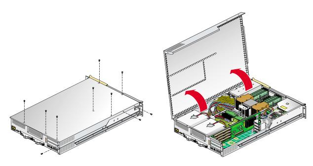
Figure 6-25 Opening Module Cover to Install DIMMs
