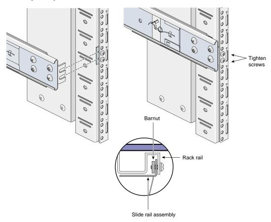
Figure 1-17 Attaching the Slide Rail to the Rack
