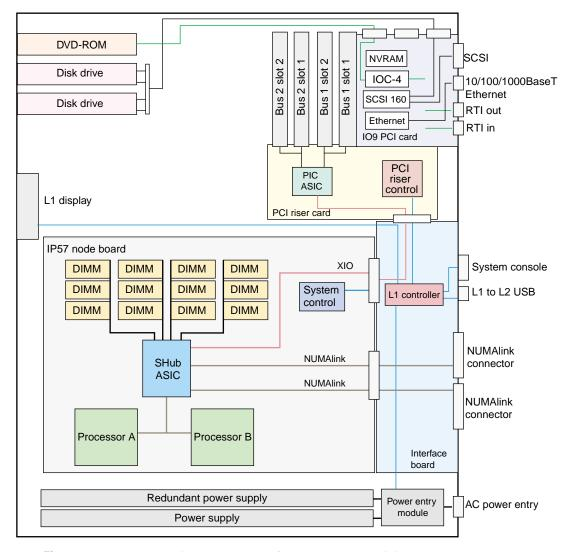
Figure 3-2 Functional Logic Diagram of Base Compute Module
