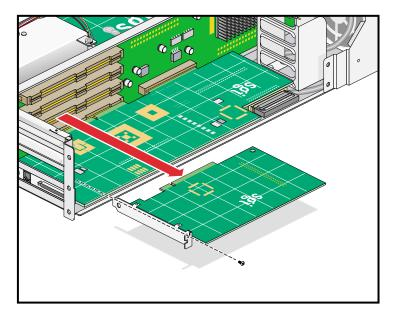
Figure 6-13 Removing the Retaining Screw and Extracting the Card
