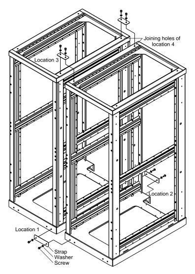
Figure 1-10 Joining Locations
