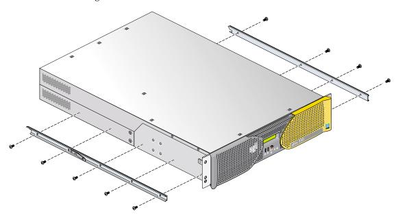
Figure 1-14 Attaching Chassis Rails to the Module Chassis
