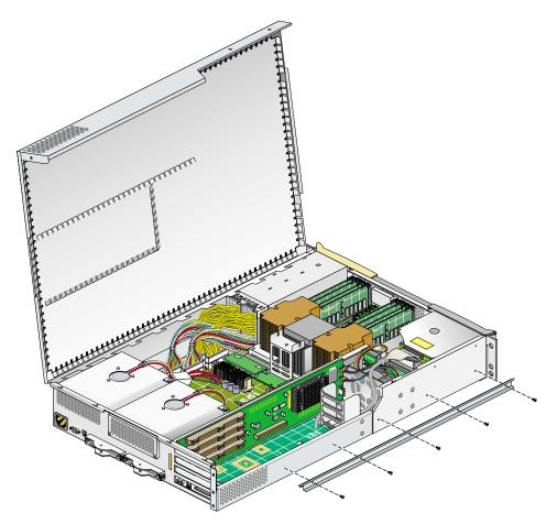
Figure 6-4 Removing an Optional Chassis Rail
