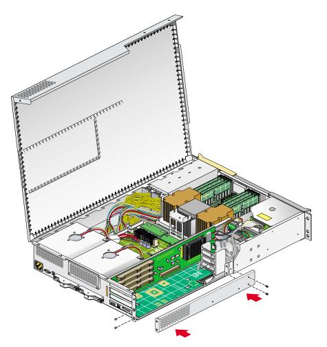
**Figure 6-8** Replacing the Lower PCI/PCI-X Support Bracket
