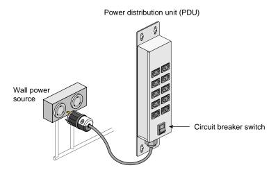
Figure 1-31 PDU Circuit Breaker
