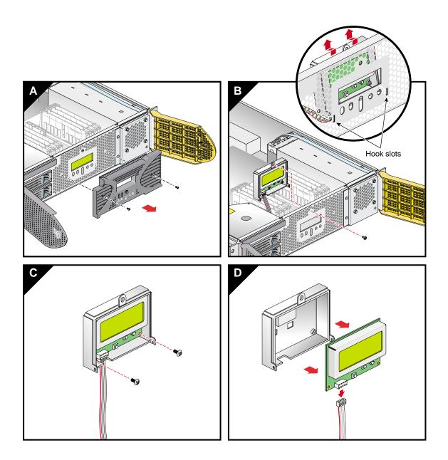
Figure 6-31 Removing the L1 Controller Display Panel
