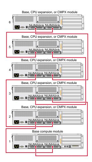
Figure 2-8 Six Module Ring Topology
