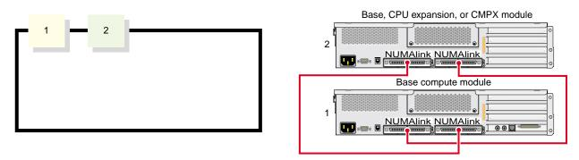
Figure 2-4 Two Module Ring Topology
