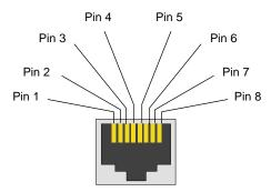
Figure A-6 RJ-45 Connector Pin Assignments
