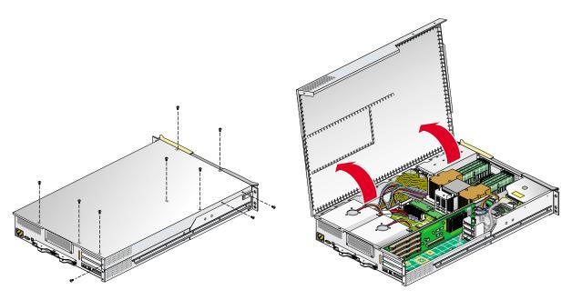
**Figure 6-30** Opening the Module to Access the L1 Controller Display
