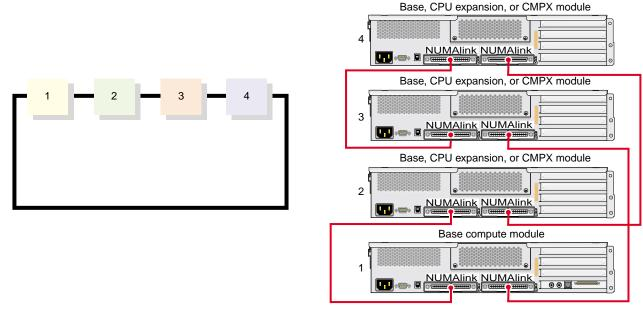
Figure 2-6 Four Module Ring Topology
