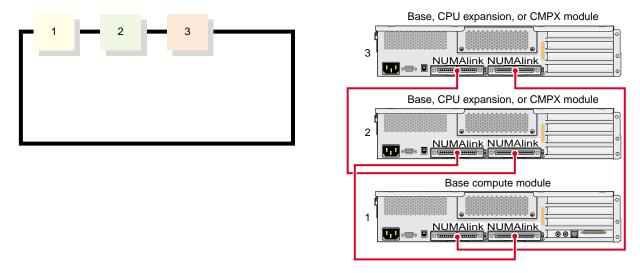
**Figure 2-5** Three Module Ring Topology
