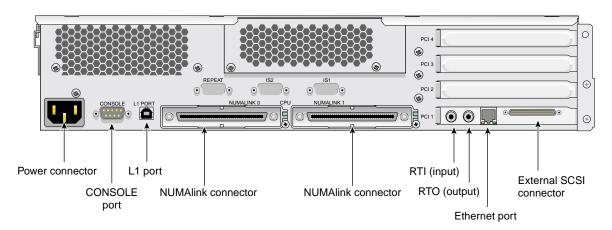
Figure A-1 Rear Panel of Compute Module
