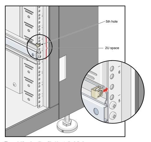
Figure 1-18 Installing Clip Nuts in Rack Rails
