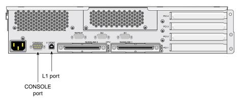
Figure A-2 Non-Proprietary Connectors on Rear Panel of CMPX Module
