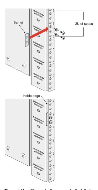
**Figure 1-16** Placing the Barnuts on the Rack Rails
