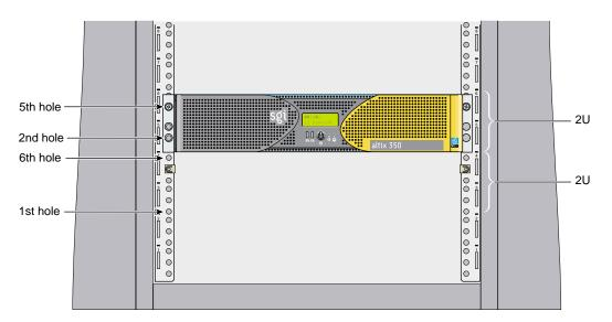
**Figure 1-15** Mounting Hole Pattern of Rack Vertical Rails
