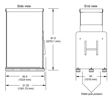
**Figure 1-3** Dimensions of Tall Rack Shipping Crate
