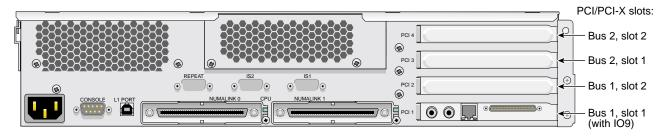
**Figure 6-3** PCI and PCI-X Card Slots in the Base Compute Module
