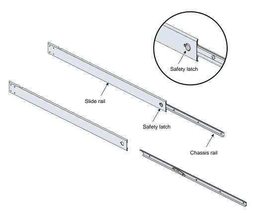
**Figure 1-12** Removing the Chassis Rail from the Slide Rail
