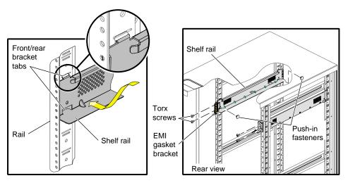
**Figure 1-23** Installing the Shelf Rails in the Rack
