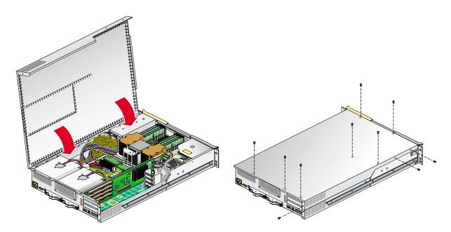
Figure 6-17 Close and Screw Down Cover
