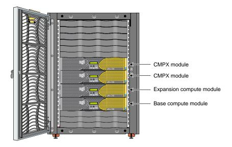
**Figure 5-6** System with CMPX Modules, Expansion Compute Module, and a Base Compute Module
