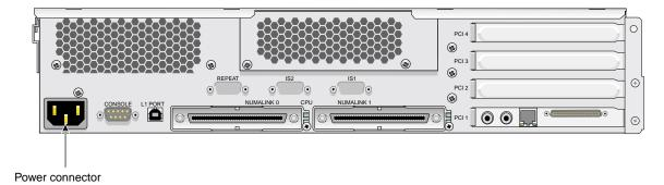
**Figure 1-27** Power Connector on the Rear of the Base Compute Module
