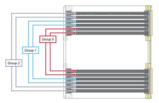
Figure 3-5 DIMM Group Locations on the Processor Board
