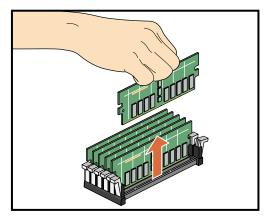
Figure 6-28 Removing a DIMM
