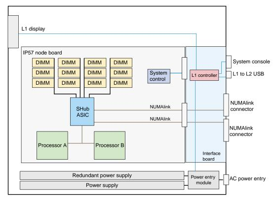
Figure 4-2 Functional Block Diagram of CPU Expansion Module
