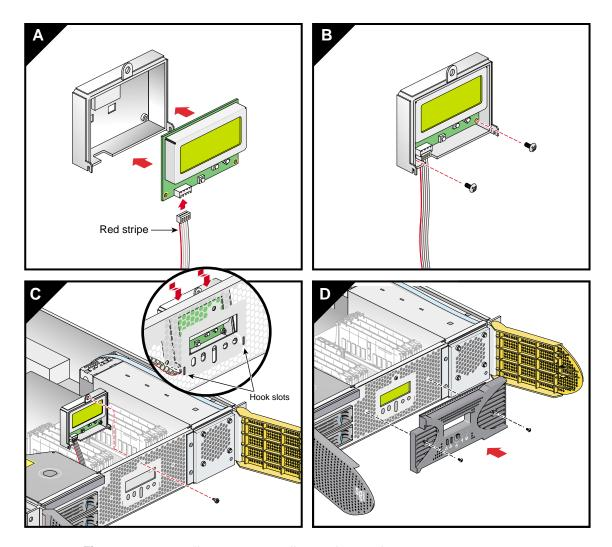
Figure 6-32 Installing an L1 Controller Display Panel
