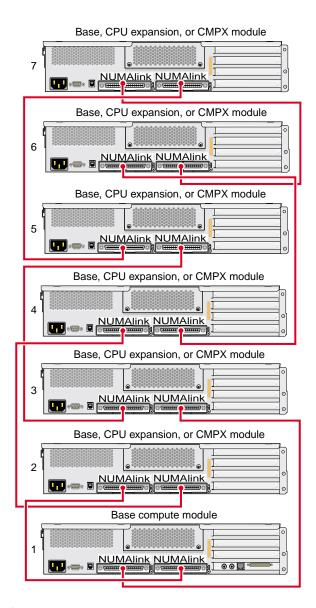
Figure 2-9 Seven Module Ring Topology
