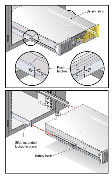
**Figure 1-21** Releasing the Safety Latches
