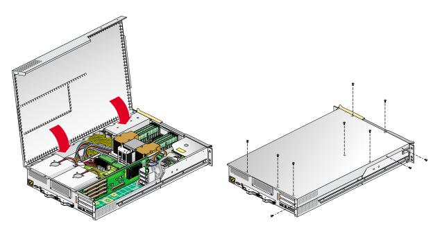
Figure 6-2 Closing the System Cover
