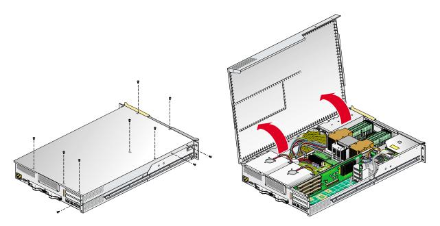
**Figure 6-10** Opening the Cover to Remove the Card
