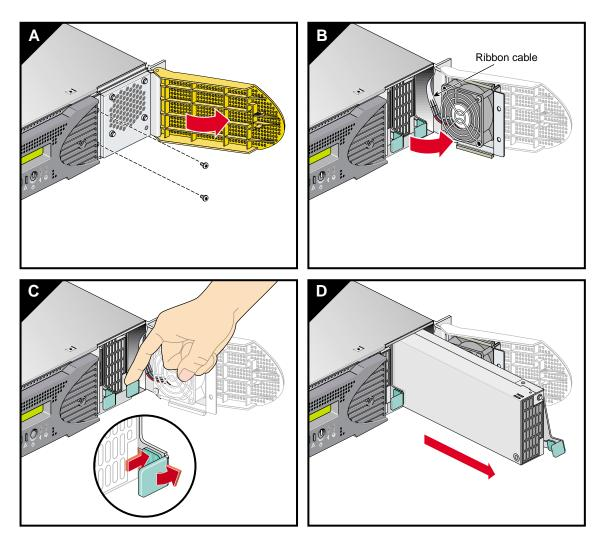
**Figure 6-22** Removing a Power Supply
