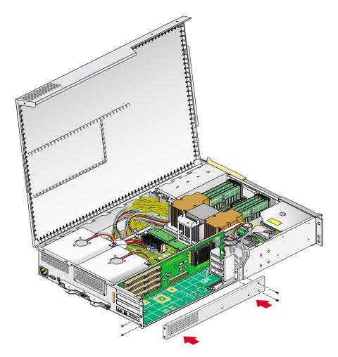
**Figure 6-15** Replacing the Lower PCI/PCI-X Support Bracket
