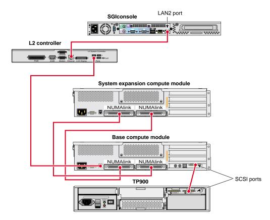
**Figure 1-26** Cabling Multiple Modules Example
