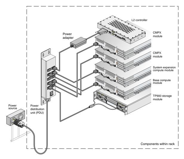
**Figure 1-29** Connecting Multiple Modules to a Power Source
