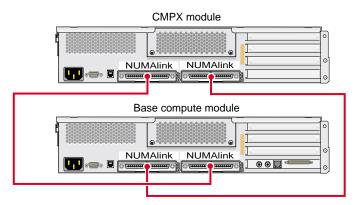
**Figure 1-25** Cabling a Base Compute Module to a CMPX Module
