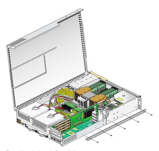
**Figure 6-9** Replacing the Chassis Rail
