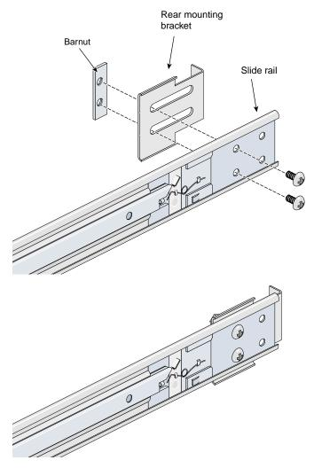
Figure 1-13 Attaching the Rear Mounting Bracket to the Slide Rail
