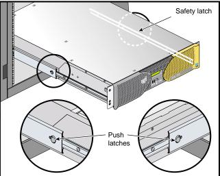
**Figure 1-19** Pressing the Safety Latches
