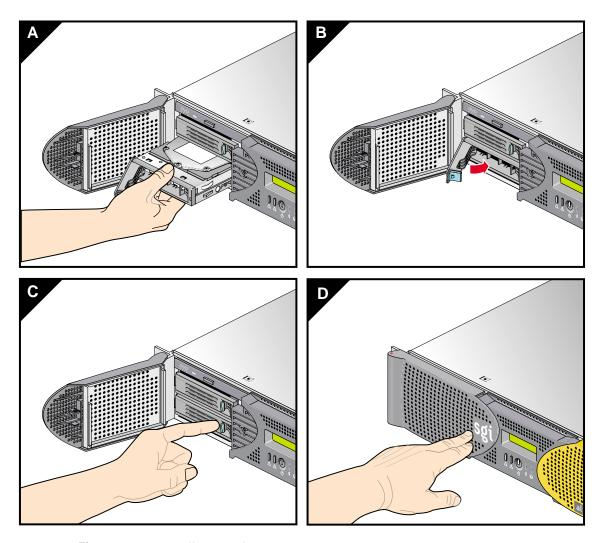
Figure 6-19 Installing a Disk Drive
