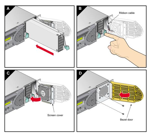
**Figure 6-23** Installing the power supply
