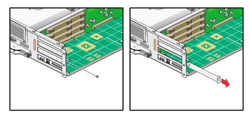
Figure 6-6 Removing the Blanking Plate
