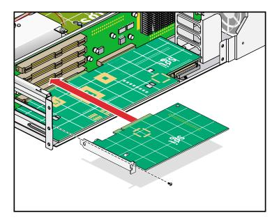
**Figure 6-7** Installing the Card and Retaining Screw
