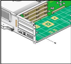
Figure 6-14 Replacing a Blanking Plate
