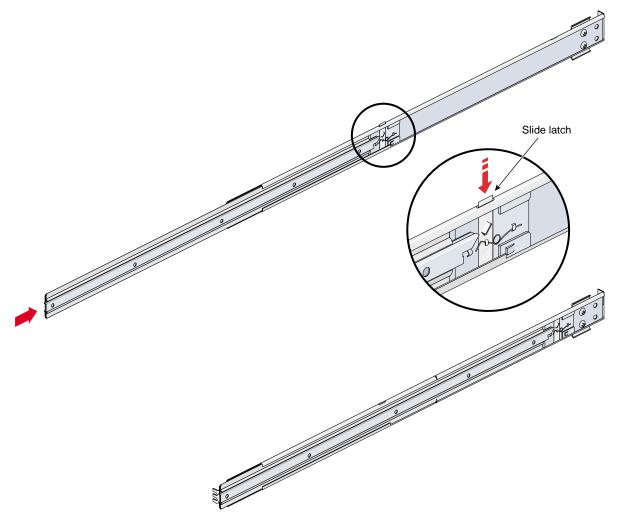
Figure 1-22 Releasing the Slide Latches
