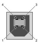
**Figure A-9** Pin Number Locations for USB Type B Connector
