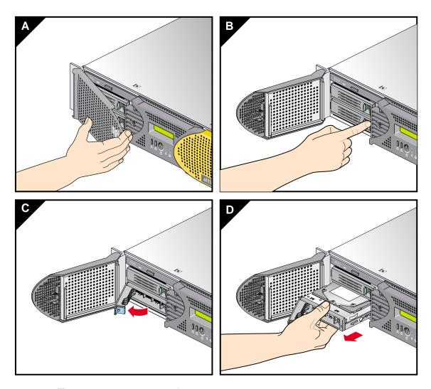
**Figure 6-20** Removing a Disk Drive
