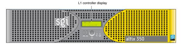
**Figure 6-29** L1 Controller Display on Base Compute Module
