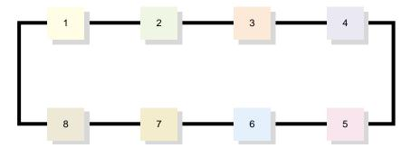
Figure 2-3 Ring Topology Connecting Eight Modules
