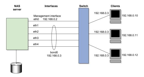
Figure 3-2 Aggregated (Bonded) Network Interfaces
