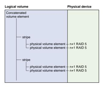
Figure A-1 Filesystem Structure
