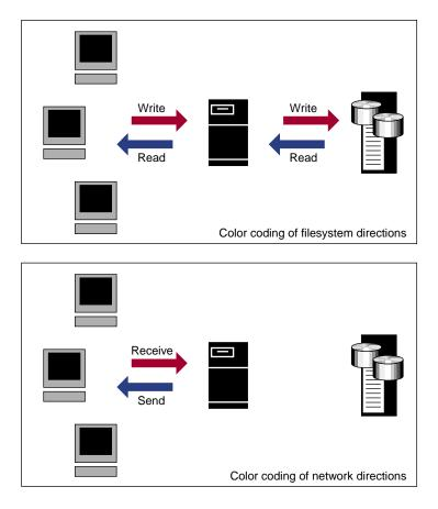
Figure 4-2 Color-Coding the Direction of Data Flow
