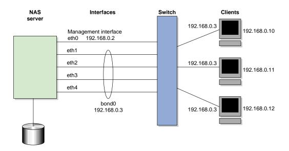
Figure 3-2 Aggregated (Bonded) Network Interfaces
