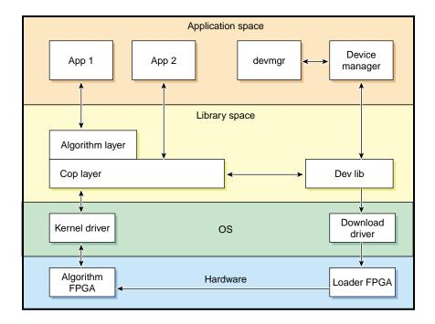
Figure 4-1 Abstraction Layer Software Block Diagram
