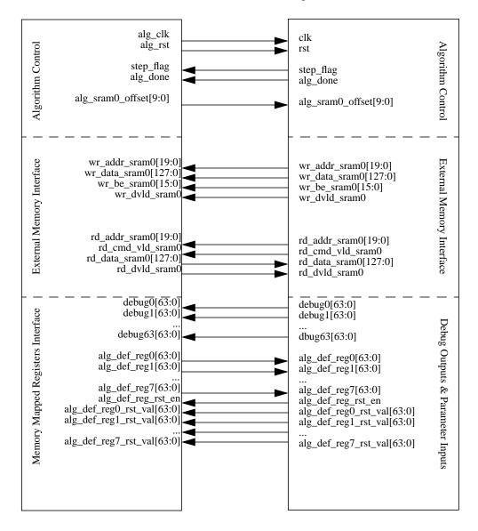
Figure 3-3 Algorithm / Core Services Interface Diagram
