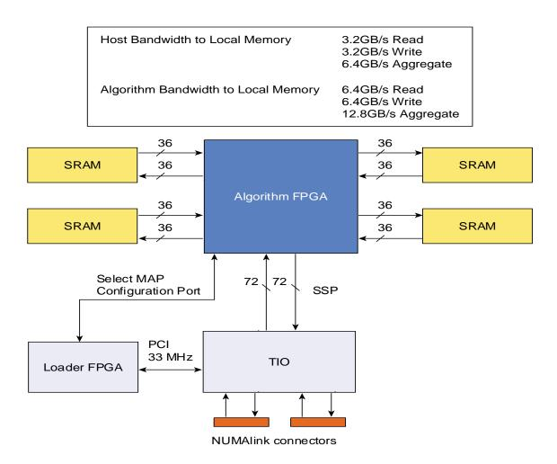
Figure 1-4 RASC FPGA Functional Block Diagram
