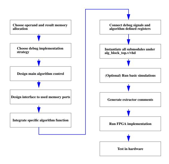
Figure 3-5 Hardware Accelerated Algorithm Design Flow
