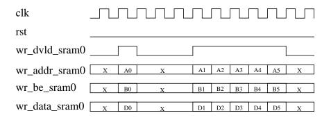
**Figure 3-8** Single, and Multiple Write Commands
