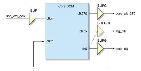
Figure 3-12 Core Clock and Algorithm Clock Source
