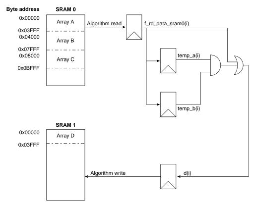
Figure 7-2 Simple Algorithm for Verilog and VHDL
