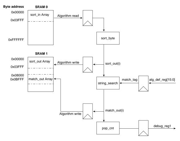
Figure 7-4 Data Flow Algorithm
