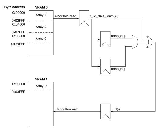
Figure 7-1 Simple Algorithm for Verilog
