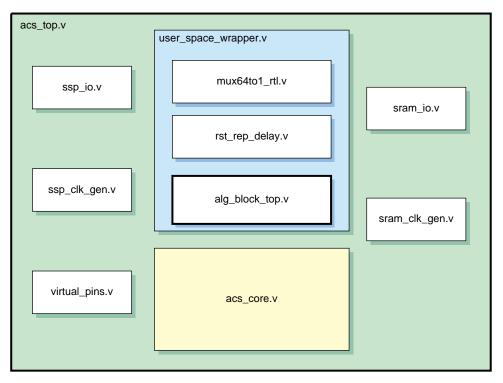
Figure 3-11 Instance Hierarchy of the RASC FPGA Design
