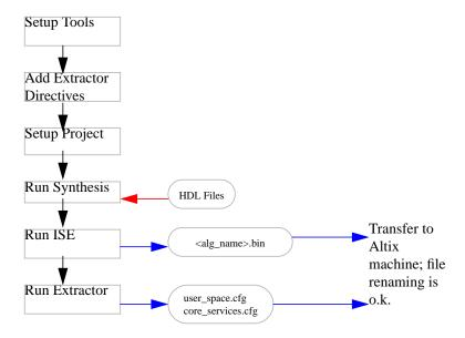
Figure 5-1 RASC FPGA Implementation Flow
