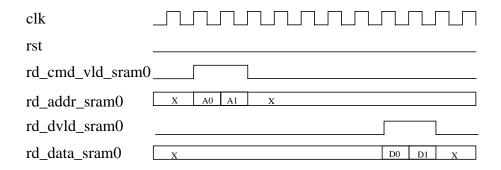
Figure 3-10 Multiple Read Transaction
