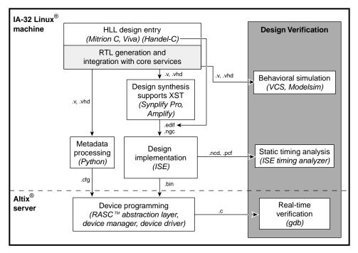
Figure 1-2 Bitstream Development with High-level Tools
