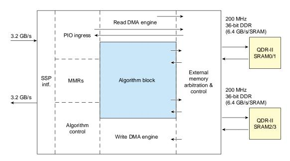
Figure 3-1 Block Diagram of the RASC Algorithm FPGA
