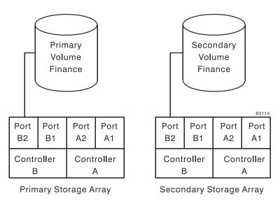
**Figure 3-7** Controller B as Controller Owner
