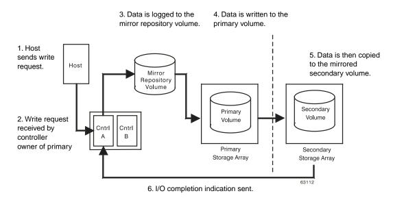
**Figure 3-3** Data Replication between Storage Arrays
