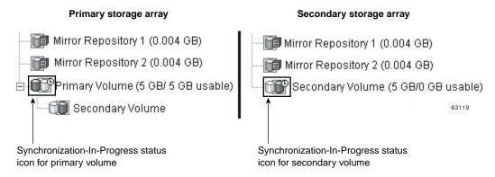
**Figure 3-5** Mirrored Volume Pair in Synchronization-in-Progress Status
