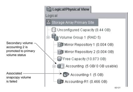
Figure 3-11 Snapcopy Volume Failure Because of Role Reversal
