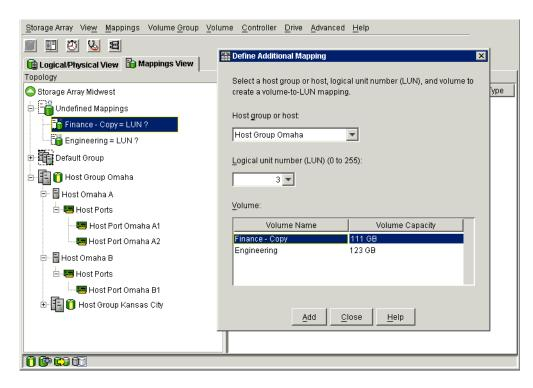
**Figure 4-25** Defining an Additional Volume-to-LUN Mapping for the Target Volume
