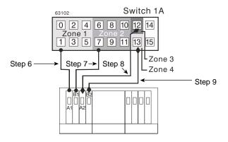
Figure 3-24 Storage Array Connections to Fibre Channel Switches
