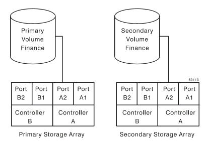
**Figure 3-6** Controller A as Controller Owner
