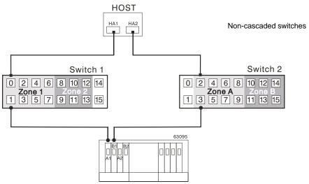
**Figure 3-15** Switch Zoning in Cascaded and Non-Cascaded Fibre Channel Switches
