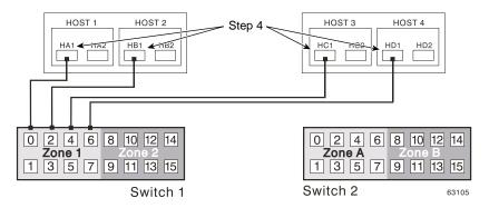
Figure 3-28 Primary Host Bus Adapter Connections to Fibre Channel Switches
