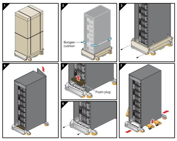
Figure 1-6 Removing a Tall Rack from the Shipping Crate
