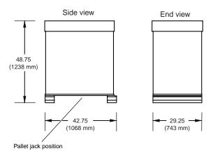
Figure 1-4 Dimensions of Short Rack Shipping Crate
