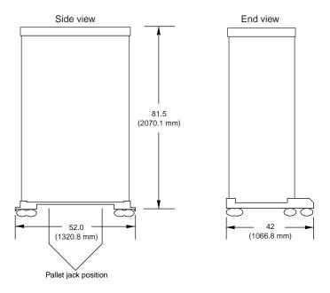
Figure 1-3 Dimensions of Tall Rack Shipping Crate
