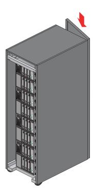
Figure 1-7 Reattaching the Tall Rack Door
