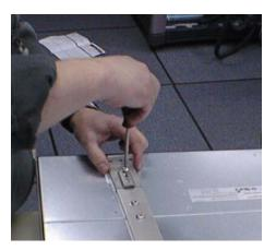
Figure 2-3 Attaching the Inner Bracket
