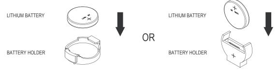
Figure E-1 Install the Battery
