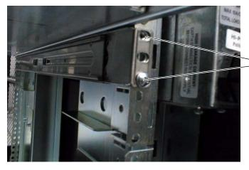
Slide two rail clips/nuts over the rack frame.
