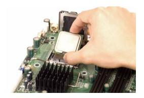
4. Align pin 1 of the CPU (the corner marked with a triangle) with the notched corner of the CPU socket.
