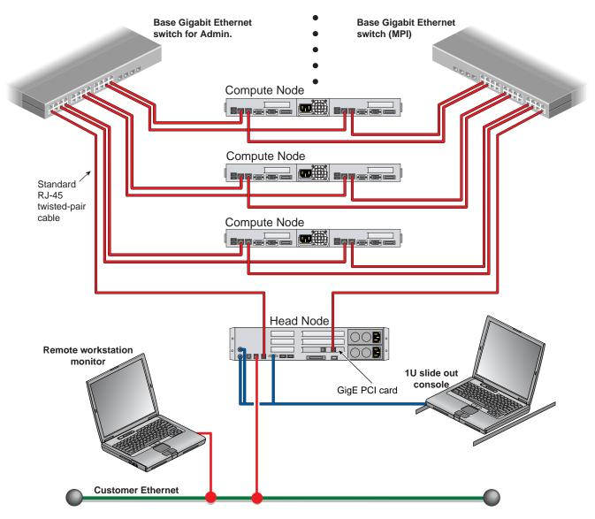
Figure 1-4 Dual-Ethernet Switch Based Cluster Example
