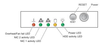
Figure 1-2 SGI Altix XE310 Compute Node Controls and Indicators
