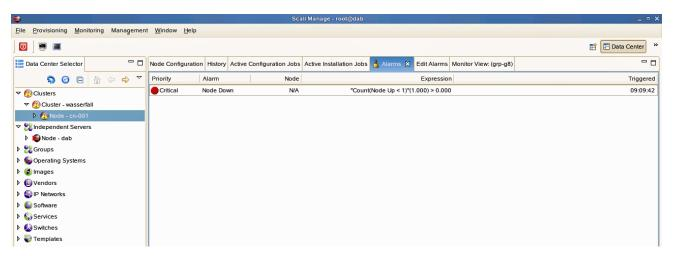
Figure 2-20 Node Down Alarm Screen Example
