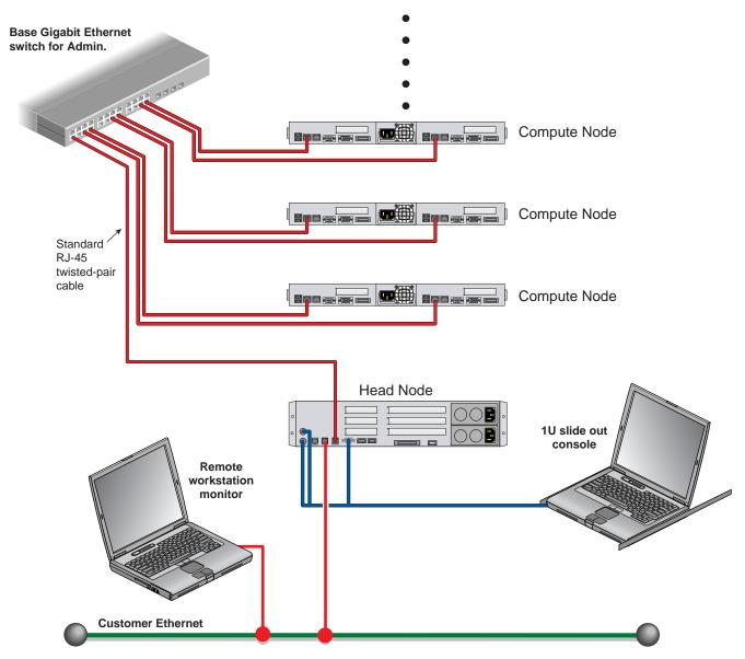
**Figure 1-3** Basic Cluster Configuration Example Using a Single Ethernet Switch
