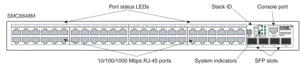
Figure 1-7 SMC Switch Connectors Example
