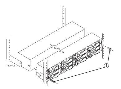
Figure 1-22 Securing the Front Screws on the Disk Enclosure
