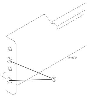
Figure 1-20 Support Rail Alignment Spacers Example
