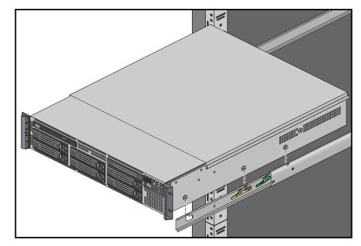
3. Using two people, align and insert the data manager's mounting studs into the component mounting channels on the two slide rails, see Figure 1-16 for an example.
