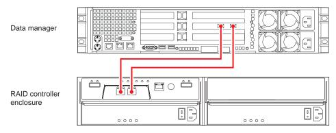
Figure 1-11 One Data Manager One Controller Enclosure (Single SATA RAID Controller)
