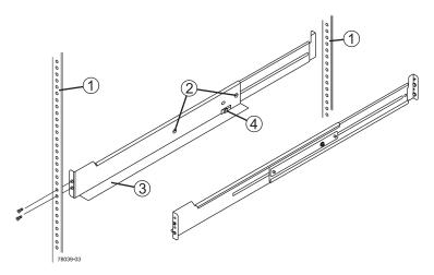
Figure 1-19 Support Rail Attachment to Rack Example
