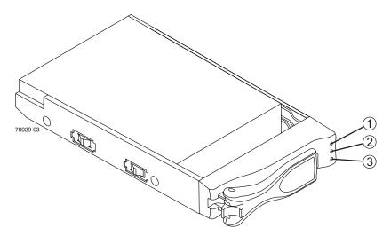
Figure 1-10 Disk Drive Indicator LEDs
