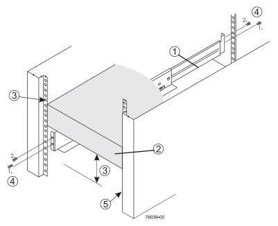
Figure 1-18 Rail Mounting Overview Example
