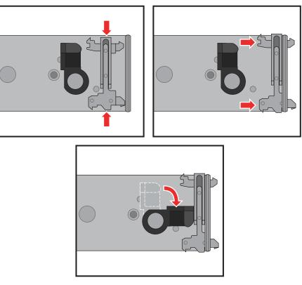
Figure 1-15 Reversing the Rail Pin Adapter
