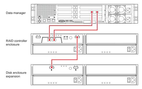
Figure 1-12 Data Manager, Single-Controller RAID Enclosure and One Disk Expansion
