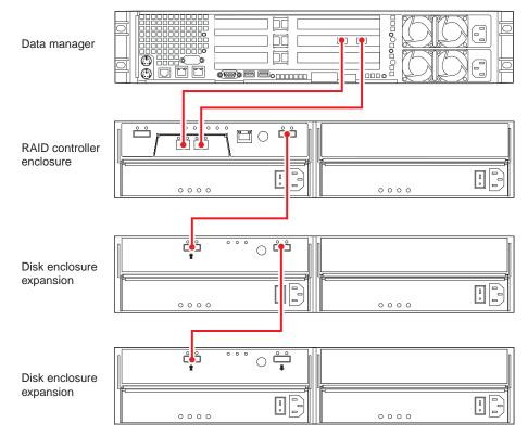
Figure 1-13 Data Manager, Single-Controller RAID Enclosure and Two Disk Expansion Units
