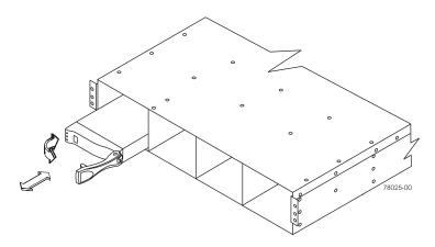
Figure 1-9 Drive Extraction (Front) From the Enclosure
