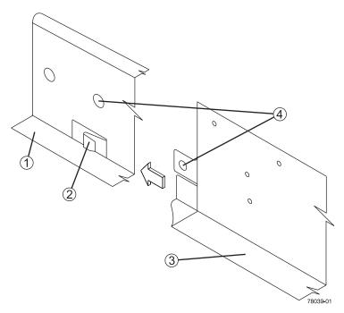
Figure 1-21 Sliding the RAID/Disk Enclosure into the Rail's Rear Clip
