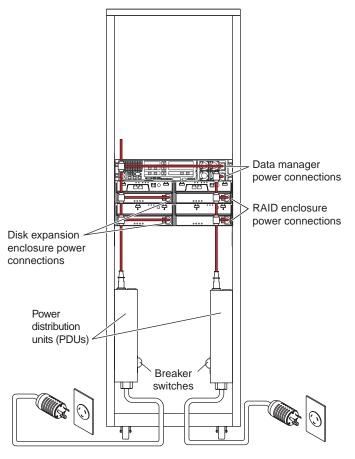
Figure 1-4 Connection Example of a Racked System to Power
