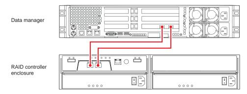
Figure 1-12 One Data Manager One Controller Enclosure (Single SATA RAID Controller)
