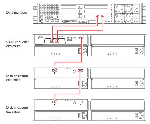
Figure 1-14 Data Manager, Single-Controller RAID Enclosure and Two Disk Expansion Units
