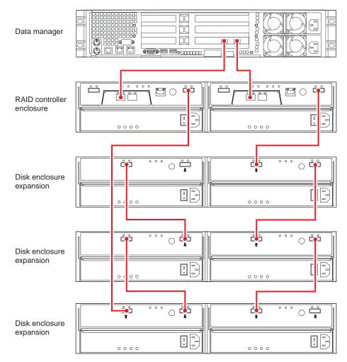
Figure 1-17 Data Manager, Dual-Controller RAID Enclosure and Three Disk Expansion Units
