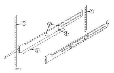
Figure 1-22 Support Rail Attachment to Rack Example
