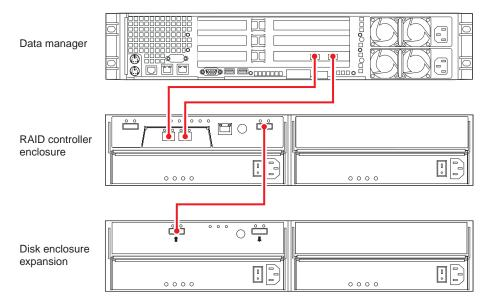
Figure 1-13 Data Manager, Single-Controller RAID Enclosure and One Disk Expansion
