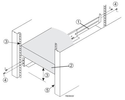
Figure 1-21 Rail Mounting Overview Example
