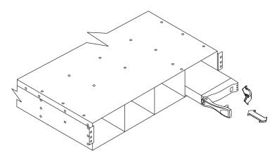
Figure 1-10 Drive Extraction (Front) From the Enclosure
