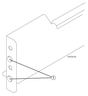
Figure 1-23 Support Rail Alignment Spacers Example
