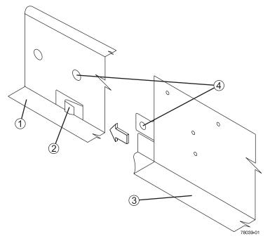
Figure 1-24 Sliding the RAID/Disk Enclosure into the Rail's Rear Clip
