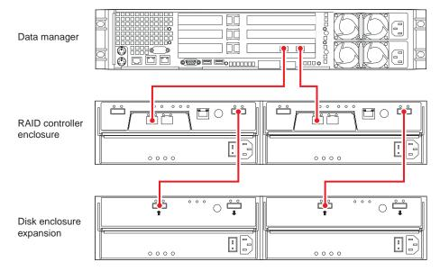
Figure 1-16 Data Manager, Dual-Controller RAID Enclosure and One Disk Expansion Unit
