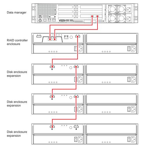
Figure 1-15 Data Manager, Single-Controller RAID Enclosure and Three Disk Expansion Units
