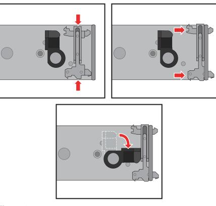
Figure 1-18 Reversing the Rail Pin Adapter
