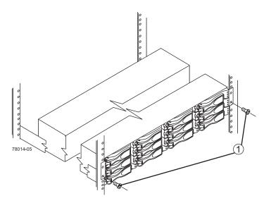
Figure 1-25 Securing the Front Screws on the Disk Enclosure
