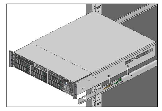
3. Using two people, align and insert the data manager's mounting studs into the component mounting channels on the two slide rails, see Figure 1-19 for an example.
