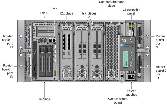
Figure 1-2 InfiniteStorage NEXIS 5000 Compute Appliance Connectors Example
