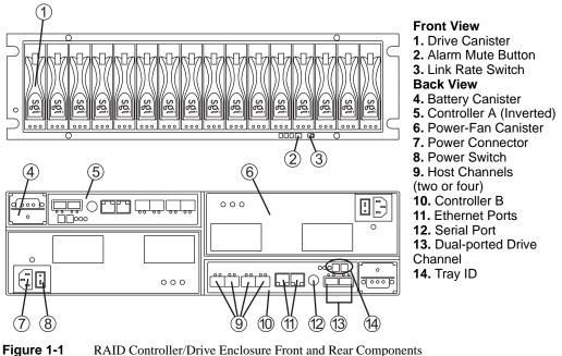
RAID Controller/Drive Enclosure Front and Rear Components
