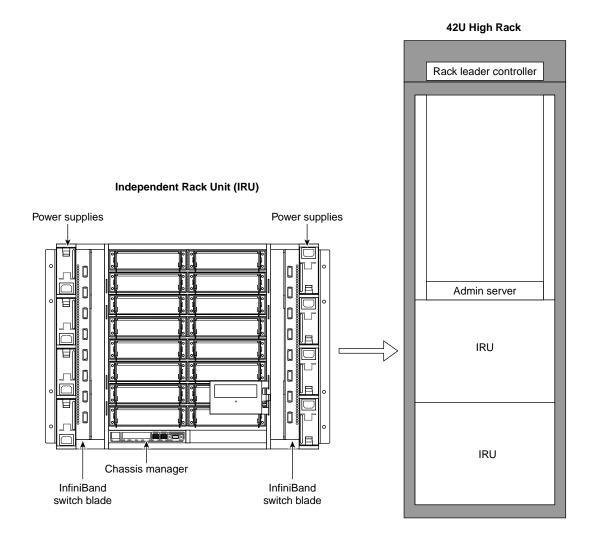
Figure 1-1 Basic System Building Blocks
