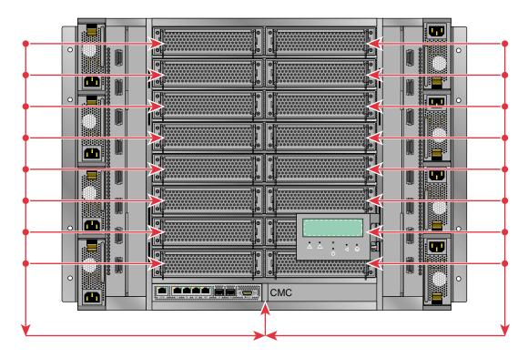
Figure 1-6  $\ensuremath{\texttt{VLAN\_GBE}}$  and  $\ensuremath{\texttt{VLAN\_BMC}}$  Network Connections - IRU View
