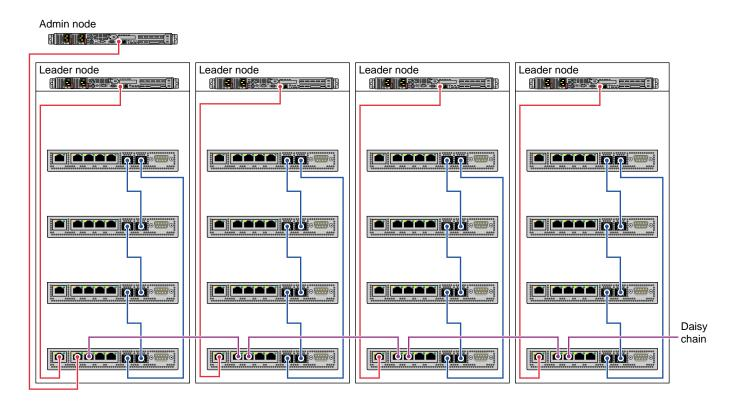
Figure 1-2 Chassis Manager Cabling
