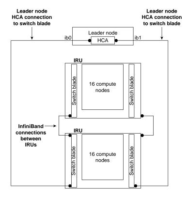
Figure A-1 Two InfiniBand Fabrics in a System with Two IRUs
