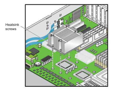
Figure 3-7 Install a CPU Heatsink
