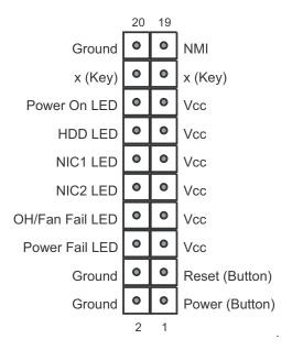
Figure 3-4 Control Panel Connector JF1 Pins
