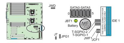
Figure 3-30 Compact Flash Jumper Settings (JWF1)
