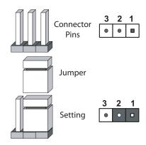
Figure 3-25 Explanation of Jumper Pins
