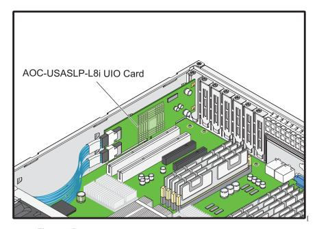
Figure 1-5 L8i UIO RAID Controller
