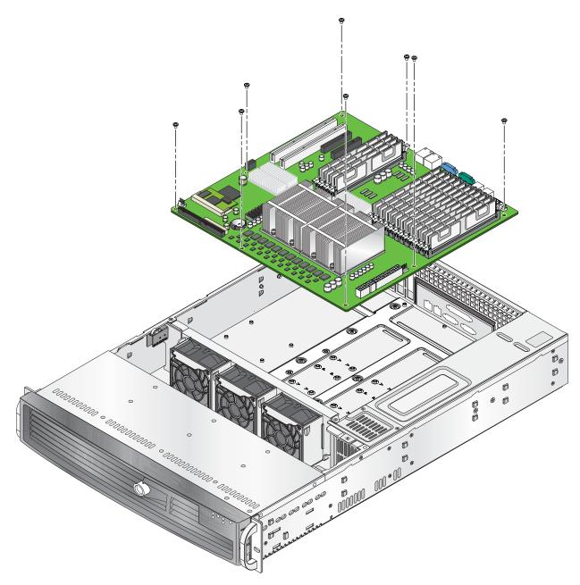
Figure 3-2 Node Board Replacement
