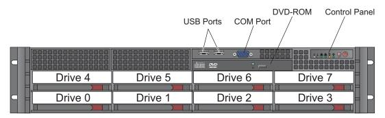
Figure 4-1 Chassis Front View
