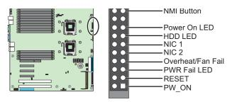
Figure 3-15 JF1 Connector Location Pin Definitions
