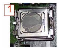
**Note:** If you plan to re-use the heatsink with a replacement processor, you must clean the TIM off of the heatsink. (Refer to "Removing TIM from a Heatsink" on page 45.)
