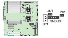
Figure 3-28 3rd Power Failure Detect Jumper Locations (JP3)
