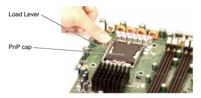
2. Gently lift the load lever to open the load plate.
