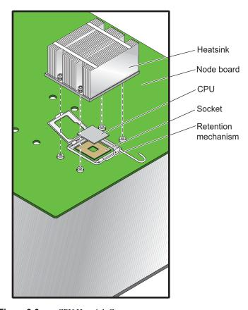
Figure 3-6 CPU Heatsink Components
