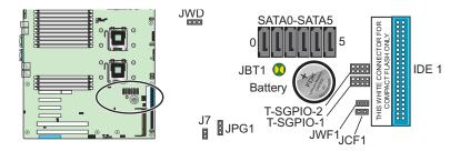
Figure 3-19 SGPIO Connector Location
