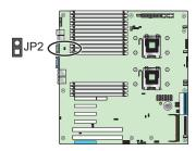
Figure 3-33 Memory Voltage Select Jumper Settings (JP2)
