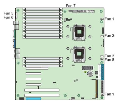
Figure 3-16 Fan Connector Locations
