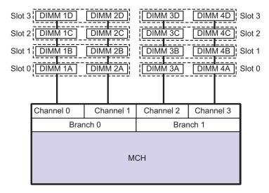
Figure 3-9 Memory Block Diagram
