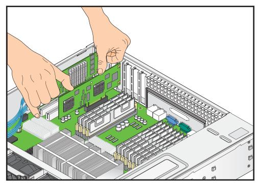
Figure 3-13 Install a PCI Card
