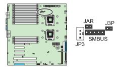
Figure 3-21 SMBUS Connector Location
