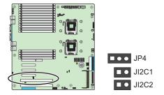
Figure 3-31 JI2C1 and JI2C2 Jumper Settings (JI2C1/JI2C2)
