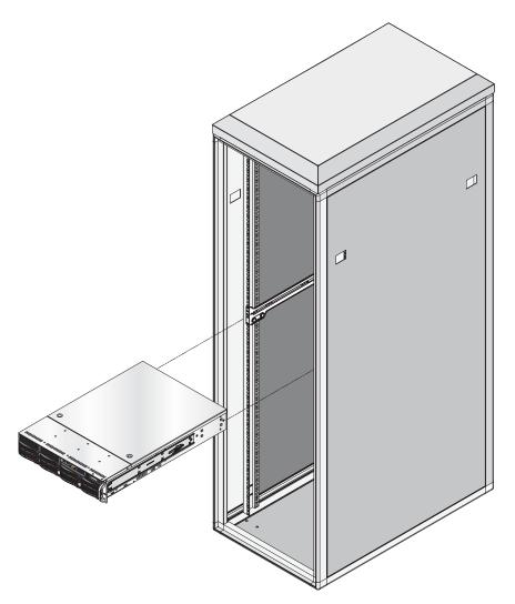
Figure 2-3 Install the Server in a Rack
