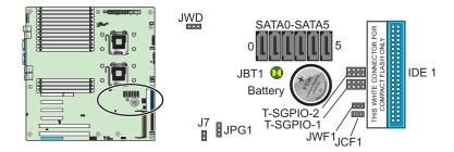
Figure 3-26 CMOS Memory Jumper Location (JBT1)
