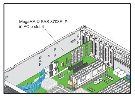
Figure 1-6 LSI MegaRAID 8708ELP RAID Controller
