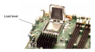
9. If the CPU is properly installed into the socket, the PnP cap is automatically released from the load plate when the lever locks.
