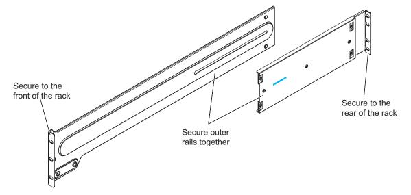
Figure 2-1 Rack Rail Installation
