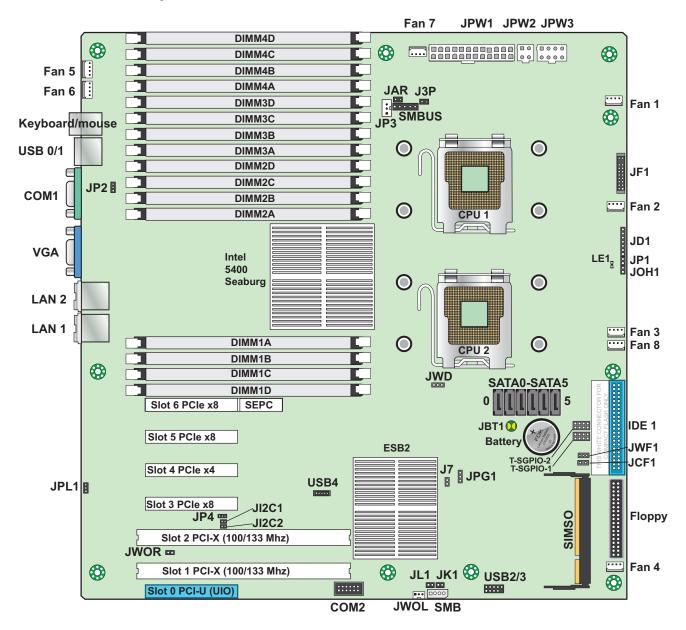
Figure 3-12 Node Board Component Locations
