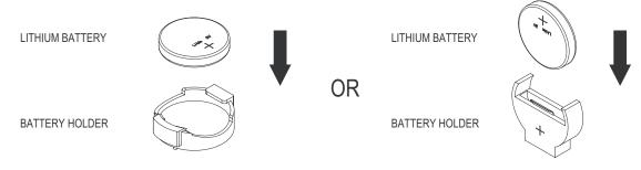
Figure E-1 Install the Battery
