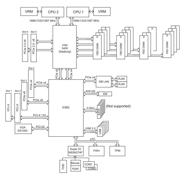
Figure 1-4 Node Board Block Diagram
