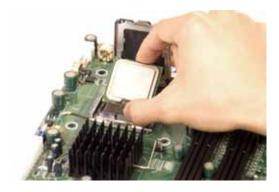
4. Align pin 1 of the CPU (the corner marked with a triangle) with the notched corner of the CPU socket.
