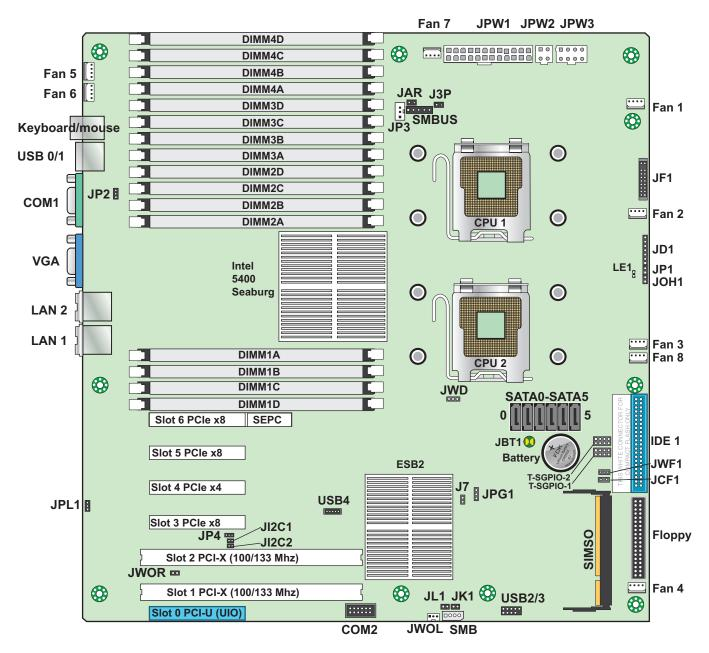
Figure 3-3 Node Board Components
