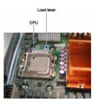
2. Gently lift the load lever to open the load plate.
