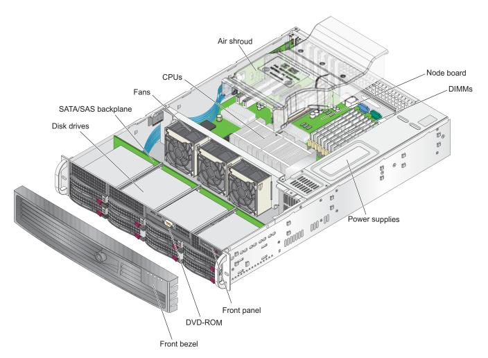
Figure 1-2 Chassis Components
