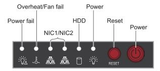
Figure 1-8 Front Panel Controls and Indicators
