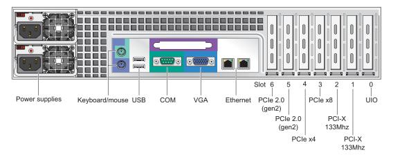
Figure 4-2 Chassis Rear View
