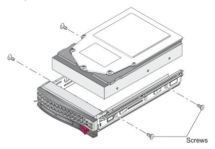
Figure 4-6 Disk Drive Carrier
