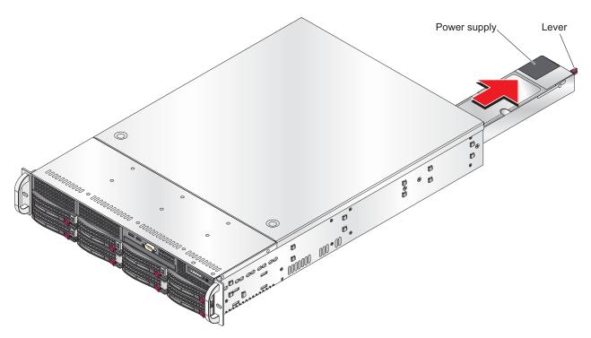
Figure 4-12 Power Supply Replacement
