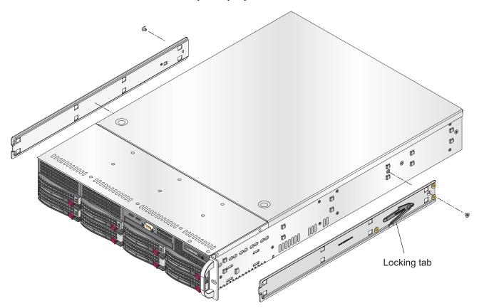
Figure 2-2 Chassis Rail Installation
