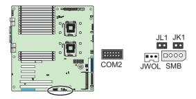
Figure 3-17 Chassis Intrusion Connector Location
