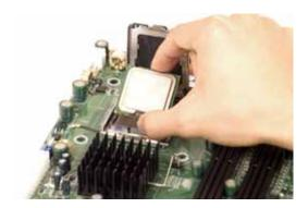
**Note:** If you are removing the processor so that you can return the node board to SGI, install a PnP cap in the socket.
