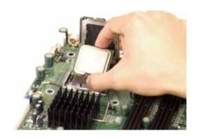
**Note:** If you are removing the processor so that you can return the node board to SGI, install a PnP cap in the socket.
