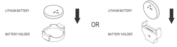
Figure E-1 Install the Battery
