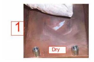
3. Use a different lint-free cloth moistened with isopropyl alcohol (IPA) to remove any remaining TIM from the heatsink.
