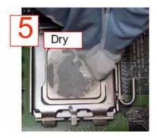
5. Use a different lint-free cloth moistened with isopropyl alcohol (IPA) to remove any remaining TIM from the processor.
