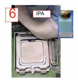
**Note:** Be sure to remove TIM from the gaps between the processor and the load plate.
