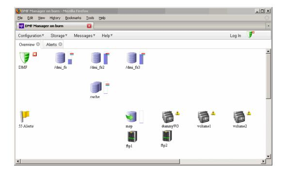
Figure 3-5 DMF Manager Showing Problems in the DMF System
