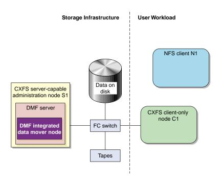
Figure 1-3 Basic DMF in a CXFS Environment
