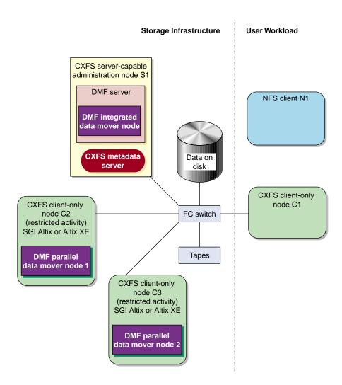
Figure 1-4 DMF with the Parallel Data Mover Option in a CXFS Environment
