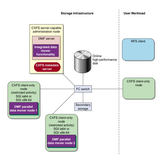
Figure 1-8 DMF with the Parallel Data Mover Option in a CXFS Environment
