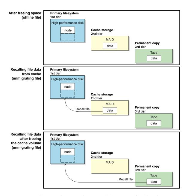
Figure 1-6 Three Tiers with Fast-Mount Cache: Freeing and Recalling File Data
