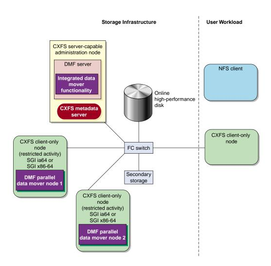
Figure 1-10 DMF with the Parallel Data Mover Option in a CXFS Environment
