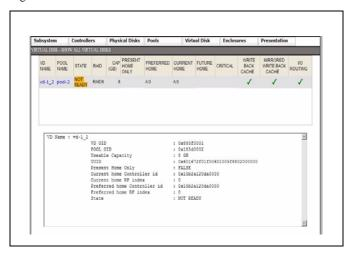
**NOTE:** A virtual disk on a storage pool is NOT accessible until its initialization is complete.
