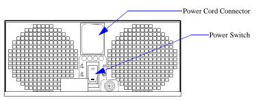
The InfiniteStorage 6120 must always be operated with two PCM installed. Module replacement should only take a few minutes to perform but must be completed with 10 minutes from removal of the failed module. Four (4) LEDs mounted on the PCM indicate the status of the module and the fans (Figure 6). Figure 7 provides a description of the color and status of the LEDs.
