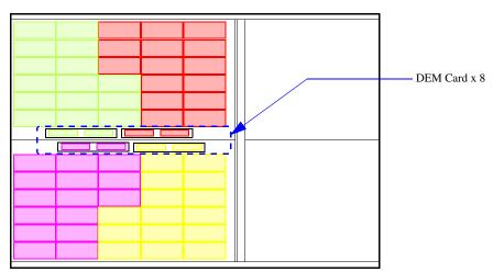
Figure 9. DEM Card Locations (Viewing from Top)
