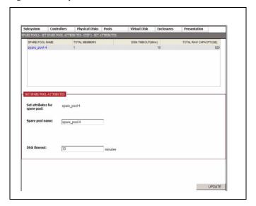
**WARNING:** When assigning disk drives to a spare pool that is to be assigned to a given storage pool, be sure to select a disk that is as large or larger than any disks in the assigned storage pool.
