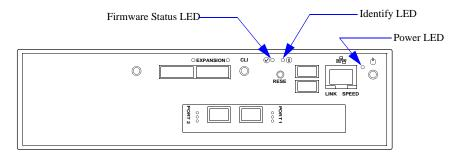
Figure 91. Controller LED Indicators
