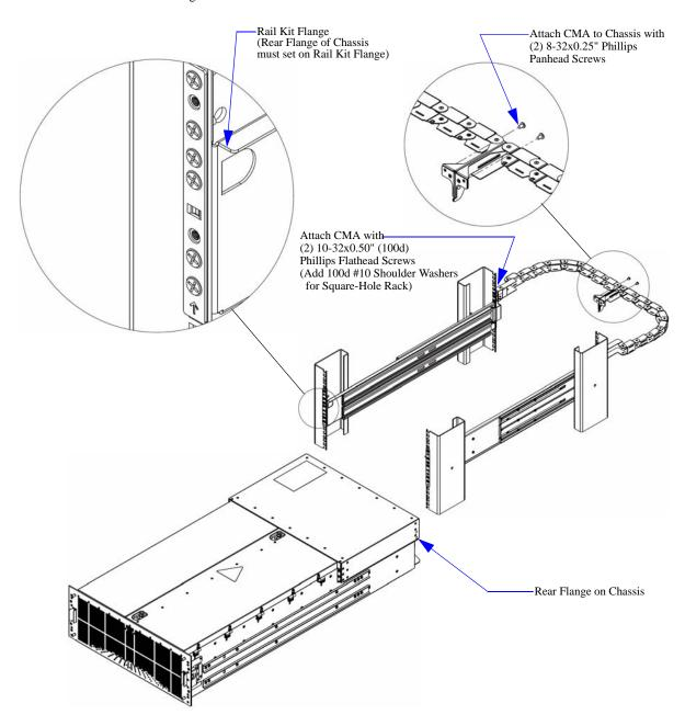
Figure 17. Install Chassis to Rack
