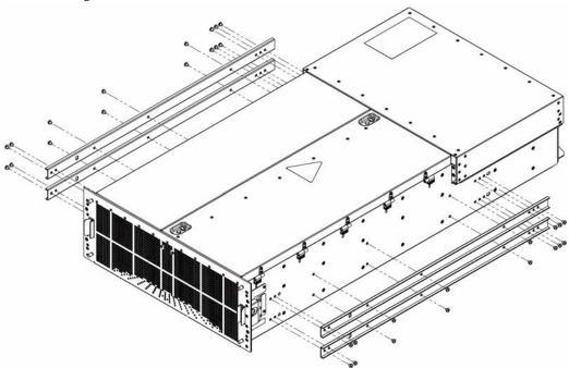
Figure 14. Attach 4 Inner Sliders to Chassis
