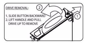
**CAUTION:** Drive spin down—Damage can occur to a drive if it is removed while still spinning. If possible, use the operating system to spin down the drives prior to removal. If this is not possible, we recommend that you perform ALL steps of the following procedure to ensure that the drive has stopped prior to removal.
