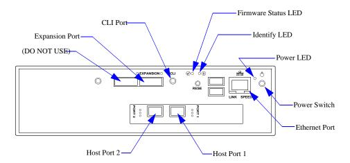
There are two 8Gb/s host ports for Fibre Channel host connections. You may connect your host systems directly to these ports or connect the ports to your Fibre Channel switches and hubs. When an FC signal is present on the port, the respective LED turns green.
