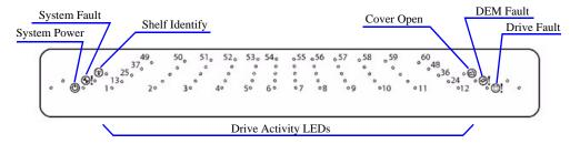
Figure 12. Front Panel LED Description
