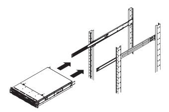
Figure 2-5 Installing the Server in a Rack
