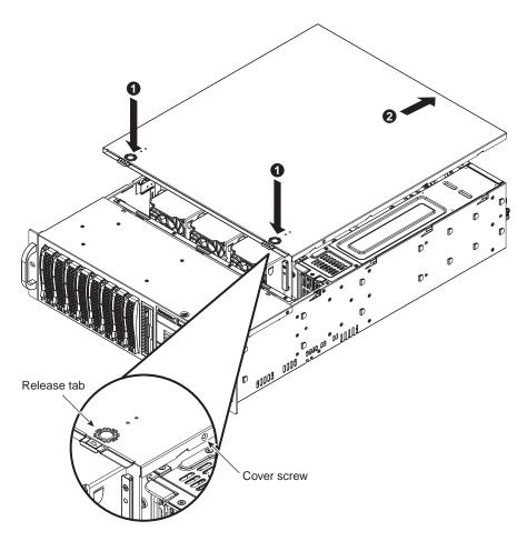
Figure 5-1 Removing the Chassis Cover
