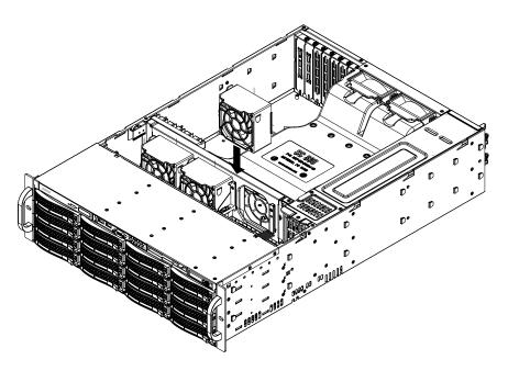
Figure 5-7 Installing the Front Fan
