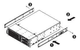
Figure 2-4 Installing the Inner Rail Extensions
