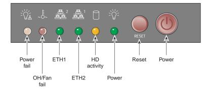
Figure 4-1 Control Panel Interface
