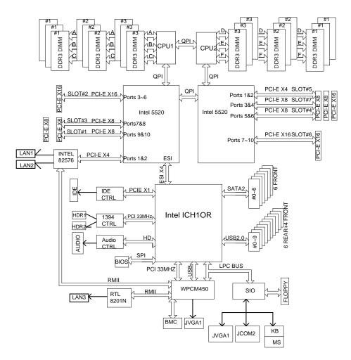
Figure 1-2 Altix XE500 Serverboard Block Diagram
