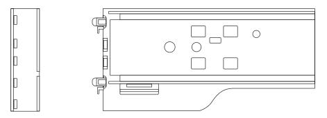
Figure 2-2 Square-to-round Hole Adapter for 2U Quick Attach Rails
