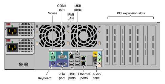
Figure 5-5 PCI Slot Location
