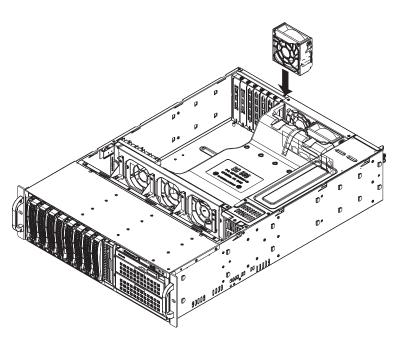
Figure 5-8 Installing a Rear Fan
