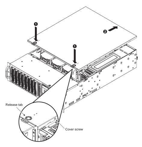
Figure 2-6 Accessing the Inside of the System
