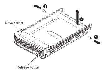
**Figure 5-3** Removing the Dummy Drive from the Carrier
