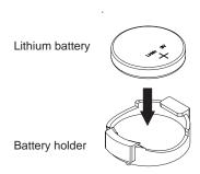
Figure 3-1 Installing the Onboard Battery
