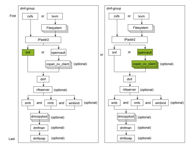
Figure 6-4 Adding the Resource for the Mounting Service
