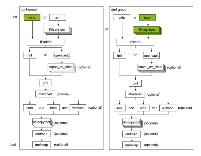
Figure 6-2 Adding the Resources for the DMF Group and the Clustered/Local Filesystems
