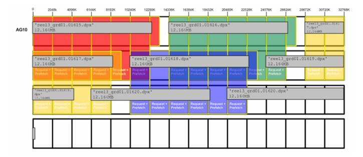
be prefetched into cache. Figure 12-8 shows an example of a 4-thread frametest read (2-MB stripe unit / 1-GB cache size/ prefetch = x1 / 16 slices).
