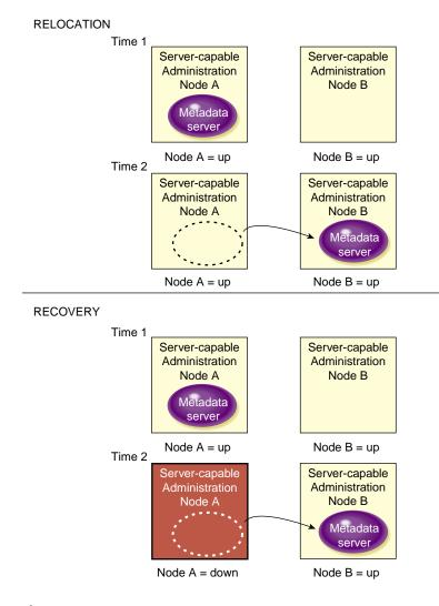
Figure 1-6 Relocation versus Recovery
