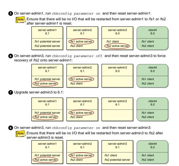
Figure 12-3 Example Rolling Upgrade Procedure (part 2)
