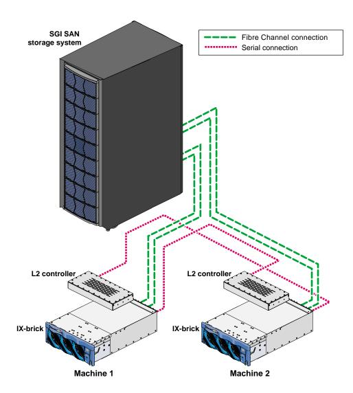
Figure C-6 Altix 3000 Connections
