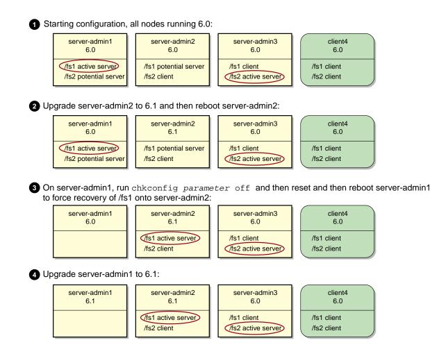
Figure 12-2 Example Rolling Upgrade Procedure (part 1)
