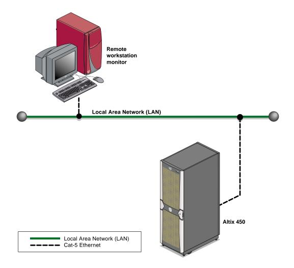
Figure C-2 SGI Altix 450 System Control Network
