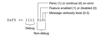
Figure D-1 Explanation of Bit Values
