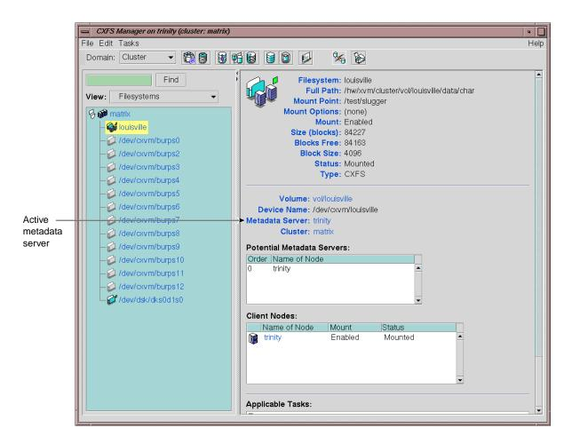
Figure 12-5 GUI Window Showing the Metadata Server
