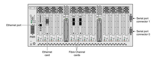
Figure C-5 IX-brick Rear Panel
