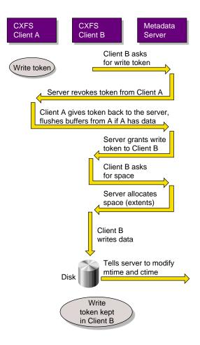
Figure A-6 Metadata Flow on a Write
