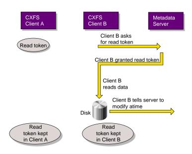
Figure A-8 Metadata Flow on a Read on Client B Following a Read on Client A
