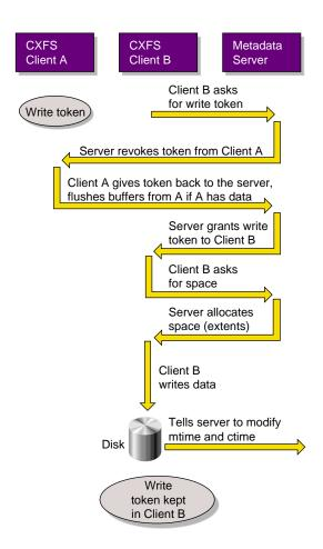
Figure A-6 Metadata Flow on a Write
