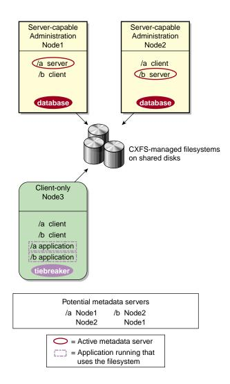
Figure 1-4 Two Metadata Servers for Two Filesystems
