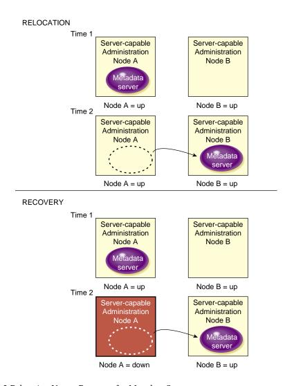
Figure 1-6 Relocation Versus Recovery for Metadata Servers
