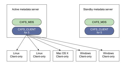
Figure 5-2 Adding a Fifth Client-only Node and Changing the OS Composition
