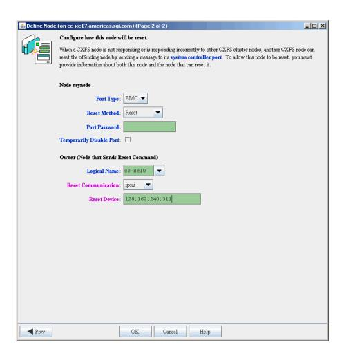
Figure 10-4 Example System Reset Settings
