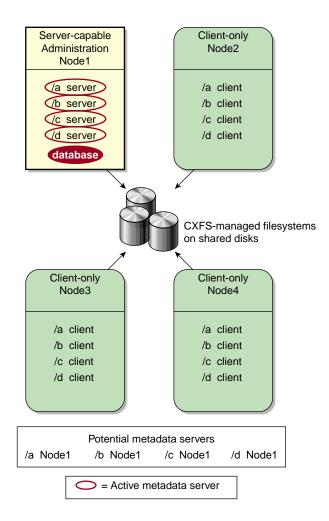
Figure 1-3 One Metadata Server (No Relocation or Recovery)
