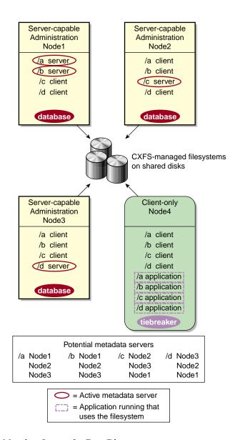
Figure 1-5 Three Metadata Servers for Four Filesystems
