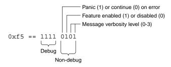
Figure D-1 Explanation of Bit Values
