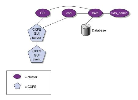
Figure A-4 Communication for a Server-Capable Administration Node Not in a Cluster
