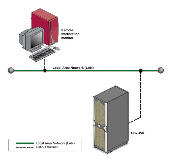
Figure E-2 SGI Altix 450 System Control Network
