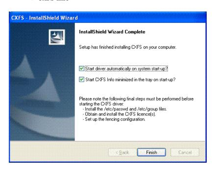
Figure 5-11 Start Driver for the cxfs\_client Service
