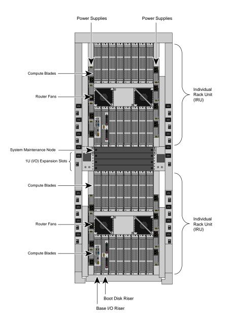
Figure 2-1 SGI Altix UV 1000 System Rack
