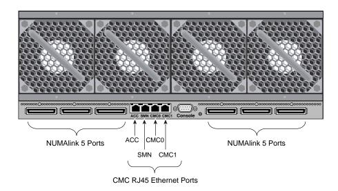
Figure 1-7 CMC Ethernet Ports on SGI Altix UV 100 Systems
